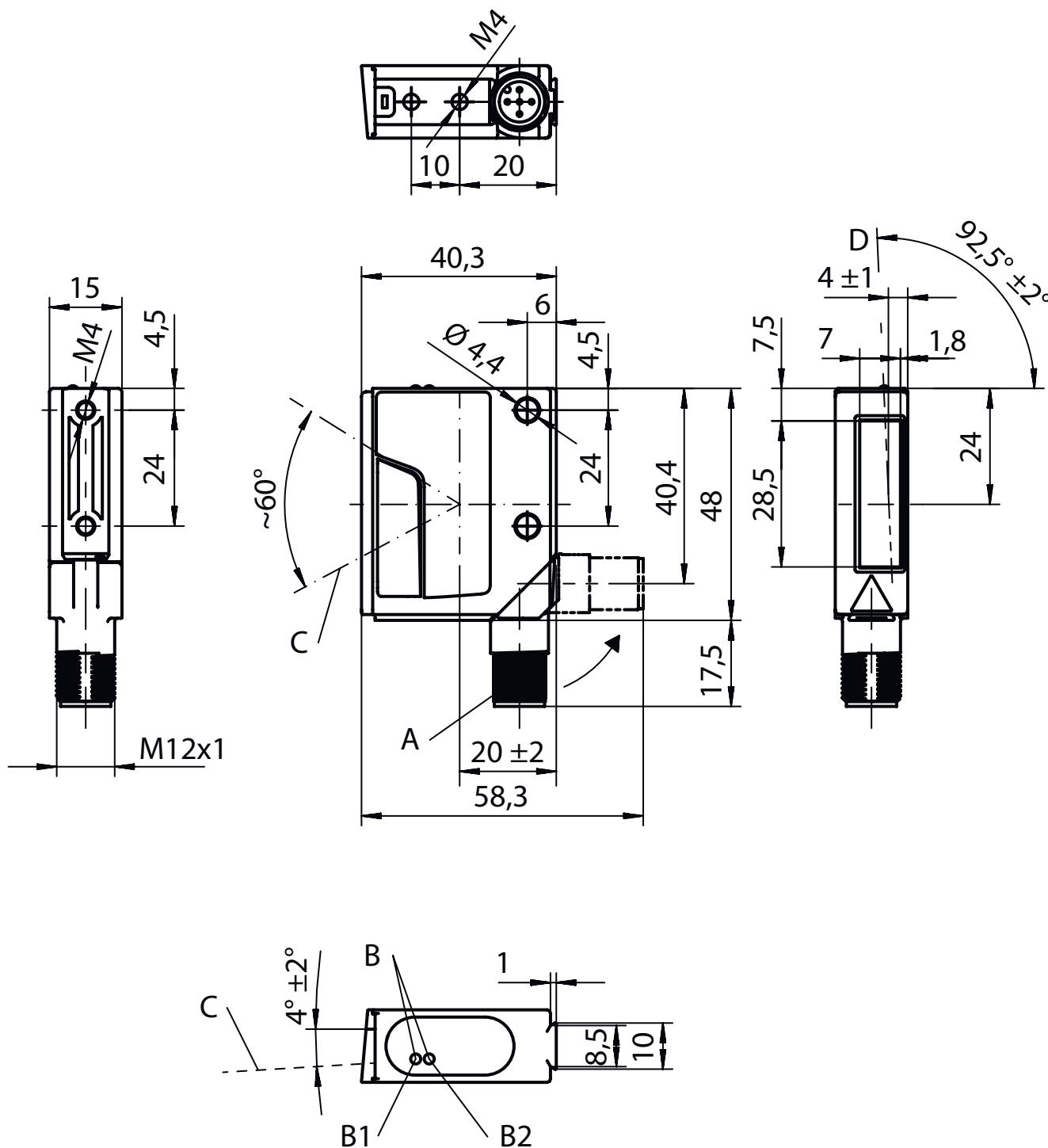
A Turning connector, turnable by 90°
