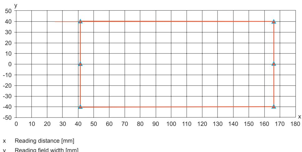
Reading field curve for module m = 0.2 ... 0.5 mm (8 ... 20 mil)
