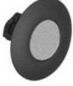
50140183 | MTKZ 7-30 SET | Reflector | Design: Round<br>Reflective surface, diameter: 15 mm<br>Material: Plastic<br>Base material: Plastic<br>Chemical designation of the material: PA<br>Fastening: Clip<br>Suitable for bore hole diameter: 6 ... 7 mm<br>Suitable for material thickness: 0.8 ... 5 mm<br>Processing temperature: 5 ... 45 °C |
