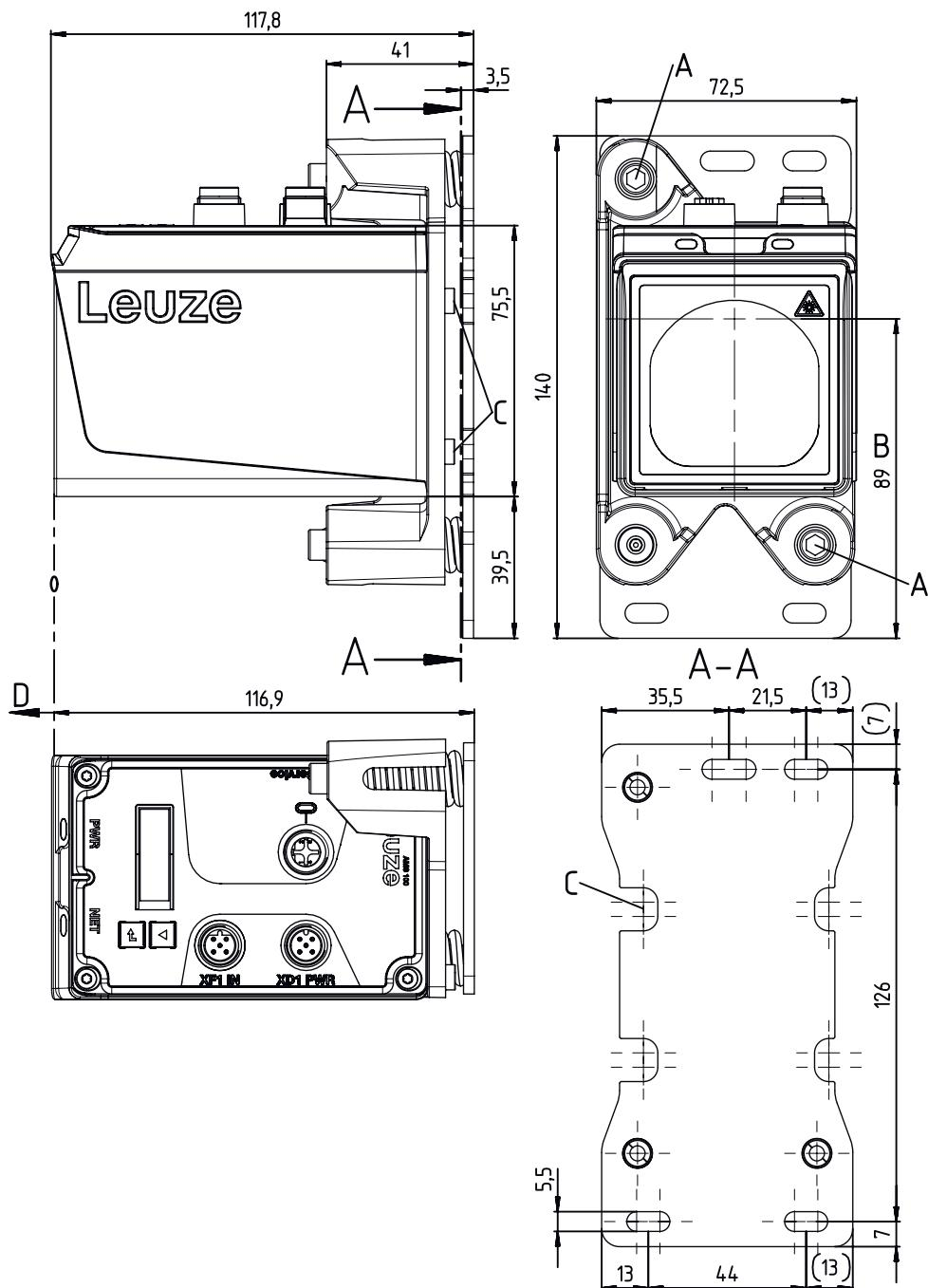
A Adjustment screws with hexagon socket WAF4
