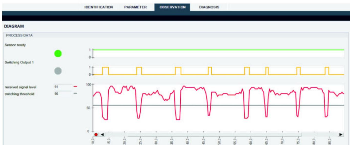
Simple visualization of the process data in the Leuze Sensor Studio PC configuration software enables a fast assessment of the process stability.
