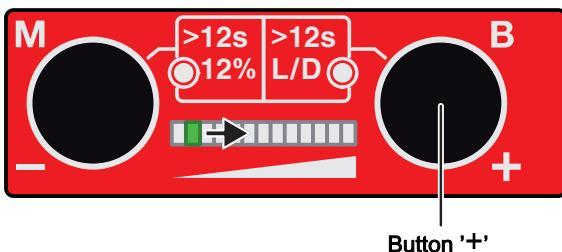
Briefly pressing the '-' button decreases the sensitivity of the sensor, the bar graph indicates less signal.
