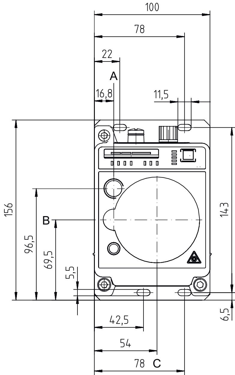
A Center axis of transmitter and alignment laser
