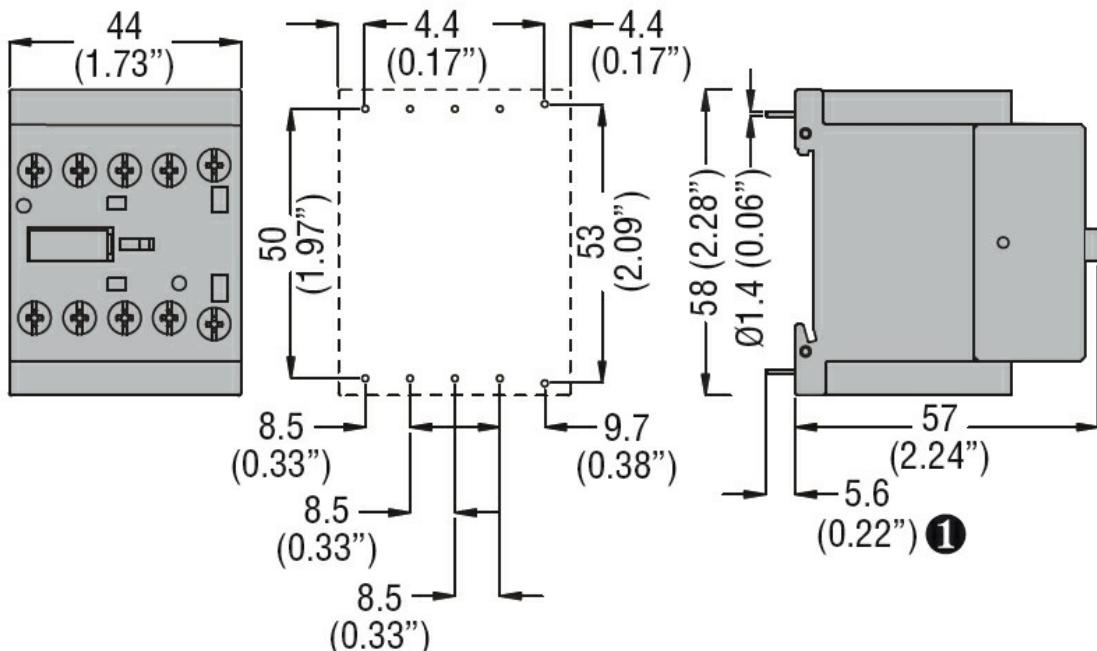
**①** Recommended PCB drillings 1.7-2mm.
