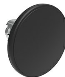
Mushroom head pushbutton, spring return Ø 60mm/2.36" LPSB614
