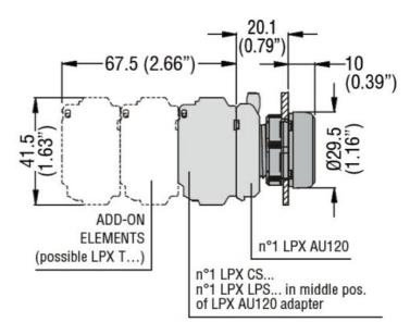
LED INTEGRATED LAMP-HOLDER, FLASHING LIGHT Ø22MM PLATINUM SERIES, SCREW TERMINATION, 18...30VAC/DC. YELLOW
