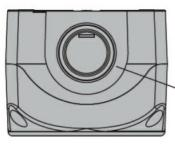
Knockout for M20/M25/PG13.5/PG16 (on top and bottom)
