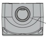
Knockout for M20/M25/PG13.5/PG16 (on top and bottom)
