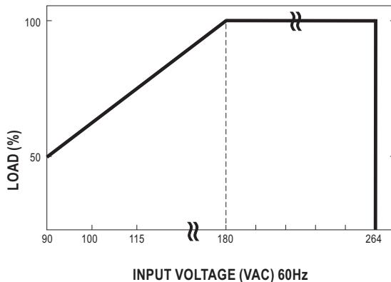
■ DERATING LOADs vs INPUT VOLTAGE
