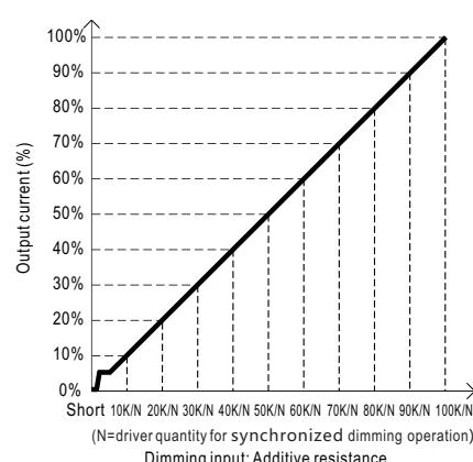
Note : 1. Min. dimming level is about 8% and the output current is not defined when 0% < Iout < 8%.
