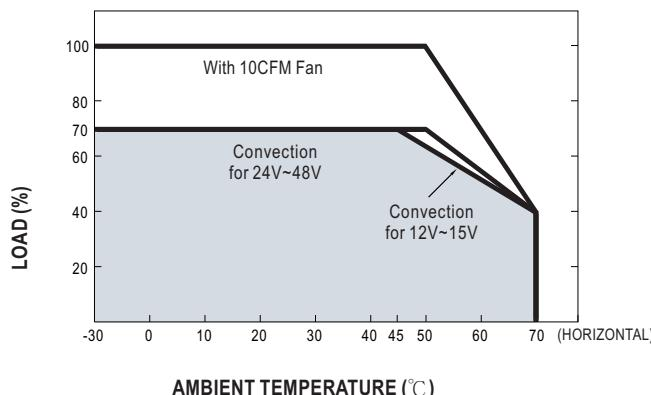
■ Output Derating VS Input Voltage
