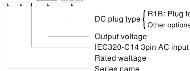
DC plug type R1B: Plug for standard model, power DIN 5 pin
