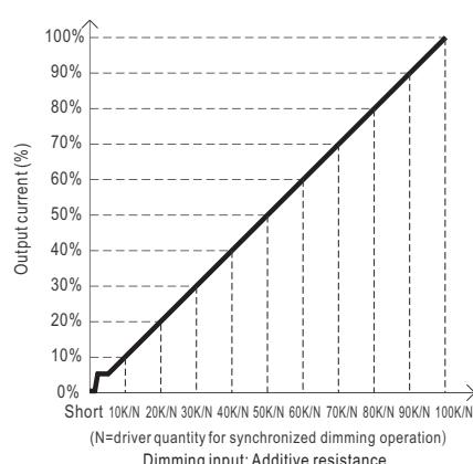
Note : 1. Min. dimming level is about 5% and the output current is not defined when 0% < Iout < 5%.
