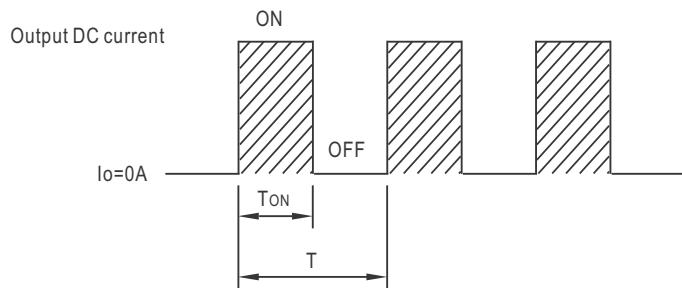
$$\text{Duty cycle}(\%) = \frac{T_{ON}}{T} \times 100\%$$
