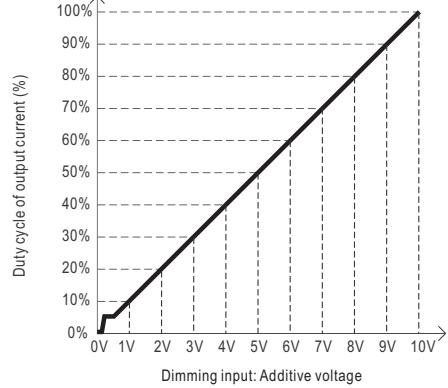
◎ Applying additive 10V PWM signal (frequency range 300~3000Hz):
