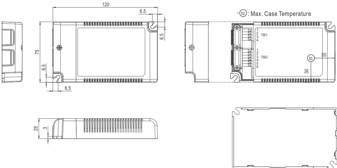
NOTE: Please use wires with a cross section of  $0.75\sim1.5\text{mm}^2$  for TB1
