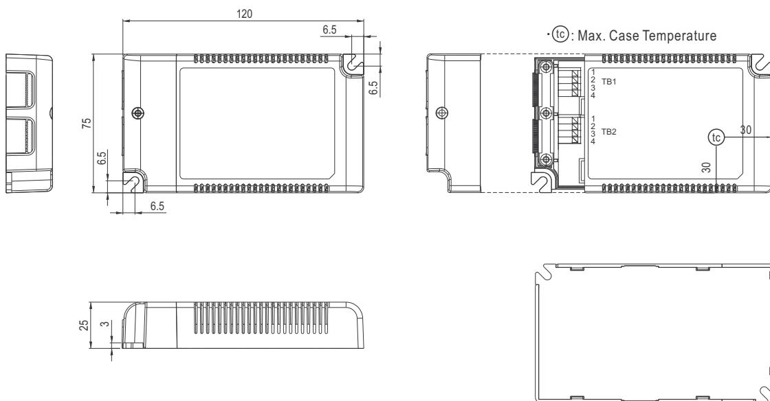
NOTE: Please use wires with a cross section of 0.75~1.5mm<sup>2</sup> for TB1
