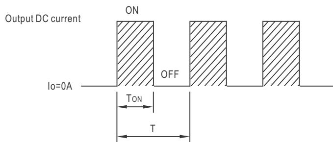
$$\text{Duty cycle}(\%) = \frac{T_{ON}}{T} \times 100\%$$
