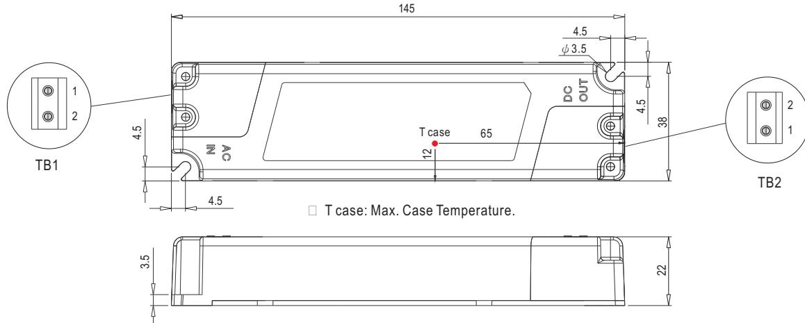
NOTE: The input and output line for using UL1015 18AWG\*2C is suggested
