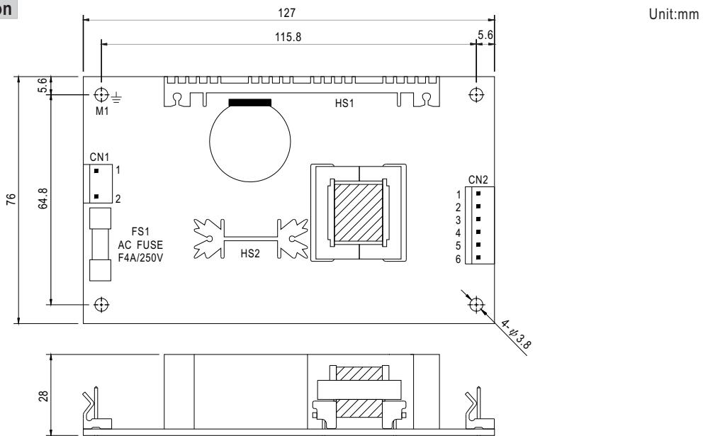
AC Input Connector (CN1) : Molex 5277-02 or equivalent
