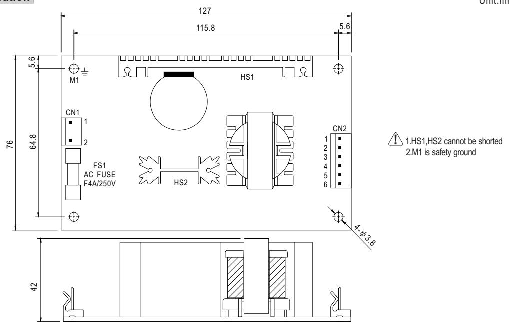
AC Input Connector (CN1) : Molex 5277-02 or equivalent
