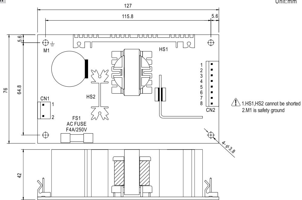
AC Input Connector (CN1) : Molex 5277-02 or equivalent
