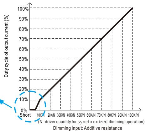
Note : 1. Min. duty cycle of output current is about 6% and the output current is not defined when  $0\% < I_{out} < 6\%$ .
