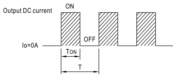
$$\text{Duty cycle}(\%) = \frac{T_{ON}}{T} \times 100\%$$
