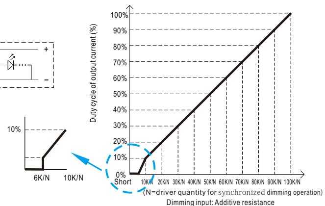
Note : 1. Min. duty cycle of output current is about 6% and the output current is not defined when  $0\% < I_{out} < 6\%$ .
