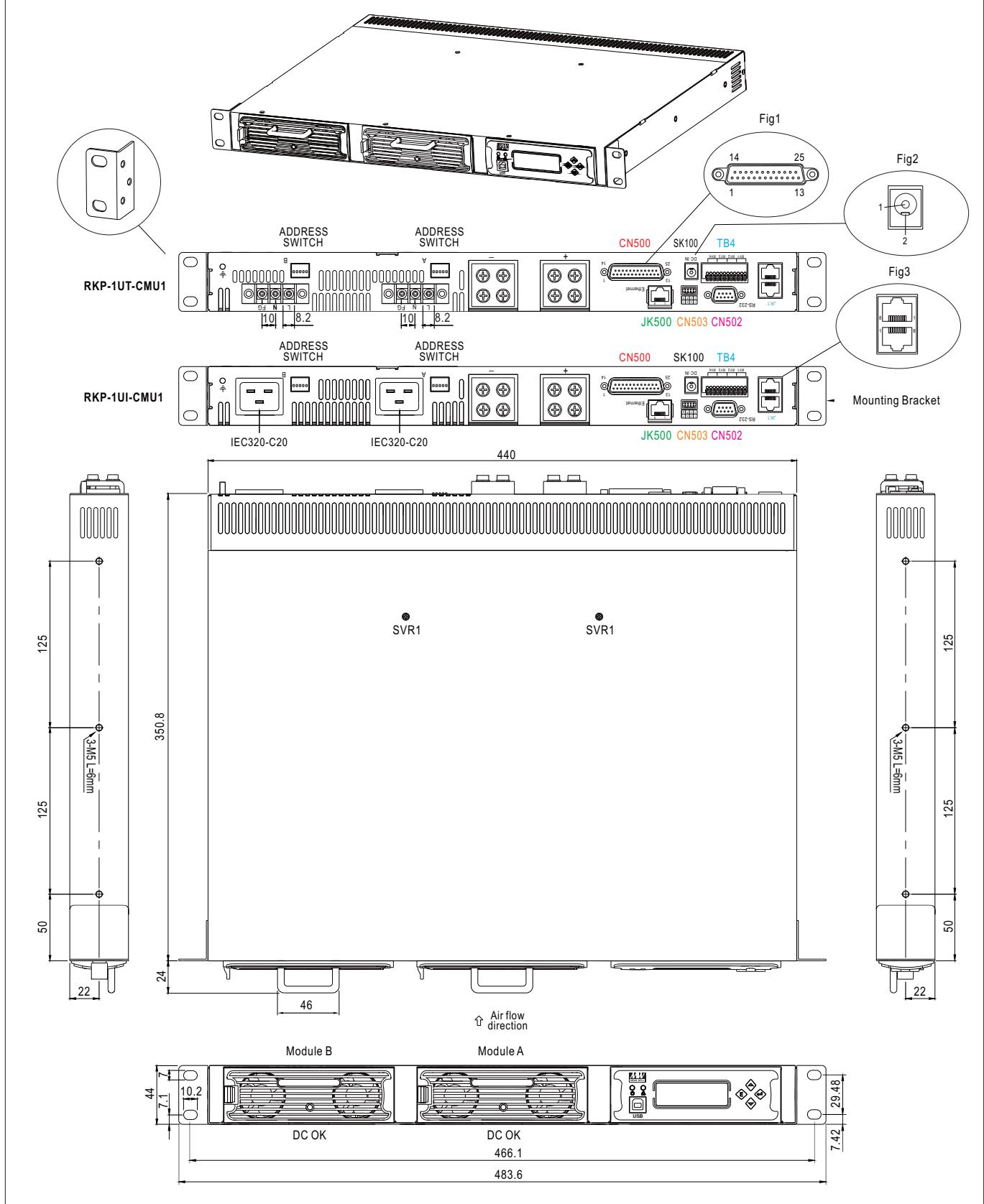
※ IN/OUT Connector Pin No. Assignment([CN500](#)) : D-Type Right Angle 25 positions
