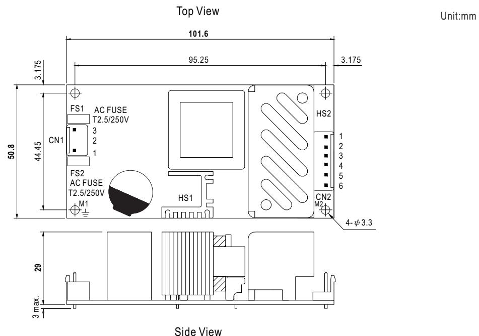
**AC Input Connector (CN1) : JST B3P-VH or equivalent**
