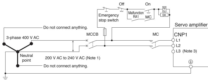
Notes: 1. Use a step-down transformer as necessary to keep the power supply voltage between 200 V AC and 240 V AC.
