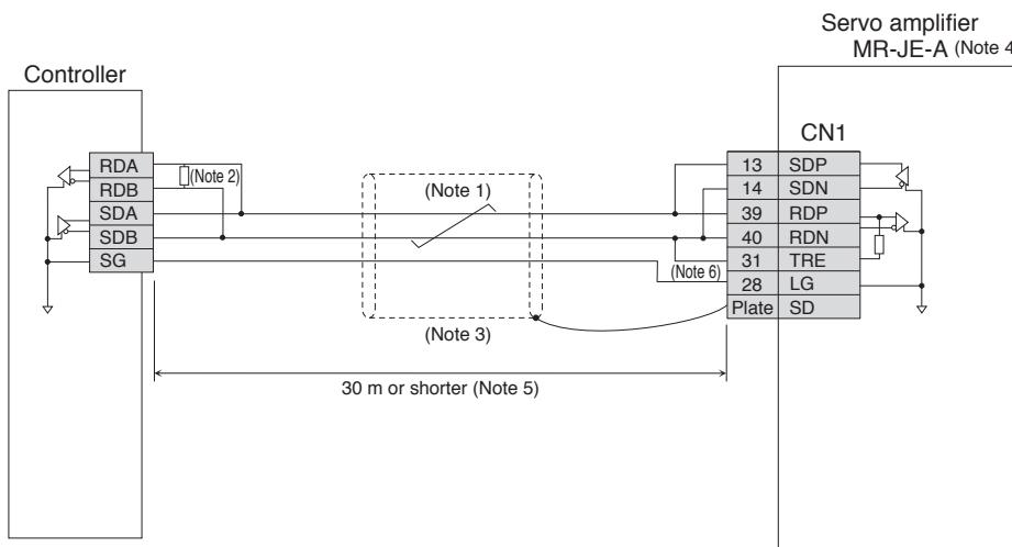
Notes: 1. Twist the wires from SDP and SDN together, and RDP and RDN together.
