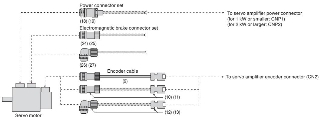
Notes: 1. This cable does not have a long bending life. Thus, be sure to fix the cable before using.
