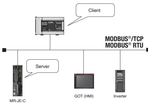
\* MODBUS® RTU is supported by servo amplifiers with software version A4 or later.
