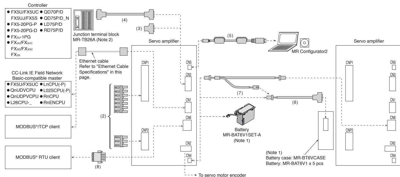
Notes: 1. Refer to "Battery" or "Battery Case and Battery" in this catalog. Battery and battery case are not required when the MR-JE-C servo amplifier is used in incremental system.
