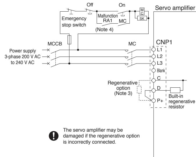
Notes: 1. For 1-phase 200 V AC to 240 V AC, connect the power supply to L1 and L3 terminals. Do not connect anything to L2.
