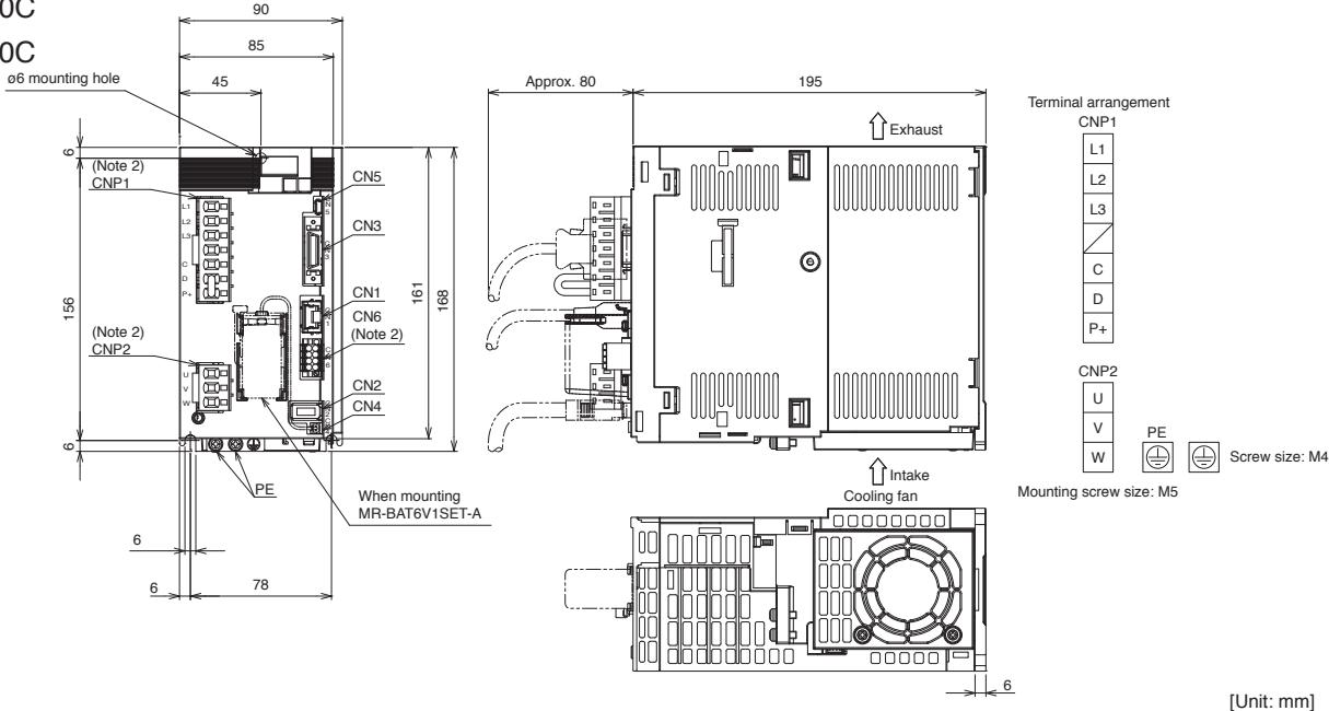
Notes: 1. CNP1 and CN6 connectors are supplied with the servo amplifier.
