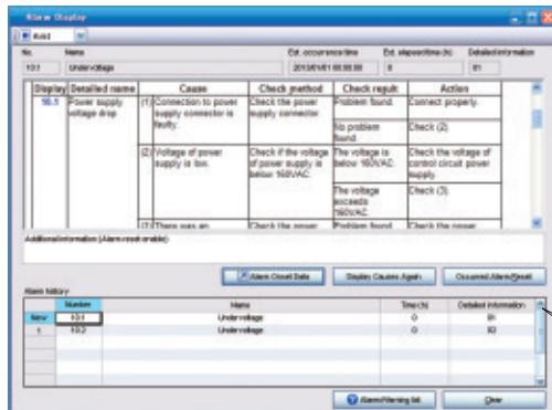
The alarm No. shows whether the undervoltage alarm was caused by instantaneous power failure or by lowered power bus voltage in the servo amplifier.
