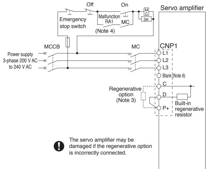
Notes: 1. For 1-phase 200 V AC to 240 V AC, connect the power supply to L1 and L3 terminals. Do not connect anything to L2. The connections are different from MR-E Super series servo amplifiers. Be careful not to make a connection error when replacing MR-E Super with MR-JE.
