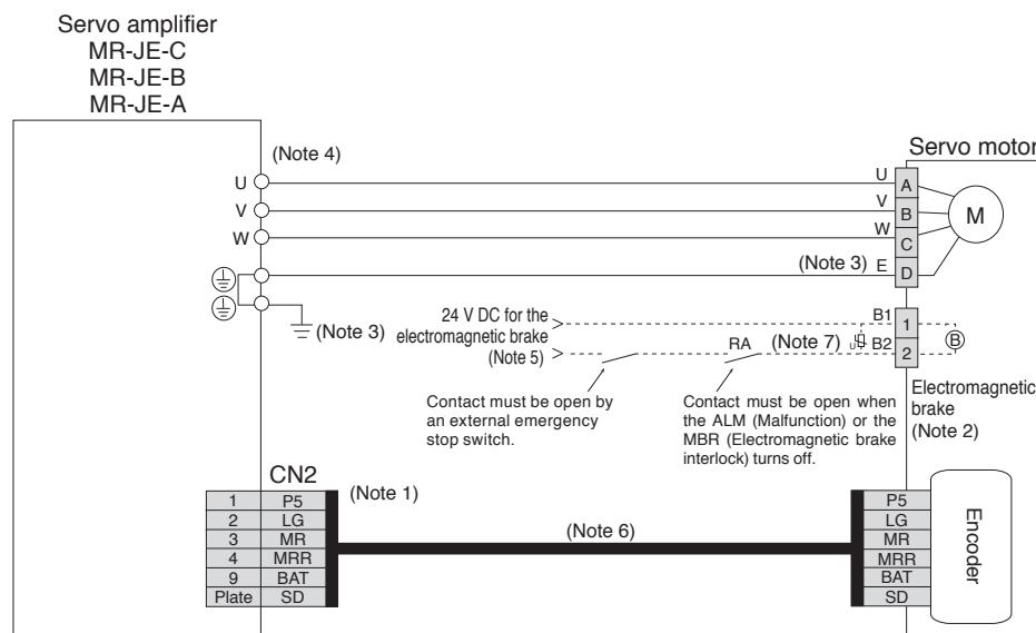
Notes: 1. The signals shown are applicable when two-wire type encoder cable is used. Four-wire type is also compatible.
