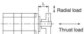
L: Distance between the flange mounting surface and the center of load
