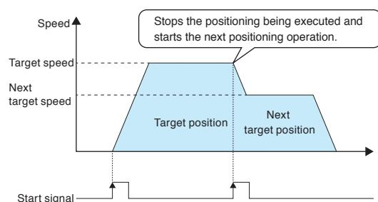
Equipped with positioning function
