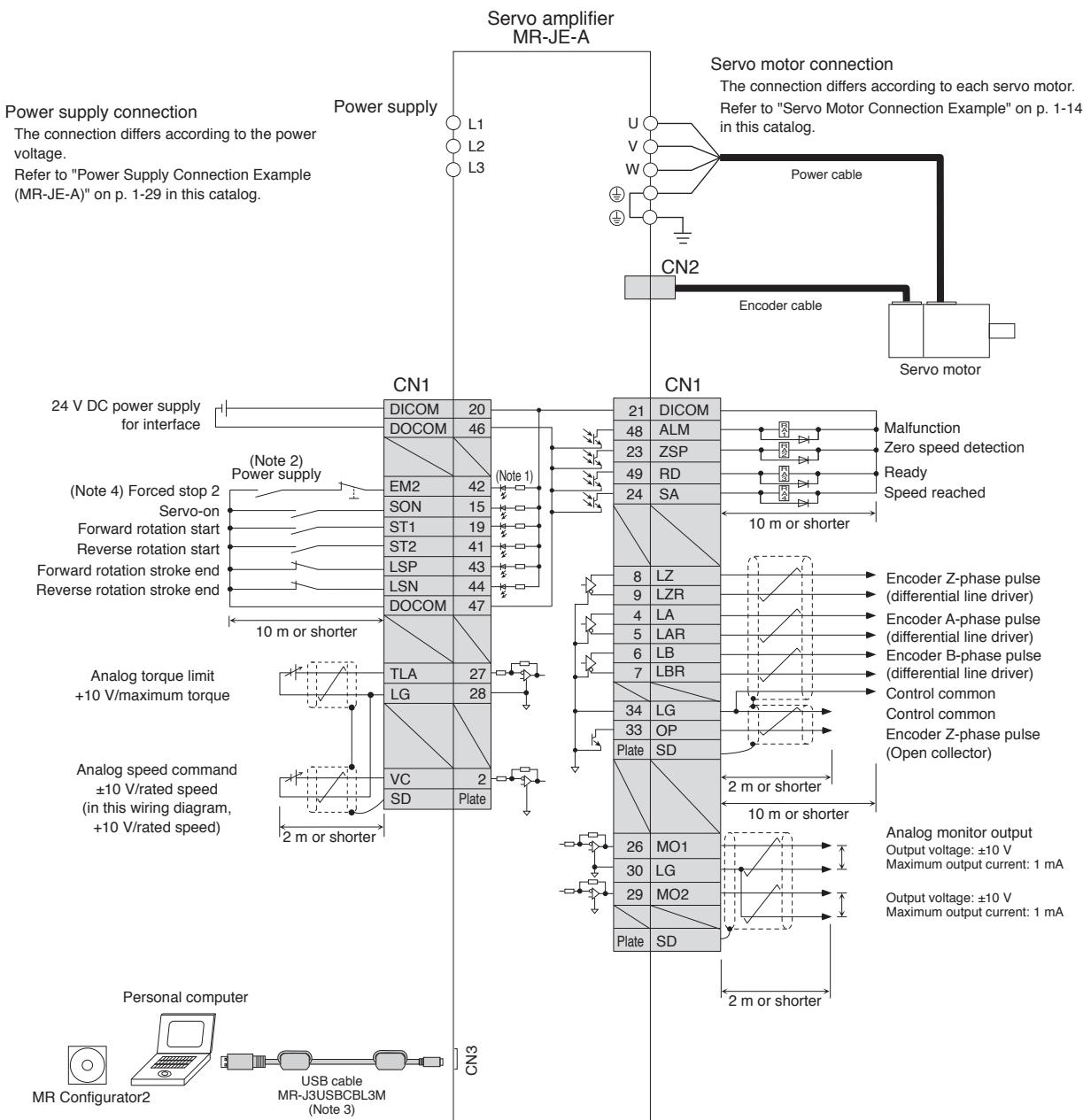
Notes: 1. This is for sink wiring. Source wiring is also possible.
