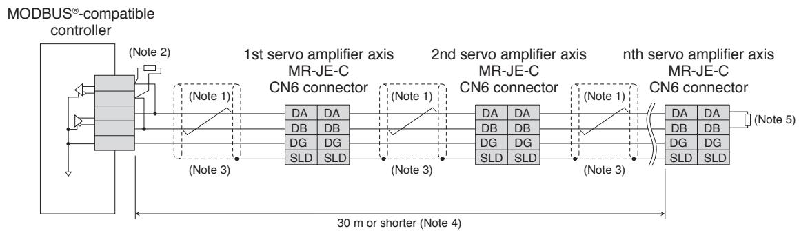
Notes: 1. Twist the wires from DA and DB together.
