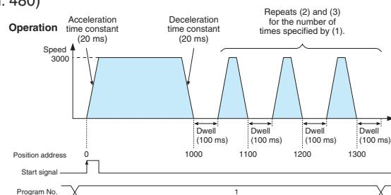
Automatic calculation of travel distance by setting the number of stations in parameter
