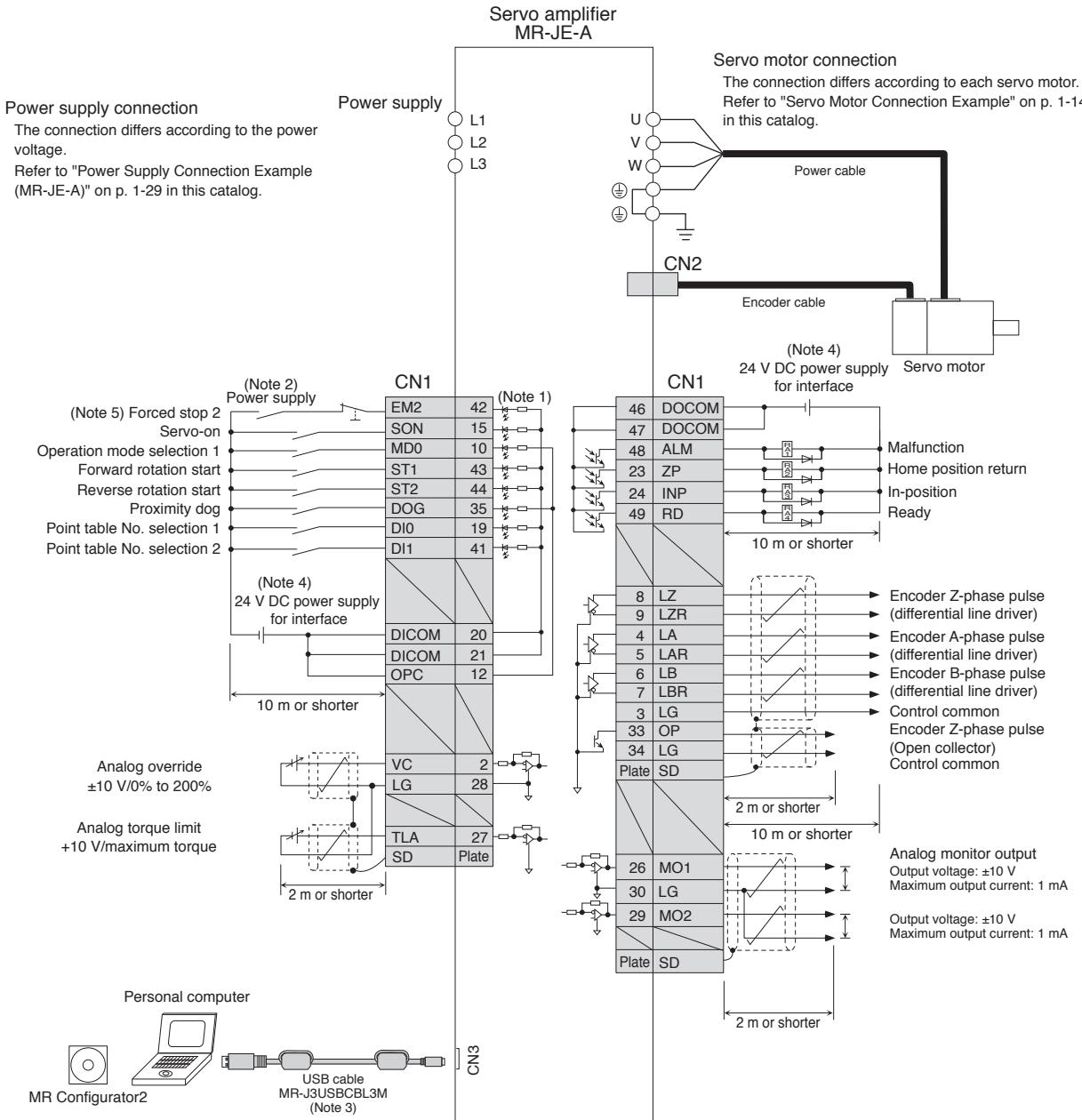
Notes: 1. This is for sink wiring. Source wiring is also possible. However, when input devices are assigned to CN1-10 pin and CN1-35 pin, be sure to use sink wiring. Source wiring is not possible in this case. In the positioning mode, input devices are assigned in the initial setting. Refer to "MR-JE\_A Servo Amplifier Instruction Manual (Positioning Mode)" for details.
