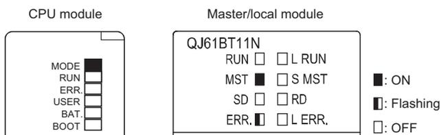
**5. The hardware test starts. During the test, the MST LED on the master/local module is flashing.**
