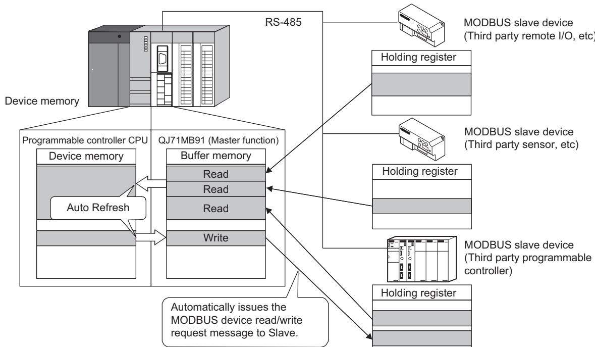
Figure 5.1 Communication using the automatic communication function
