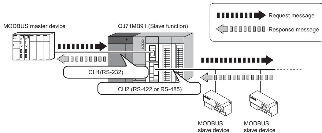
Figure 5.16 Communication using the link operation function
