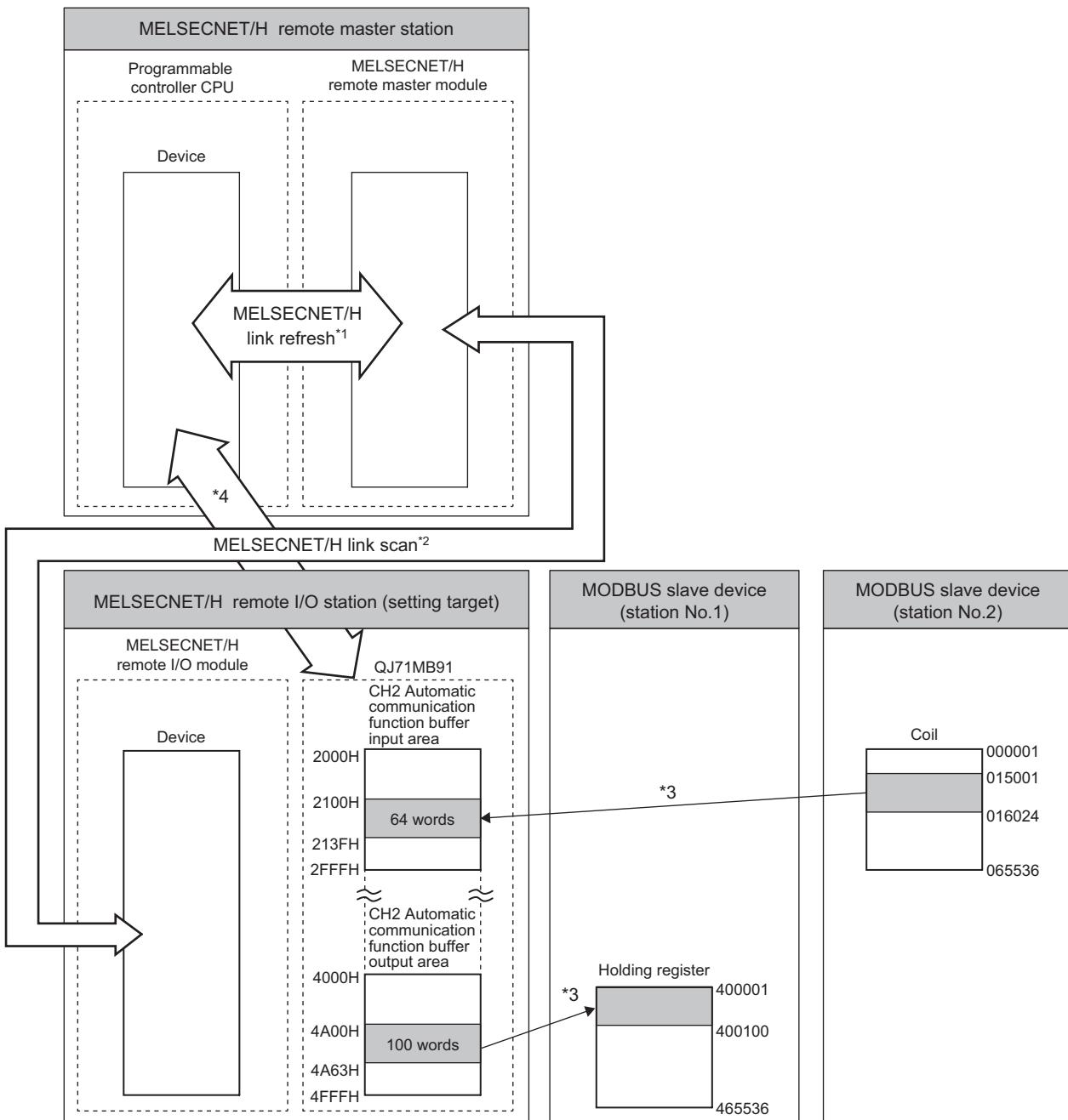
Figure 9.27 Communications (When not using GX Configurator-MB)
