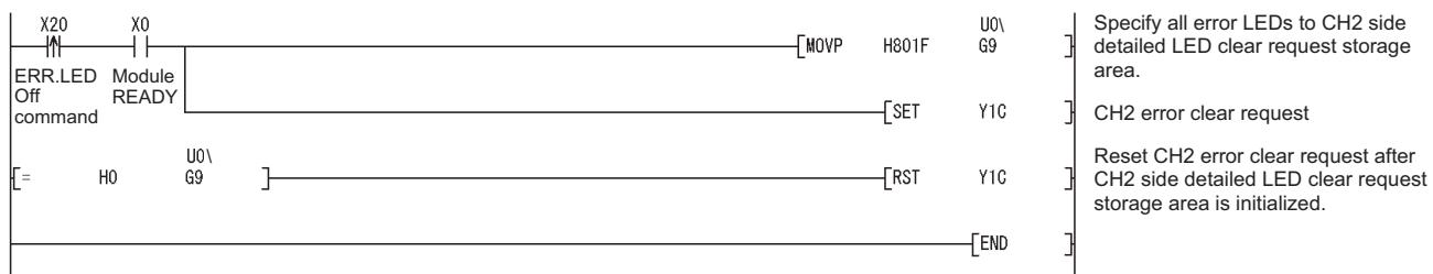
Figure 11.15 ERR. LED OFF program example
