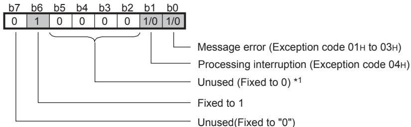
Figure 4.79 Communications event at response message transmission
