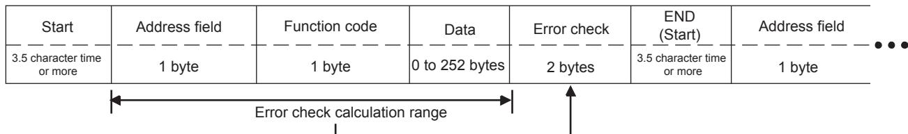
Figure 4.2 Frame in RTU mode
