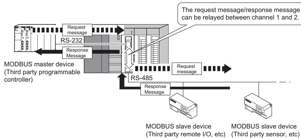
Figure 1.4 Communication using the link operation function
