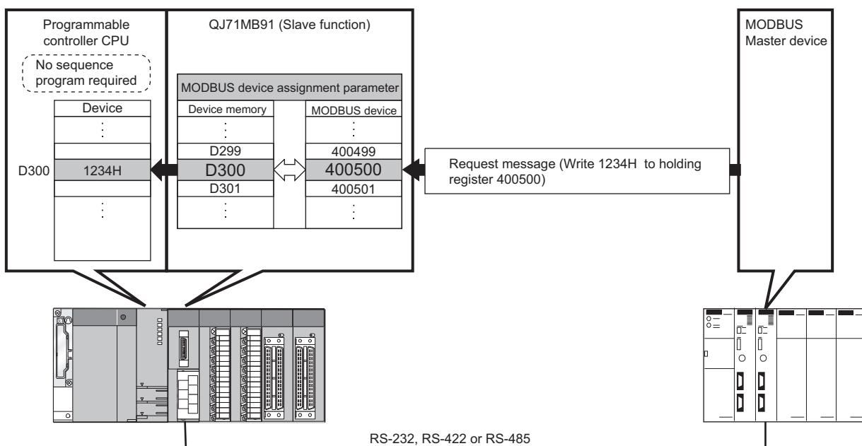
Figure 5.13 MODBUS device and programmable controller CPU device
