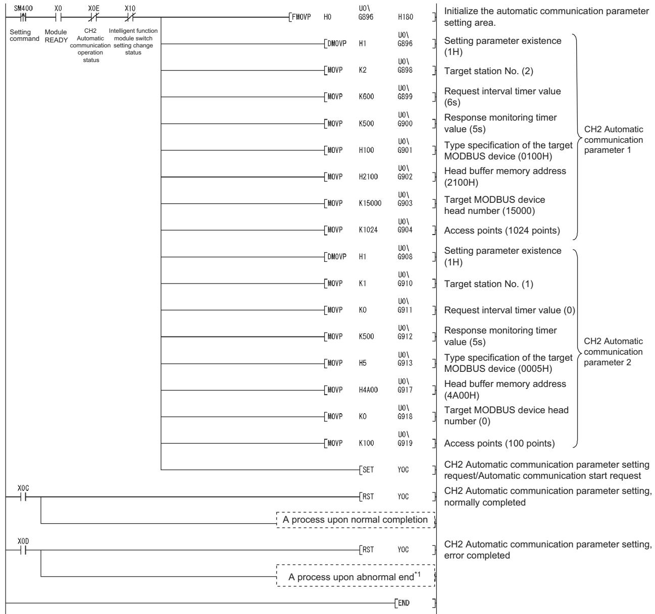
Figure 9.11 Automatic communication parameter setting program example
