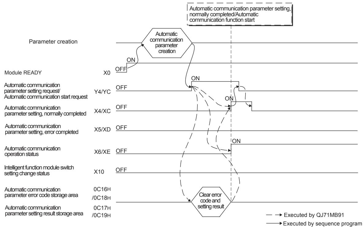
Figure 9.1 Timing chart for automatic communication parameter setting (Normal completion)
