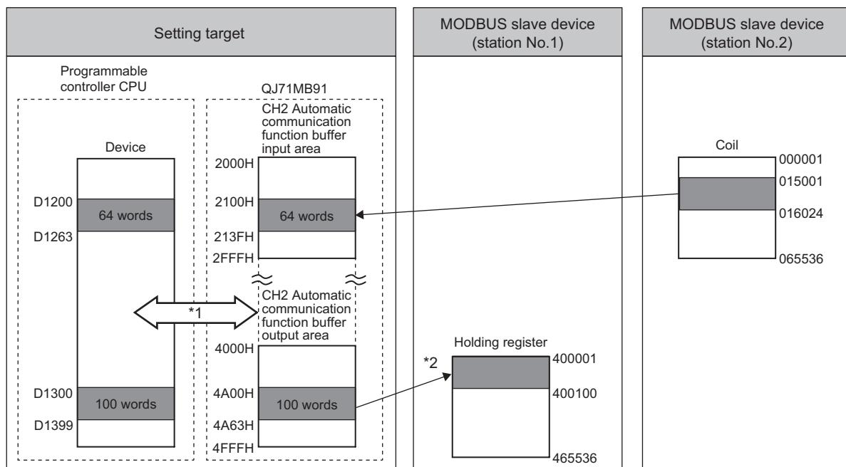
Figure 9.6 Communications with the automatic communication parameters set
