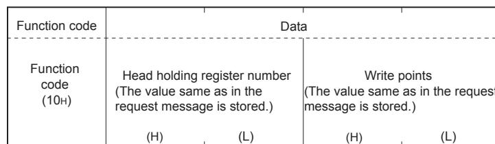
Figure 4.86 Write multiple registers (Normal response message)
