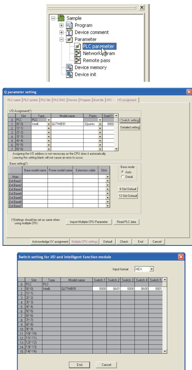
Figure 6.20 Intelligent function module switch setting procedure
