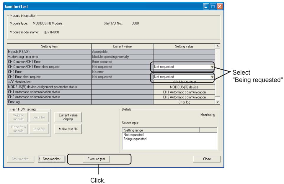
Figure 11.9 Turning off the ERR. LED on the Monitor/test screen
