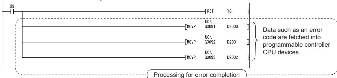
Data to be stored in the programmable controller CPU are as follows:
