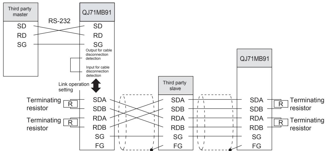
Figure 6.18 Connection (for link operation setting, 1:n communication, 4 wires) when host is slave
