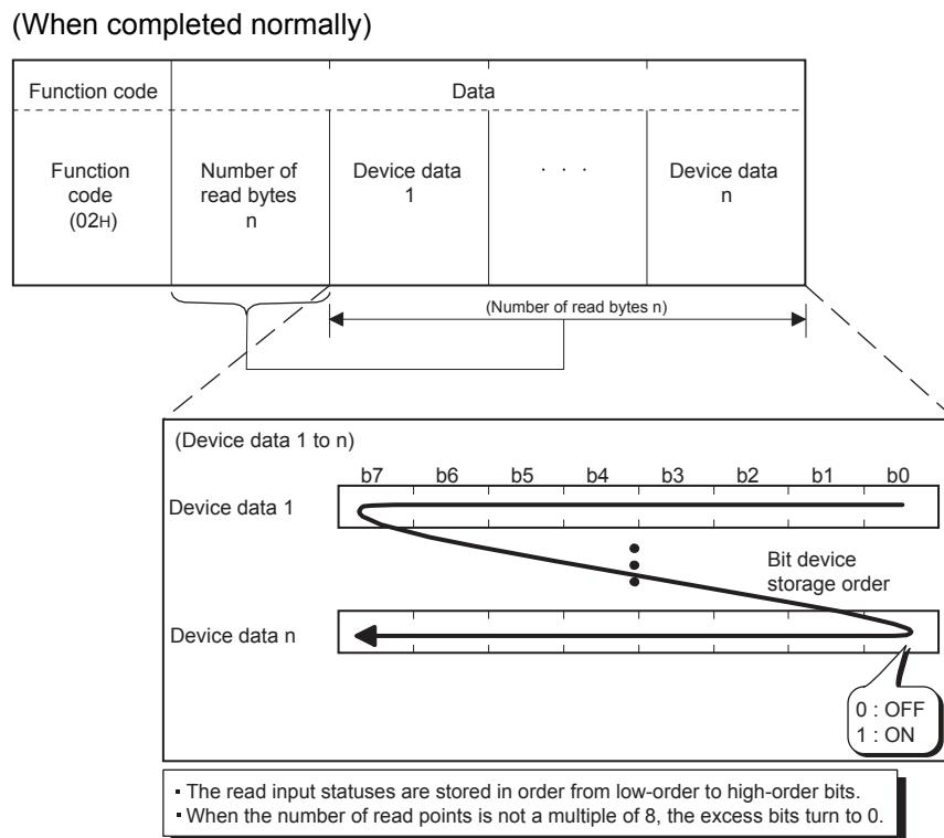
Figure 4.13 Read discrete inputs (Normal response message)
