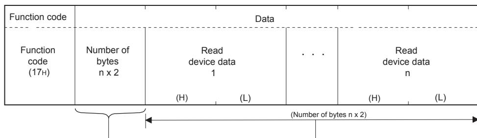
Figure 4.99 Read/Write multiple registers (Normal response message)
