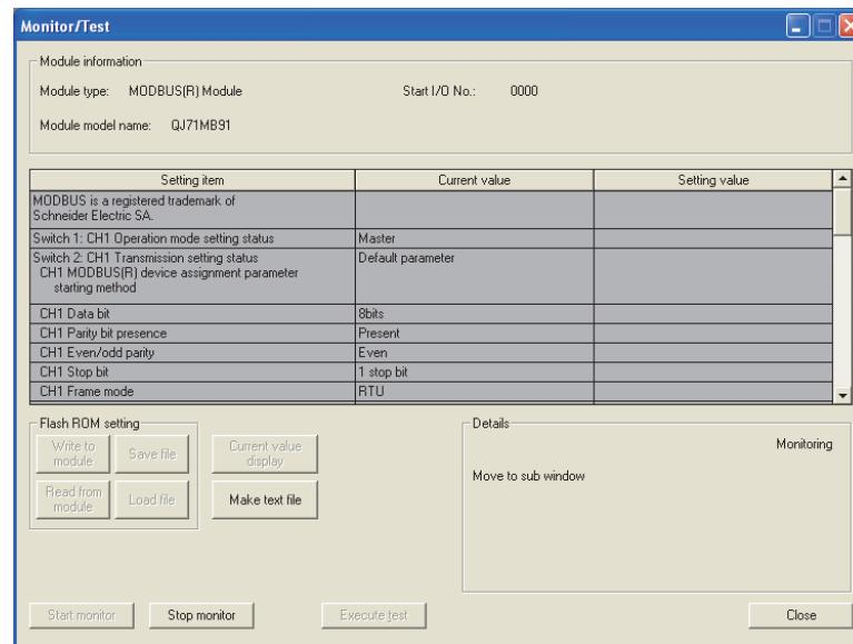
Figure 11.8 Monitor/test screen
