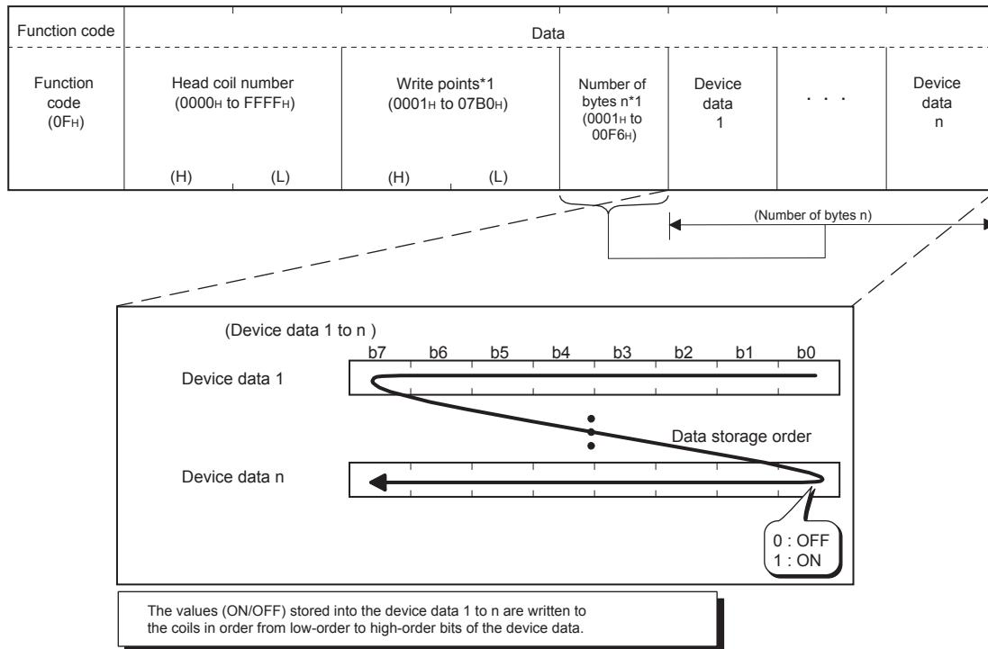
Figure 4.82 Write multiple coils (Request message)
