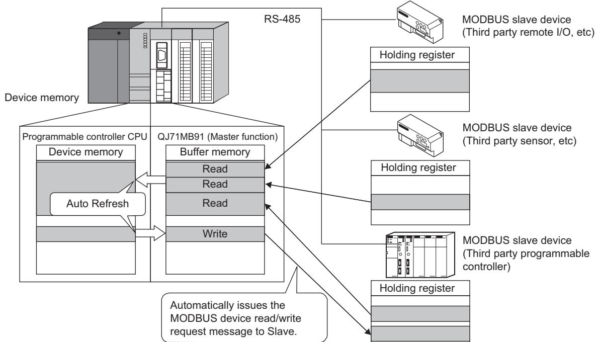
**Figure 1.1 Communication using the automatic communication function**
