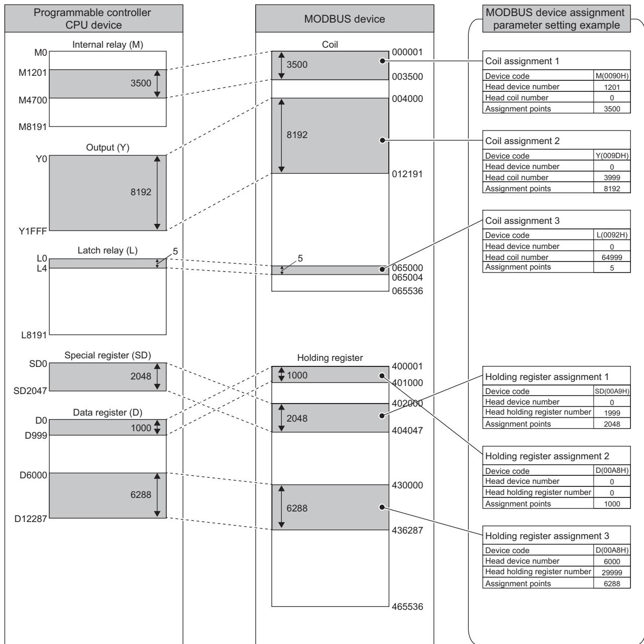
Figure 7.7 MODBUS device assignment parameter setting diagram
