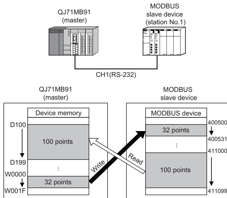
Figure 10.3 Configuration example for MBRW instruction execution
