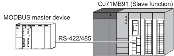
**Figure 2.6** Connecting to a master station (1:1) with a RS-422/485 line(c) Connecting to master stations (1:1) with RS-232 and RS-422/485 lines
