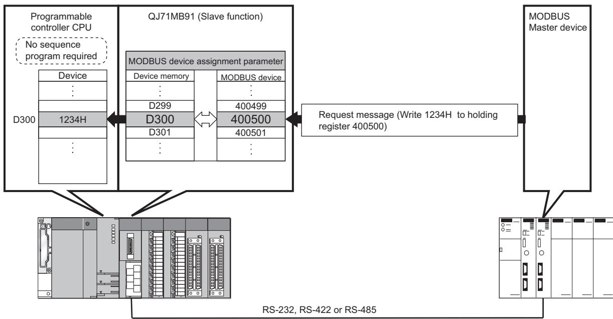
Figure 7.6 MODBUS device and programmable controller CPU device
