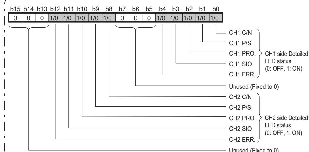
The QJ71MB91 stores the lower 8 bits of the buffer memory's Detailed LED status as a diagnostic register. (address: 0006H/0007H)
