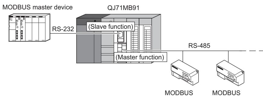
Figure 2.11 Using the RS-232 interface as the slave station and the RS-422/485 interface as the master station
