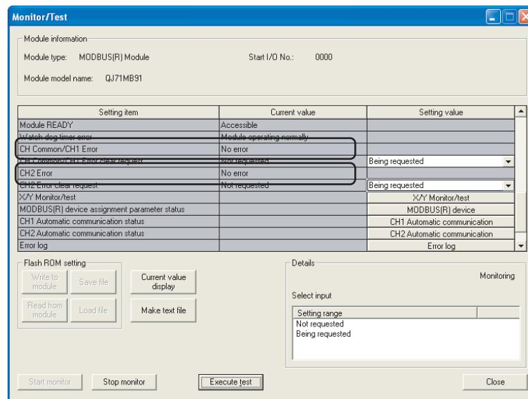
Figure 11.11 Monitor/test screen (after the ERR.LED turned off)
