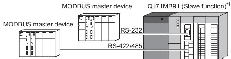
**Figure 2.7** Connecting to master stations with RS-232 and RS-422/485 lines
