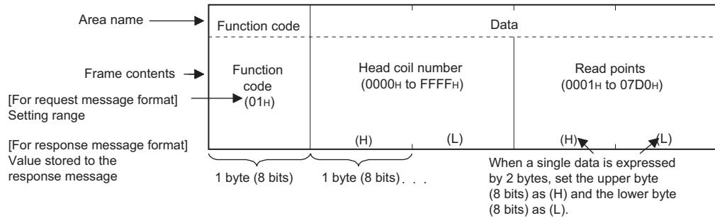
Figure 4.7 Request/Response message format diagram
