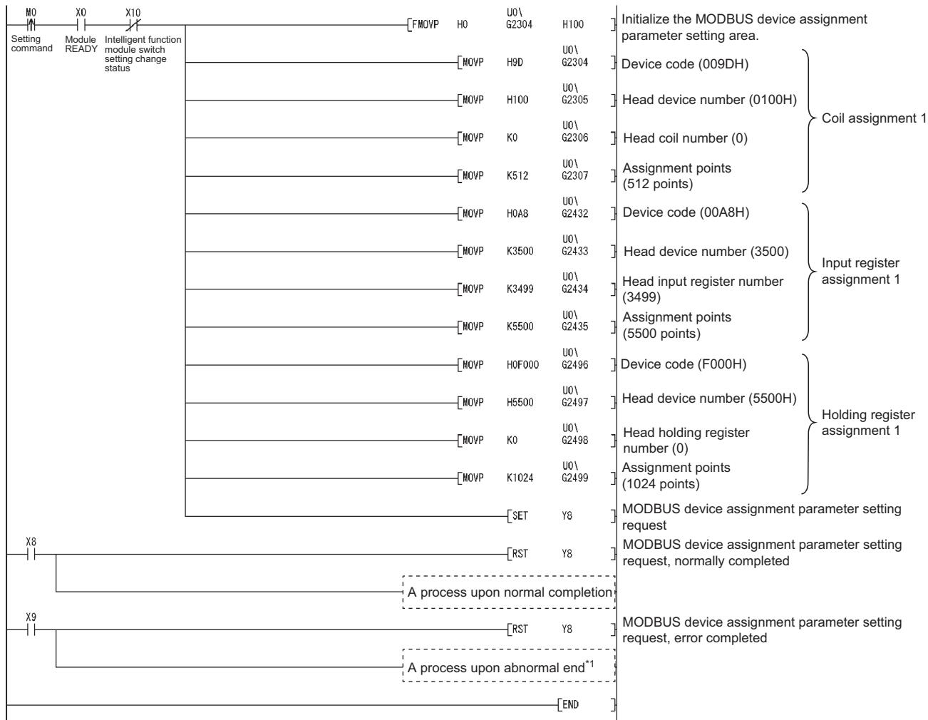
Figure 9.18 MODBUS device assignment parameter setting program example
