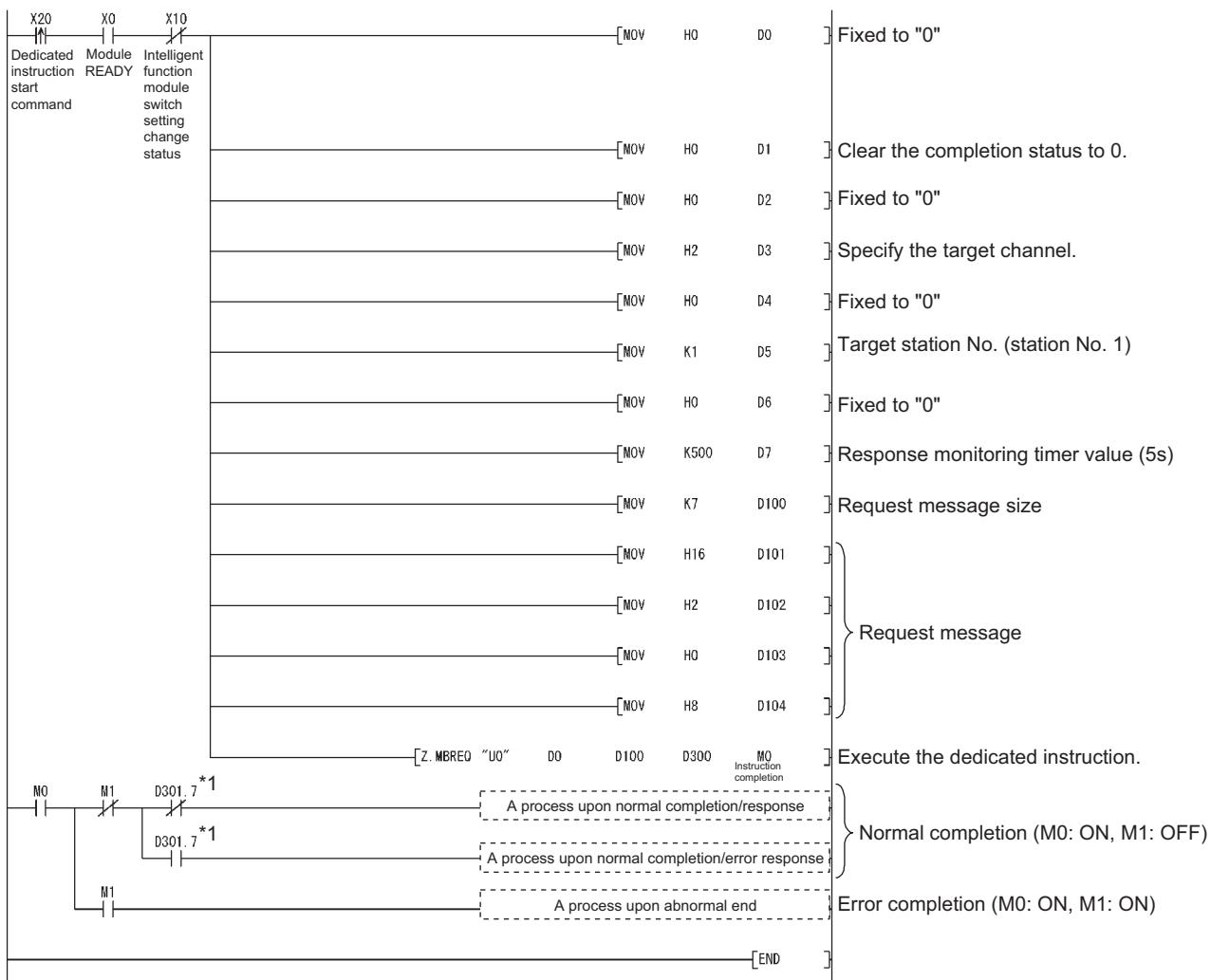
\* 1 D301.7 is the most significant bit of the function code to be stored in the response message.
