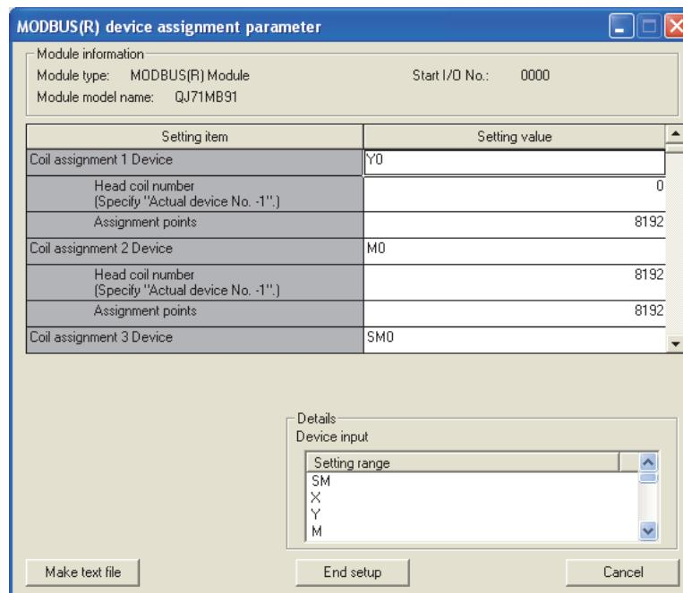
Figure 8.9 MODBUS device assignment parameter setting screen
