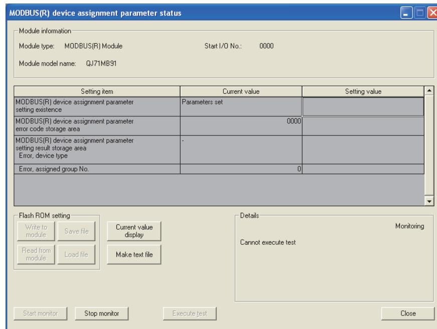
Figure 8.14 MODBUS device assignment parameter status screen
