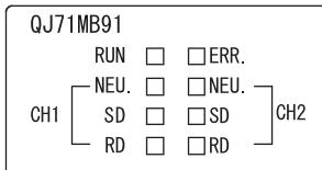
Figure 6.3 QJ71MB91 LEDs
