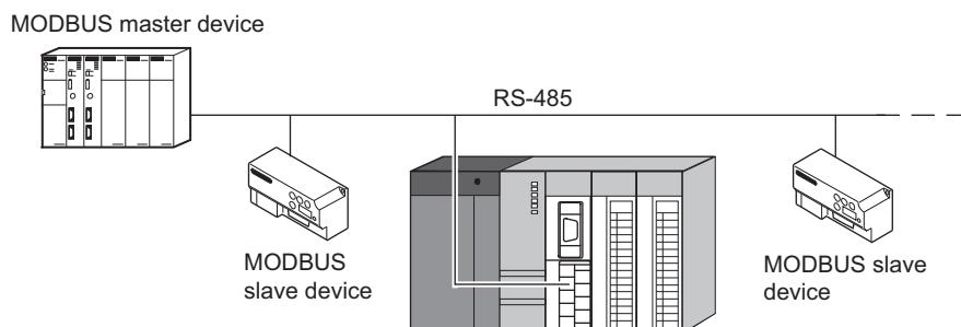
**Figure 2.8** Connecting to a master station (1:n)
