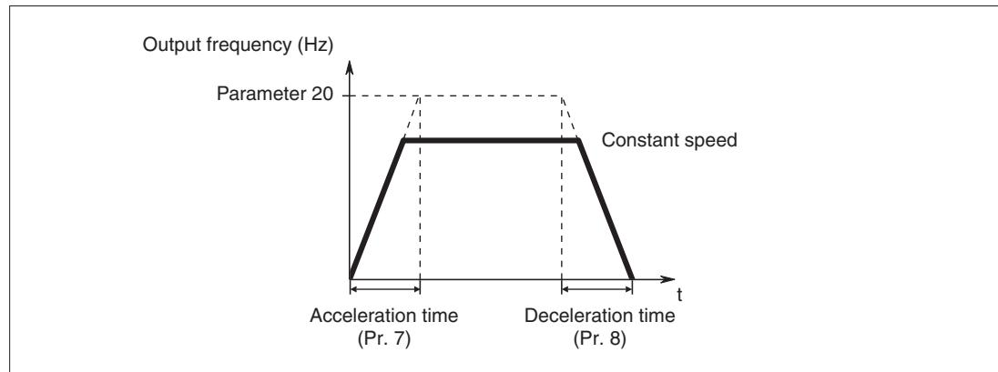
Parameter 7 sets the acceleration time for the drive. The value defines the time in seconds in which the drive will be accelerated up from 0 Hz to the frequency preset in parameter 20.
