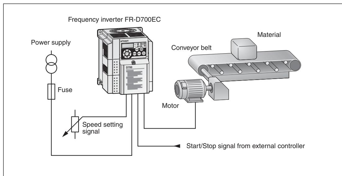
The belt is started and stopped by an external controller (for example a PLC). The speed of the motor and thus of the conveyor belt can be adjusted with a setpoint potentiometer.
