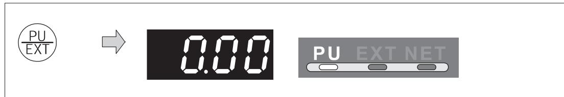
Pressing PU/EXT when the inverter is in control unit mode switches the system to external operation mode and the EXT indicator lights up.
