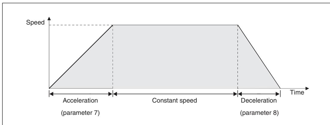
In this example we are going to use an FR-D700 series inverter to power and control the belt using the speed/time pattern shown in the graph above. The configuration is as follows:
