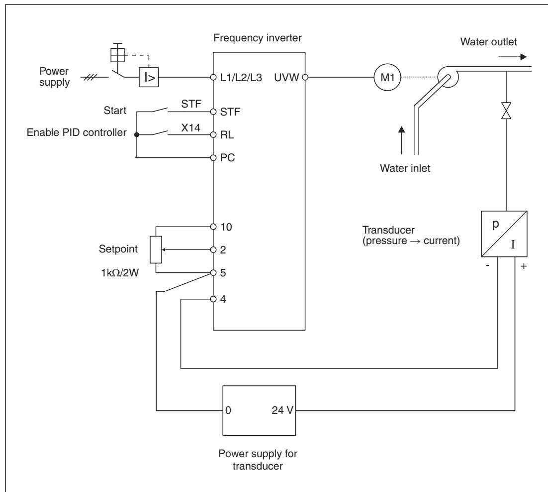
For the PID controller application using the configuration shown above you must also set the inverter parameters shown in the table below, in addition to the basic parameters.
