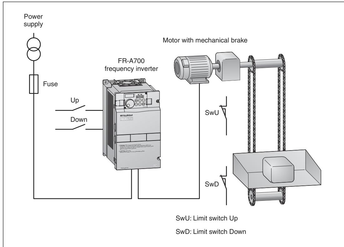
In the wiring diagram on the next page the mechanical brake is controlled via the RUN terminal. The frequency at which the brake is released can be set with parameter 13.
