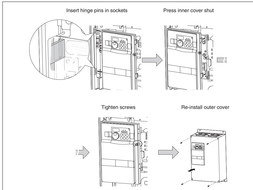
**Removing and replacing on models from FR-F746-00023 through FR-F746-01160****● Removing the front cover**
