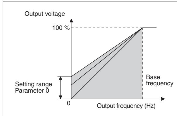
You can use parameter 0 to achieve better performance for starting the motor under load. The base frequency is set in parameter 3.
