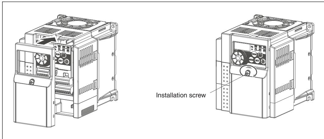
**Removing and replacing on models FR-D740-120 and FR-D740-160****● Removing the front cover**
