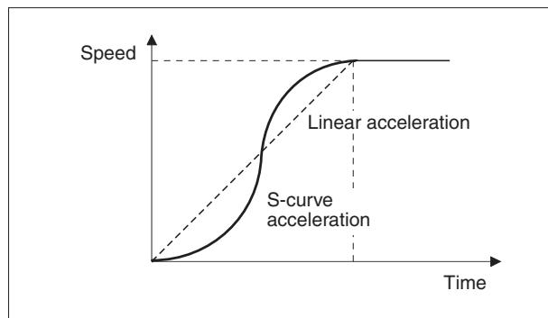
If the material on the belt still shifts when stopping and starting even with a gentle acceleration curve you can solve the problem by programming an S-curve for acceleration and deceleration, as shown in the graph on the left.
