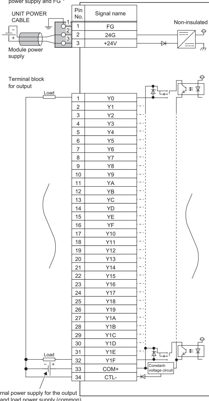
\*1 Only one wire can be inserted into a wire insertion opening for the terminal block for module power supply and FG. Multiple wires cannot be connected to a terminal. Connecting two or more wires may cause a poor contact.
