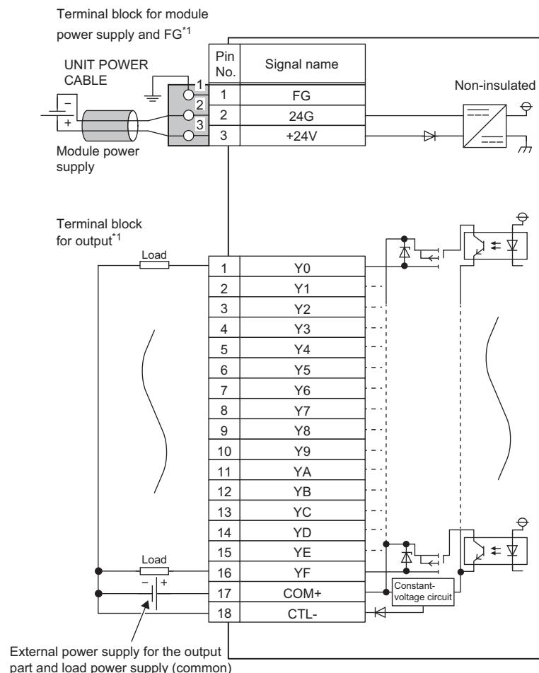
\*1 Only one wire can be inserted into a wire insertion opening for the terminal block for module power supply and FG. Multiple wires cannot be connected to a terminal. Connecting two or more wires may cause a poor contact.
