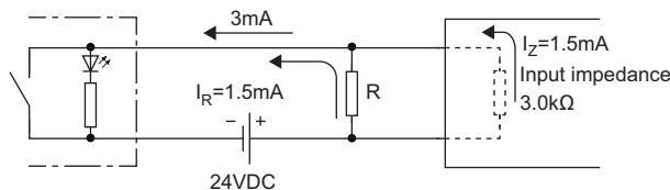
2. To satisfy the condition that the OFF current of NZ2GN2B1-32D is 1.5mA or lower, the current through the connected resistor should be 1.5mA or higher. From the formula below, the connected resistor (R) is lower than 3.0kΩ.
