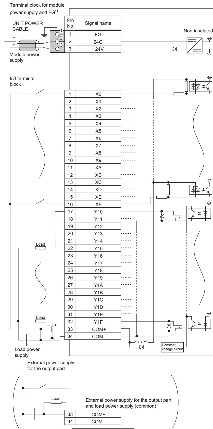
\*1 Only one wire can be inserted into a wire insertion opening for the terminal block for module power supply and FG. Multiple wires cannot be connected to a terminal. Connecting two or more wires may cause a poor contact.
