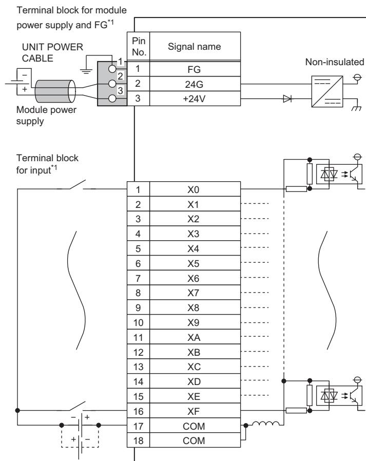
\*1 Only one wire can be inserted into a wire insertion opening for the terminal block for module power supply and FG. Multiple wires cannot be connected to a terminal. Connecting two or more wires may cause a poor contact.
