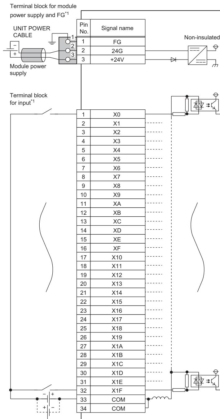
\*1 Only one wire can be inserted into a wire insertion opening. Multiple wires cannot be connected to a terminal. Connecting two or more wires may cause a poor contact.
