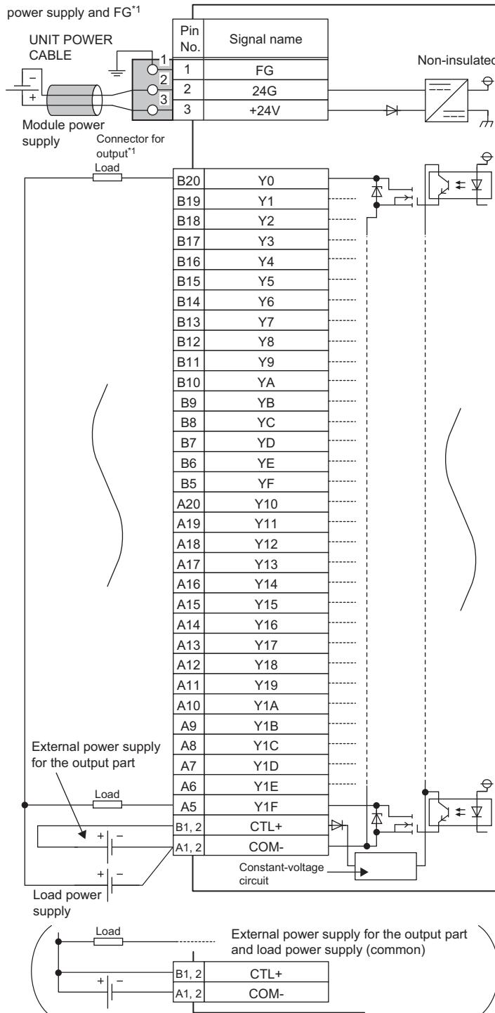
\*1 Only one wire can be inserted into a wire insertion opening for the following: terminal block for module power supply and FG, connector for output. Multiple wires cannot be connected to a terminal. Connecting two or more wires may cause a poor contact.
