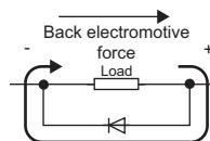
Action 2. Configure a sneak current path by connecting a diode across positive and negative of the external power supply. When taking the action described in Example 1 at a time, connect a diode parallel to C1 and R1.
