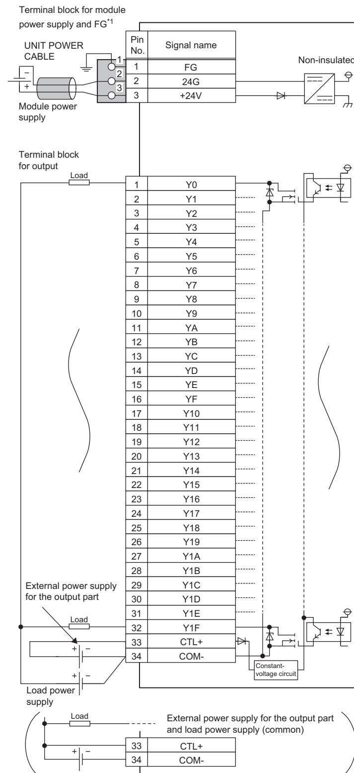
\*1 Only one wire can be inserted into a wire insertion opening for the terminal block for module power supply and FG. Multiple wires cannot be connected to a terminal. Connecting two or more wires may cause a poor contact.
