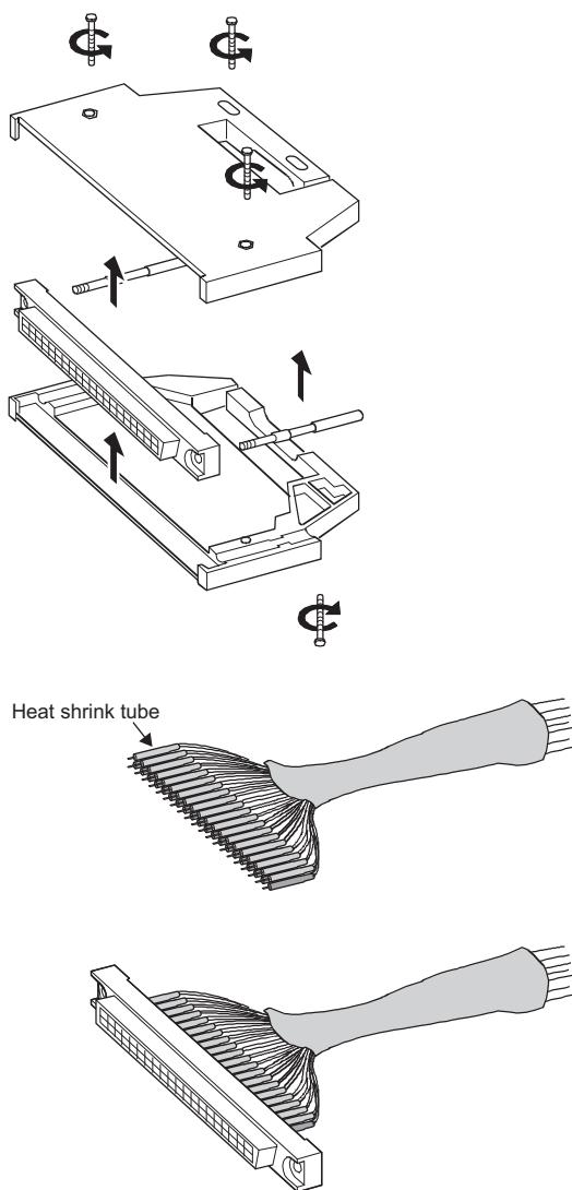
1. Loosen four screws of the connector and remove the screws.
