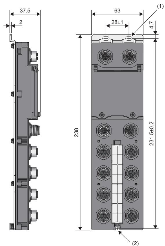
(1) 2-4.5 × 8 slotted hole (M4 mounting screw)
