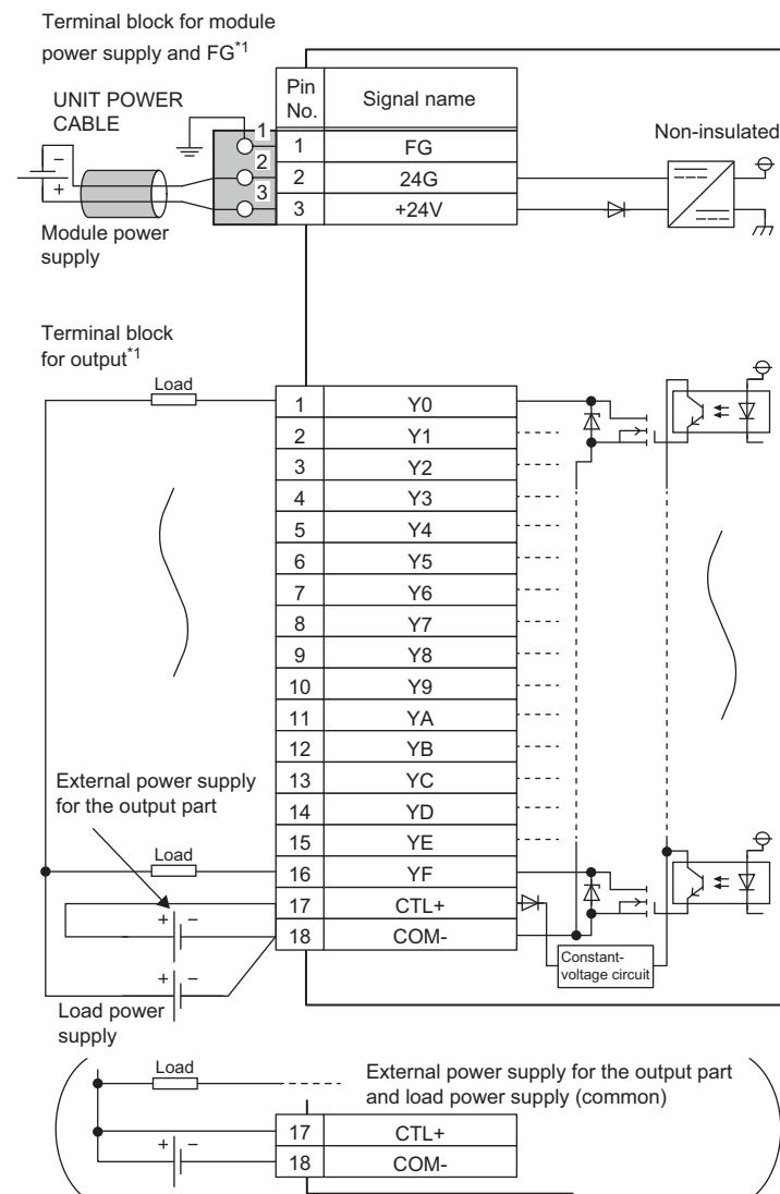
\*1 Only one wire can be inserted into a wire insertion opening. Multiple wires cannot be connected to a terminal. Connecting two or more wires may cause a poor contact.
