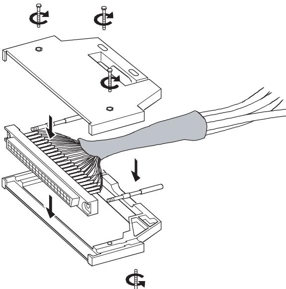
5. Place the body in one of the cover and insert the fixing screws into the screw holes. After that, fit the other cover on the body.
