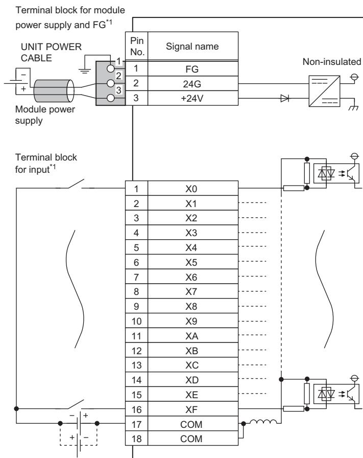
\*1 Only one wire can be inserted into a wire insertion opening. Multiple wires cannot be connected to a terminal. Connecting two or more wires may cause a poor contact.
