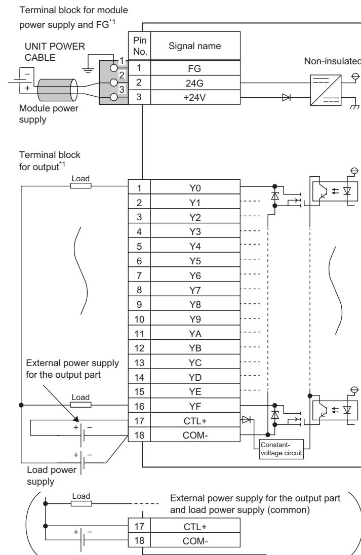
\*1 Only one wire can be inserted into a wire insertion opening for the terminal block for module power supply and FG. Multiple wires cannot be connected to a terminal. Connecting two or more wires may cause a poor contact.
