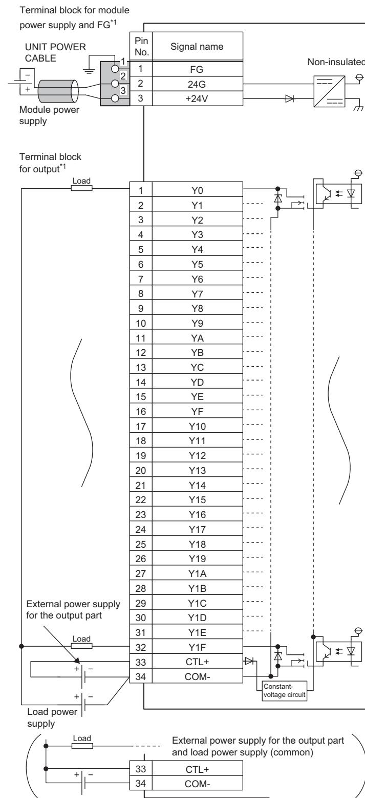
\*1 Only one wire can be inserted into a wire insertion opening. Multiple wires cannot be connected to a terminal. Connecting two or more wires may cause a poor contact.
