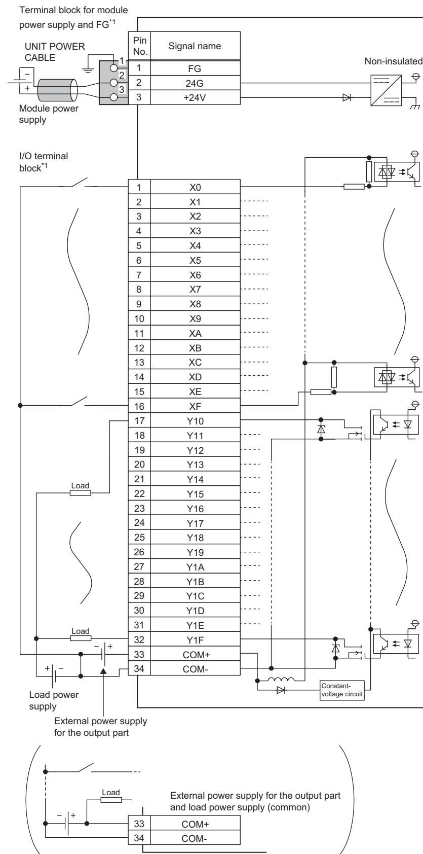
\*1 Only one wire can be inserted into a wire insertion opening. Multiple wires cannot be connected to a terminal. Connecting two or more wires may cause a poor contact.
