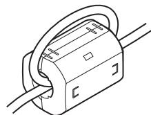
When using the I/O module (waterproof module) with the shielded cables not grounded on the module side, attach a ferrite core to signal wires to prevent the noise induced to the cables from affecting a load connected to the module.
