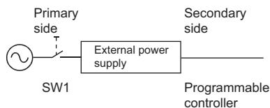
When installing the switch to the secondary side, connect a capacitor and resistor, and increase the rise time (10ms or more).
