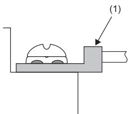
1. Loosen the terminal screw. Connect the round solderless terminal (1) as it is.
