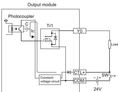
When the external power supply is powered on rapidly, the current (Ic) flows due to the stray capacitance(C).
