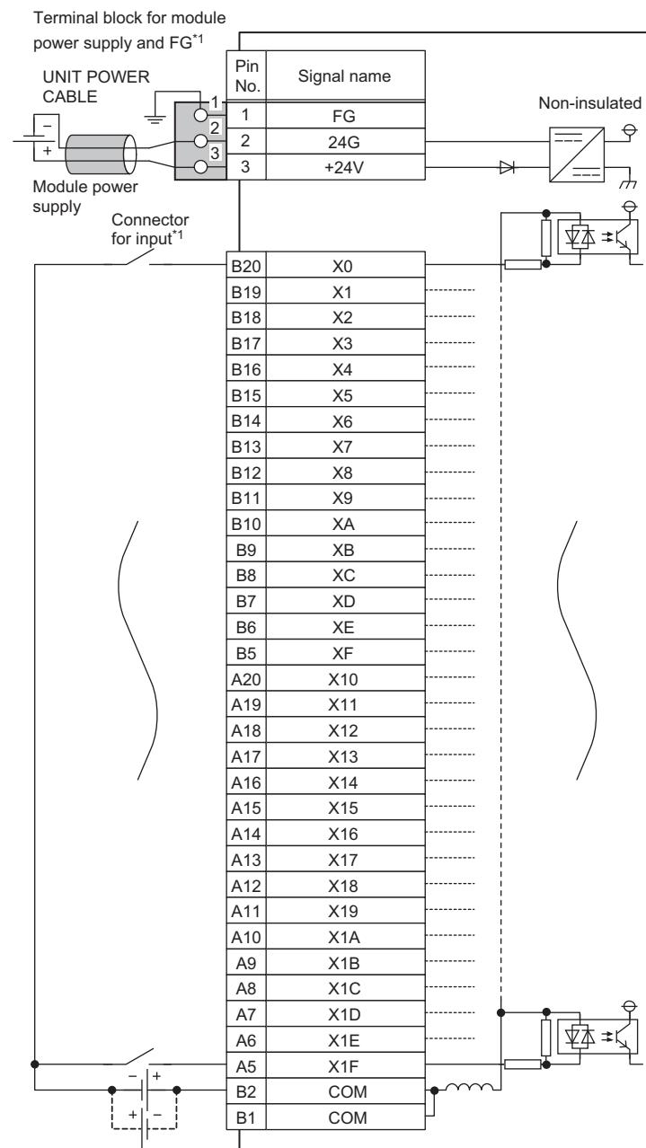
\*1 Only one wire can be inserted into a wire insertion opening for the following: terminal block for module power supply and FG, connector for input. Multiple wires cannot be connected to a terminal. Connecting two or more wires may cause a poor contact.
