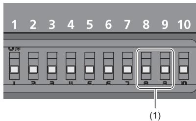
(1) Function setting switch 8 and function setting switch 9
