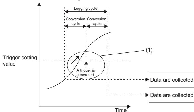
(1) The data at the timing when a trigger is generated is not stored in the buffer memory area.
