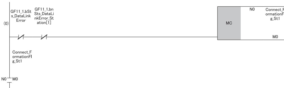
(0) Checks the data link status of the remote head module (station number 1).
