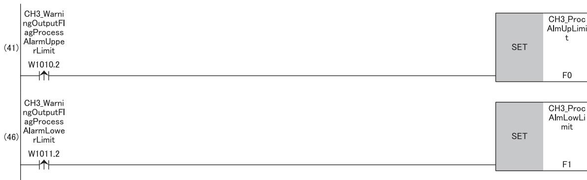
(41)Performs a processing of when a warning (process alarm upper limit) has occurred in CH3.
