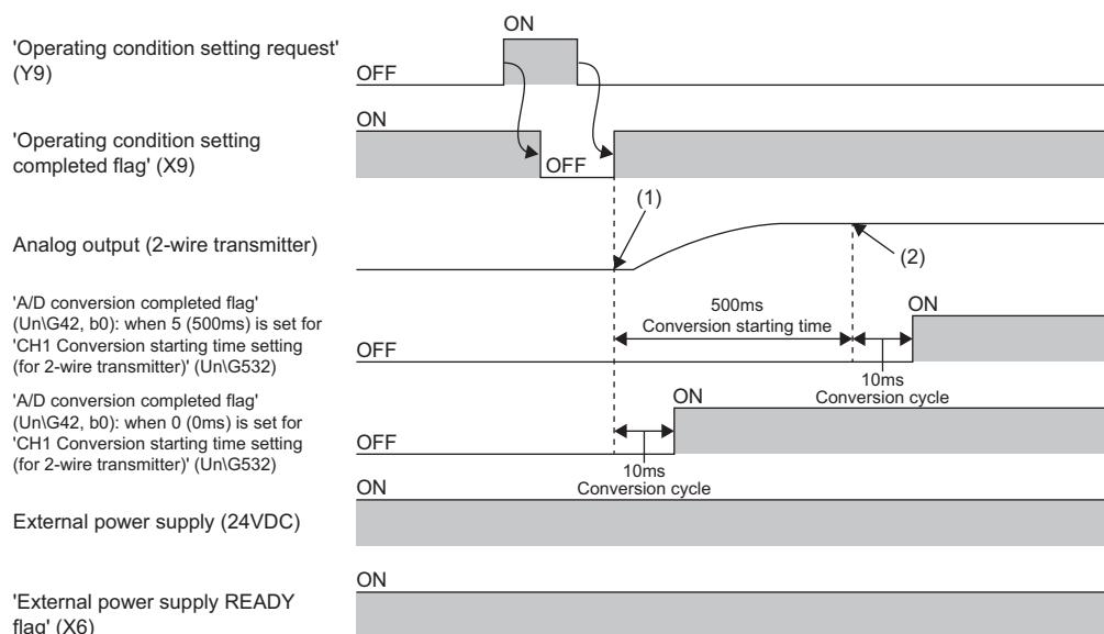
(1) When the conversion start time is 0ms, A/D conversion starts at that point.
