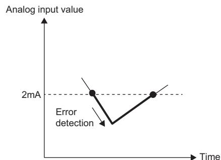
The settings for 'CH1 Input signal error detection lower limit set value' (Un\G529) and 'CH1 Input signal error detection upper limit set value' (Un\G530) are ignored.
