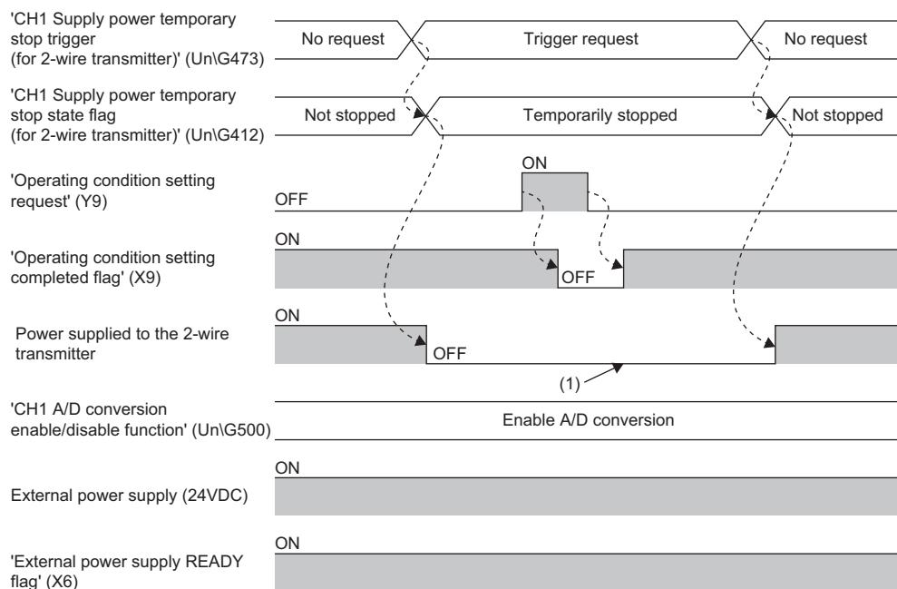
(1) Because 'CH1 Supply power temporary stop trigger (for 2-wire transmitter)' (Un\G473) is set to Trigger request (1), the supply power to the 2-wire transmitter is not turned on.
