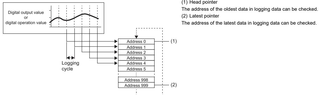
Logging data are stored in the buffer memory area. When the number of stored data points is 1001 or greater, data is sequentially overwritten from address 0 with new data.
