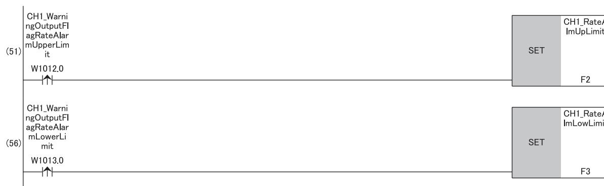
(51)Performs a processing of when a warning (rate alarm upper limit) has occurred in CH1.
