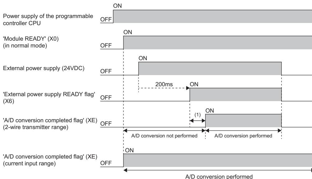
(1) A/D conversion processing is not performed until the time set in 'CH1 Conversion start time setting (for 2-wire transmitter)' (Un\G532) is passed.
