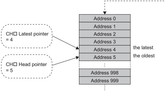
'CH1 Head pointer' (Un\G434) does not change until 'CH1 Logging data' (Un\G10000 to Un\G10999) becomes full after the logging start. (Fixed to 0)
