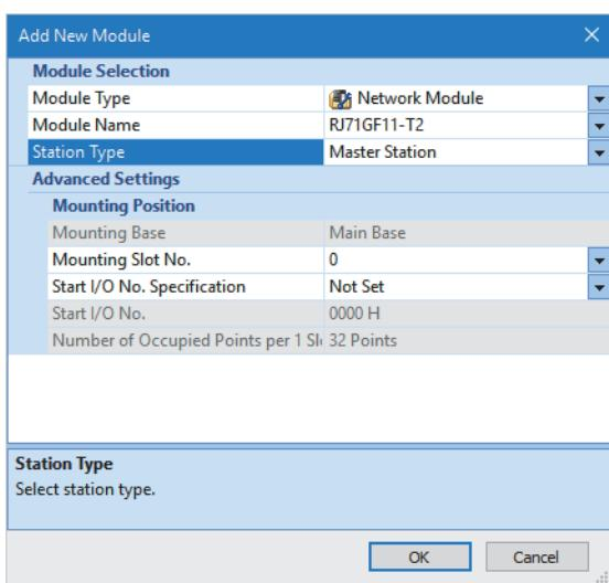
5. Click the [OK] button in the following window to add the module labels of the master/local module.
