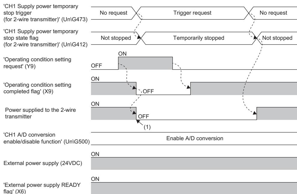
(1) Because 'CH1 Supply power temporary stop trigger (for 2-wire transmitter)' (Un\G473) is set to Trigger request (1) while 'Operating condition setting request' (Y9) is on, the supply power to the 2-wire transmitter is turned off.
