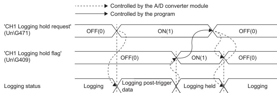
Logging does not stop when 'CH1 Logging hold request' (Un\G471) is changed from on to off before ON (1) is stored in 'CH1 Logging hold flag' (Un\G409).
