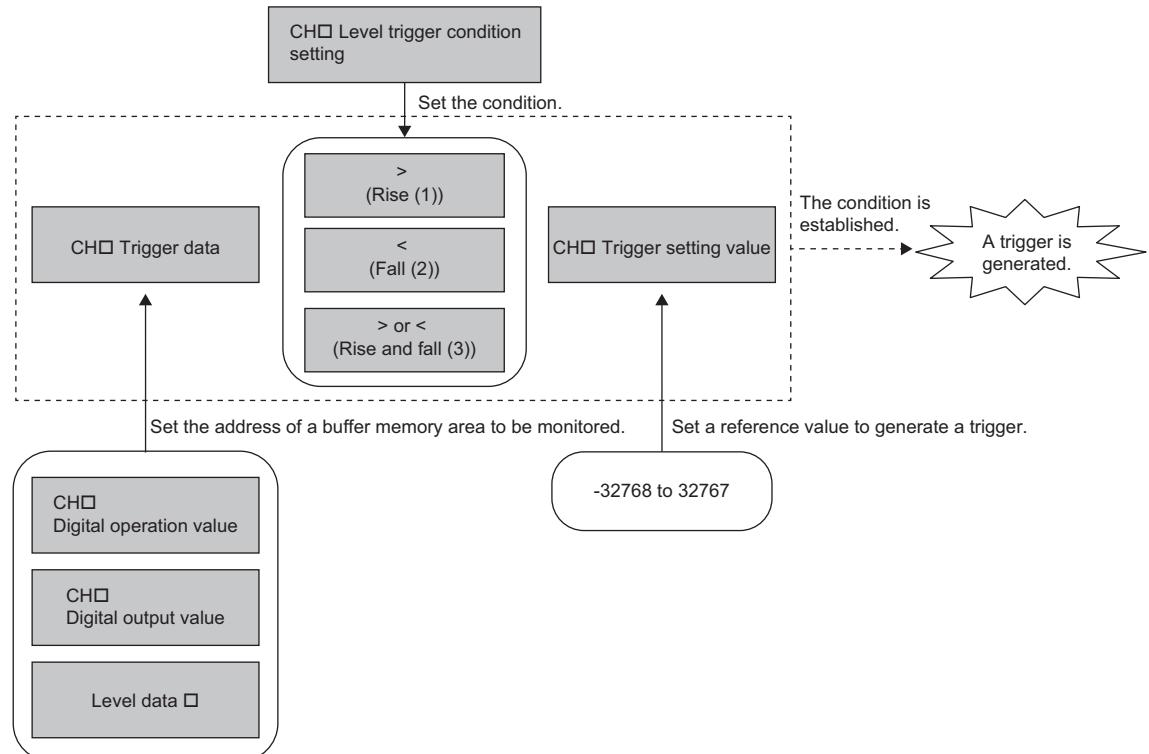
To generate a hold trigger when a value in 'CH1 Digital output value' (UnlG400) is greater than 10000, set as follows.
