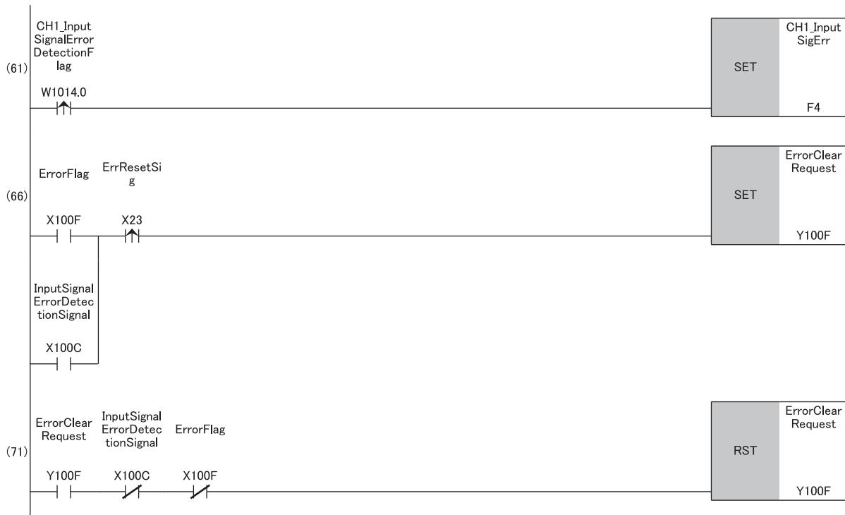
(61)Performs a processing of when an input signal error was detected in CH1.
