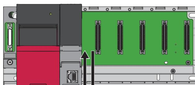
2. Power off the programmable controller, and replace the A/D converter module with a new one.
