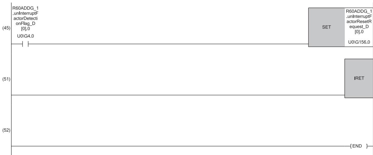
(45) Turn off Interrupt factor mask [0] when Interrupt factor detection flag turns on.
