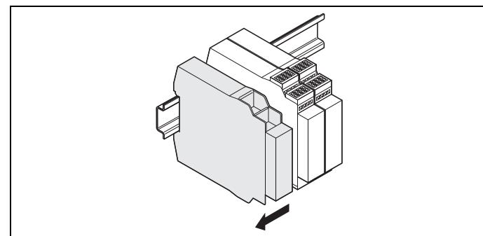
⇒ If there are several modules, slide the modules away from each other individually in the direction of the arrow until the side plug connection is separated.
