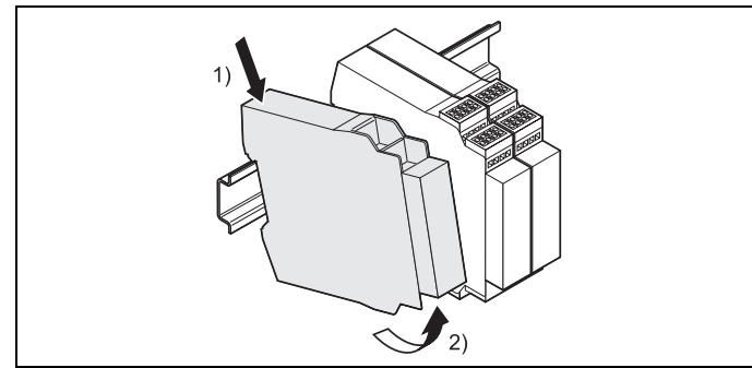
⇒ Press the module downwards at the rear (1) and remove it from the DIN rail in the direction of the arrow while keeping it pressed down (2).
