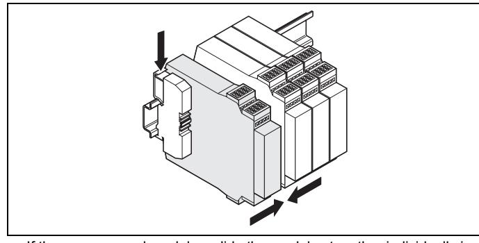
⇒ If there are several modules, slide the modules together individually in the direction of the arrow until the side plug connection latches in.
