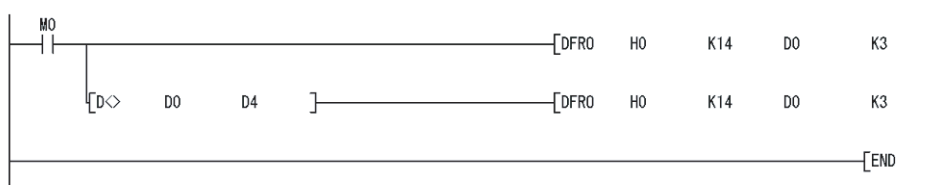
Figure 5.13 Periodic pulse counter value reading program example
