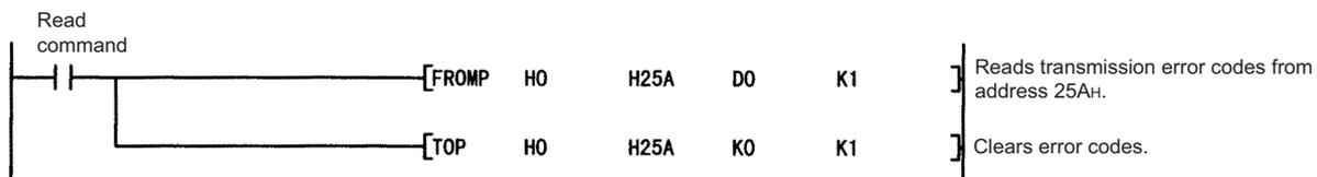
Check the error codes and take corrective actions according to Page 277, Section 15.2.
