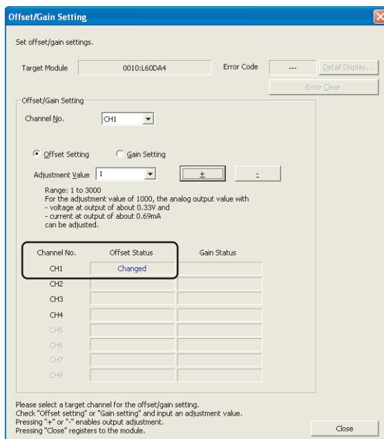
6. Clicking the or button finely adjusts the analog output voltage value or analog output current value corresponding to the set adjusted value.
