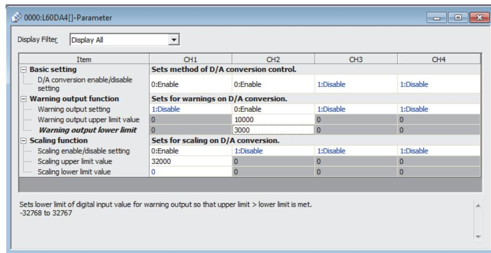
6. Display the Auto Refresh setting window for the D/A converter module (L60DA4) and configure the setting as follows.
