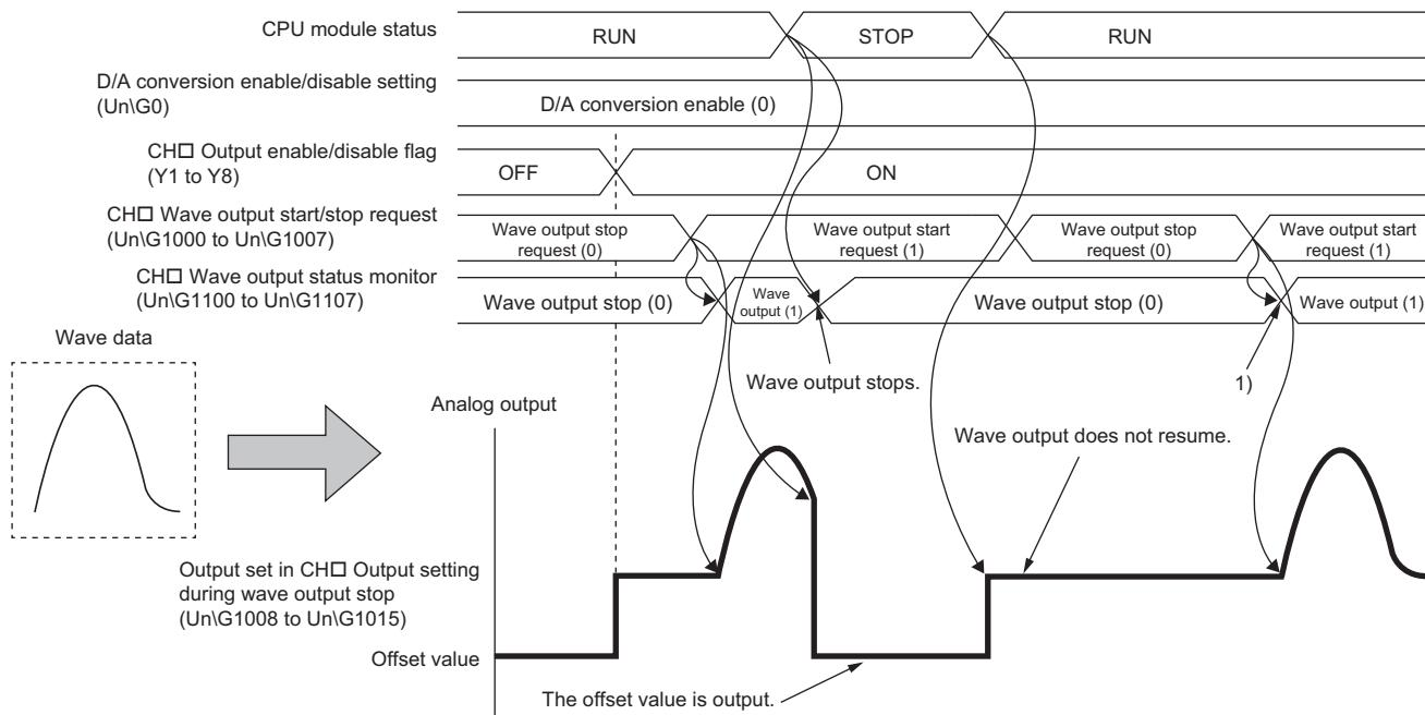
1): Wave output starts when the value set in CH□ Wave output start/stop request (Un\G1000 to Un\G1007) is changed from Wave output stop request (0) to Wave output start request (1).
