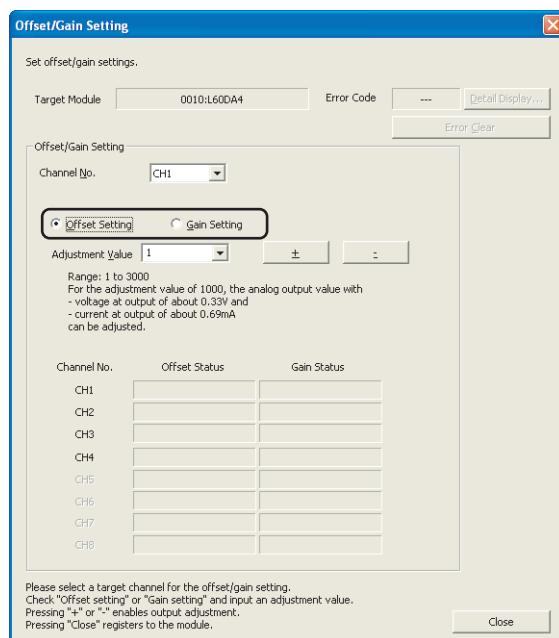
**4. Use the radio button to specify whether to perform the offset setting or gain setting. (Step 5 and later describe when the offset setting is specified.)**
