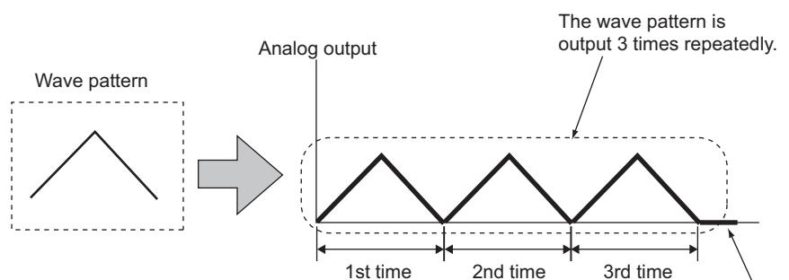
After the wave pattern was output 3 times, wave output stops and an analog value is output according to the setting in CH□ Output setting during wave output stop (Un\G1008 to Un\G1015).
