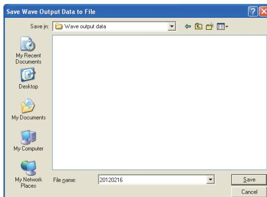
The saved wave pattern and parameter setting of the wave output function can be opened by clicking the
