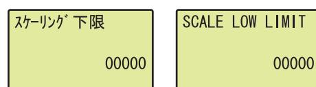
3. Move the cursor using the **◀** and **▶** buttons, and then increment or decrement the value at the cursor by 1, using the **▲** and **▼** buttons. Press the **OK** button.
