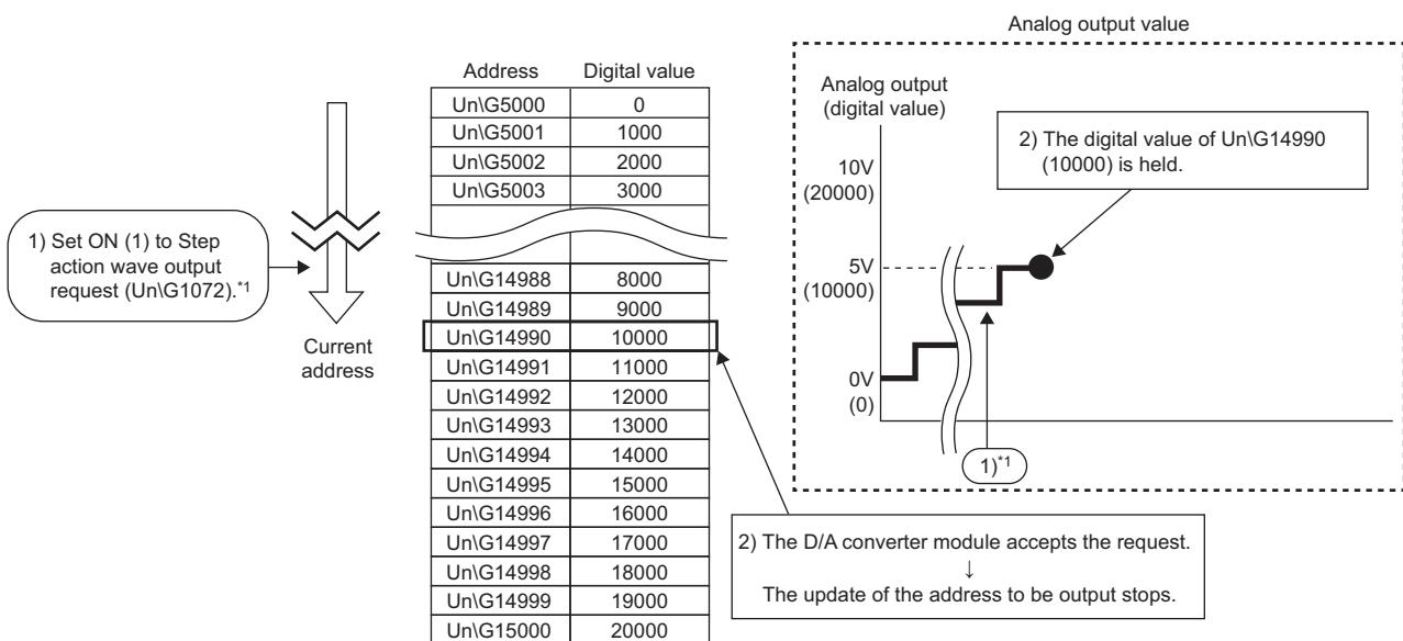
\*1 1) The contents described here is the case when the wave output status is the wave output at the timing of 1). If the wave output status is other than the wave output, following operations are performed at the timing of 2).
