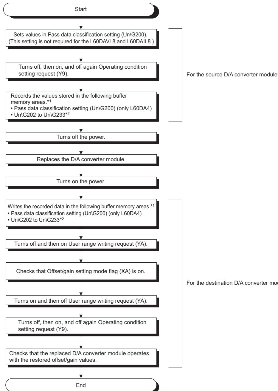
\*1 When replacing modules, you can prevent the saved offset/gain value data from getting deleted, by doing one of the following before turning the power off:
