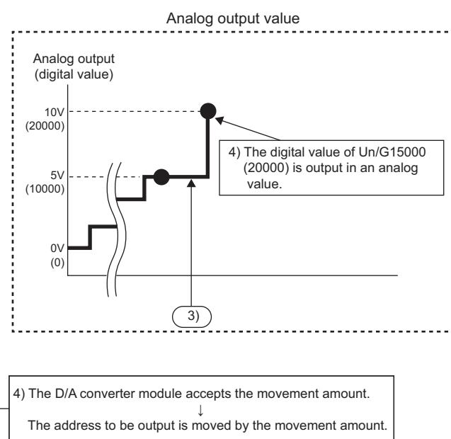
3 Change the digital value (in the address 14994) to 10000, and set CH□ Wave output step action movement amount (Un\G1080 to Un\G1087) to -6 (reverse run direction).
