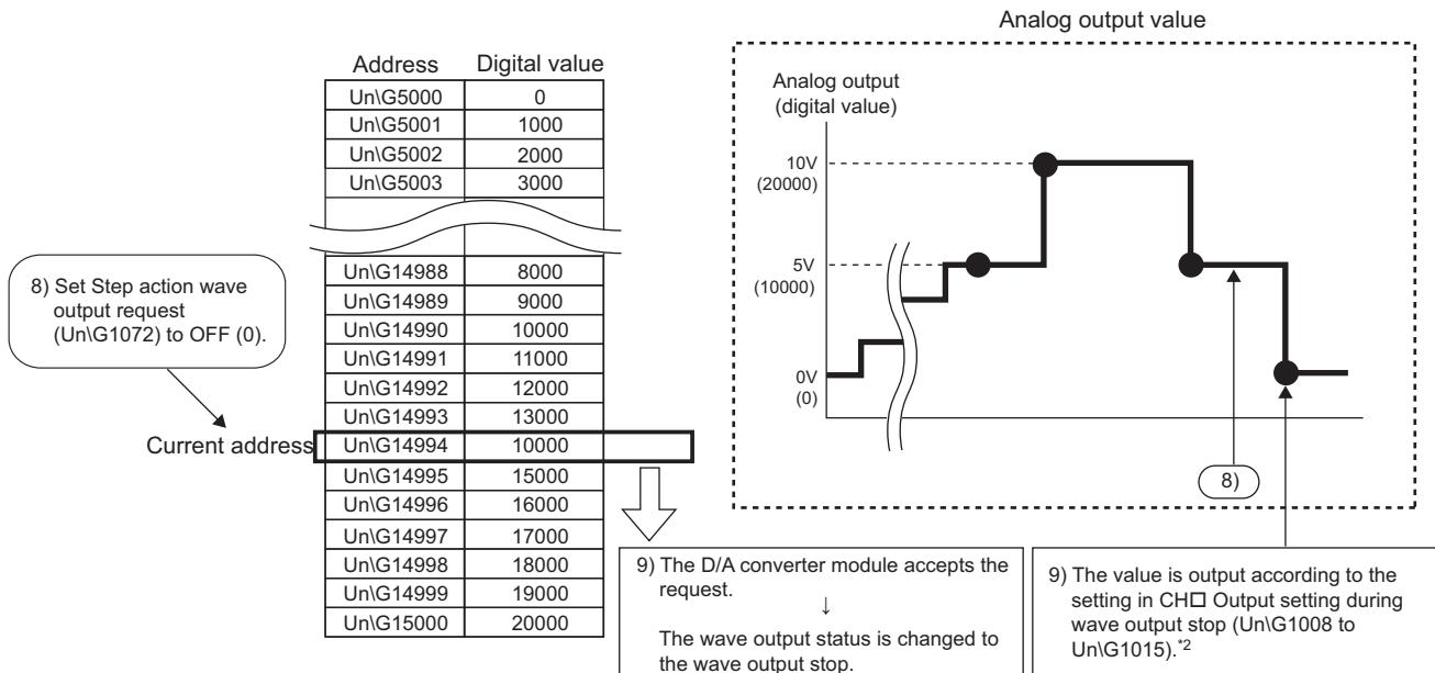
\*2 This graph shows the value when CH□ Output setting during wave output stop (Un\G1008 to Un\G1015) is set to 0V/0mA (0).
