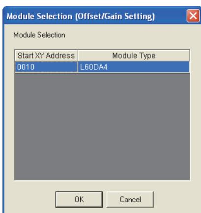
1. Select the module to configure the offset/gain setting, and click the button.
