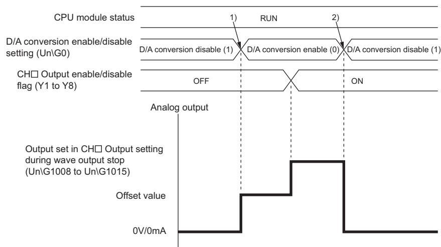
1): Set D/A conversion enable/disable (Un\G0) to D/A conversion enable (0), and turn on then off Operating condition setting request (Y9).
