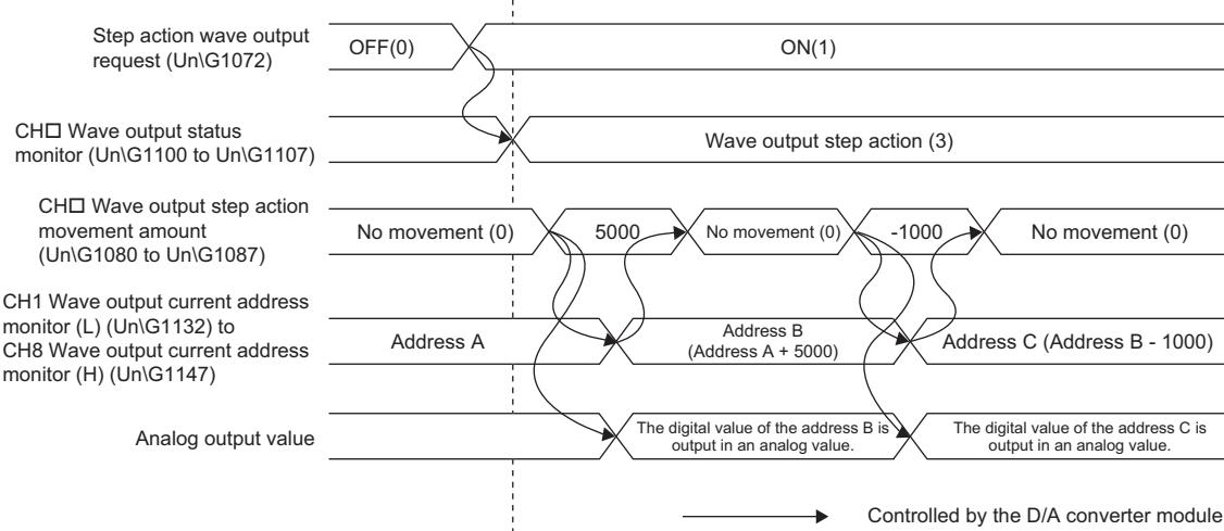
Set Step action wave output request (Un\G1072) OFF (0) → ON (1) to set the wave output status to the wave output step action.
