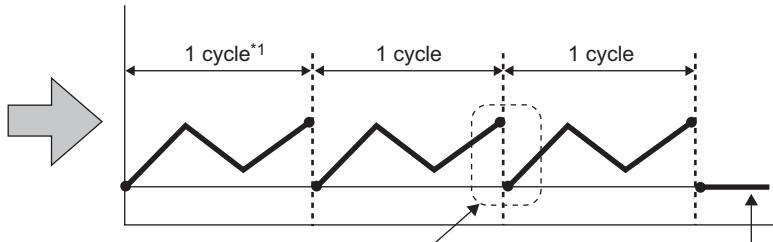
The digital values of the end point and the start point of the next iteration are consecutively output in an analog value.
