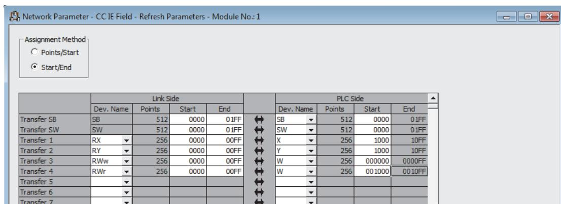
5. Write the set parameter to the CPU module of the master station and reset the CPU module, or turn off and on the programmable controller power supply.
