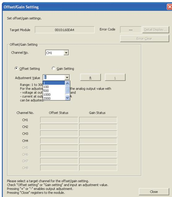
5. The adjustment amount of the offset value or gain value can be selected from "1", "100", "500", "1000", "2000", and "3000" or it can be set by inputting any value (1 to 3000).
