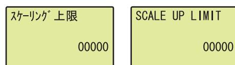
2. Move the cursor using the **◀** and **▶** buttons, and then increment or decrement the value at the cursor by 1, using the **▲** and **▼** buttons. Press the **OK** button.
