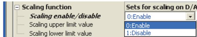
3. Set values for "Scaling upper limit value" and "Scaling lower limit value".
