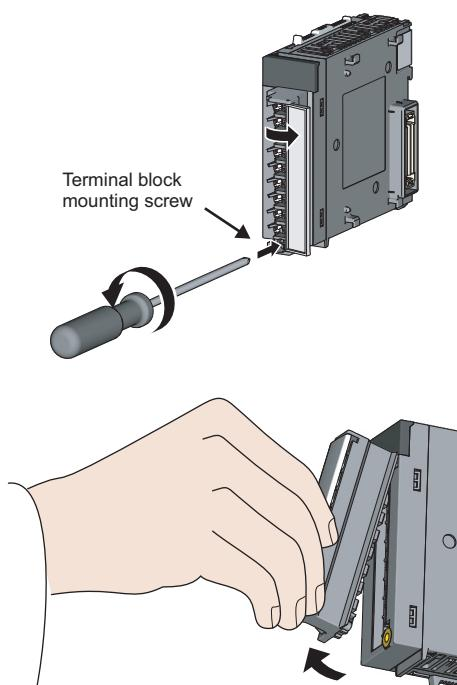
1. Open the terminal cover and loosen the terminal block mounting screw.
