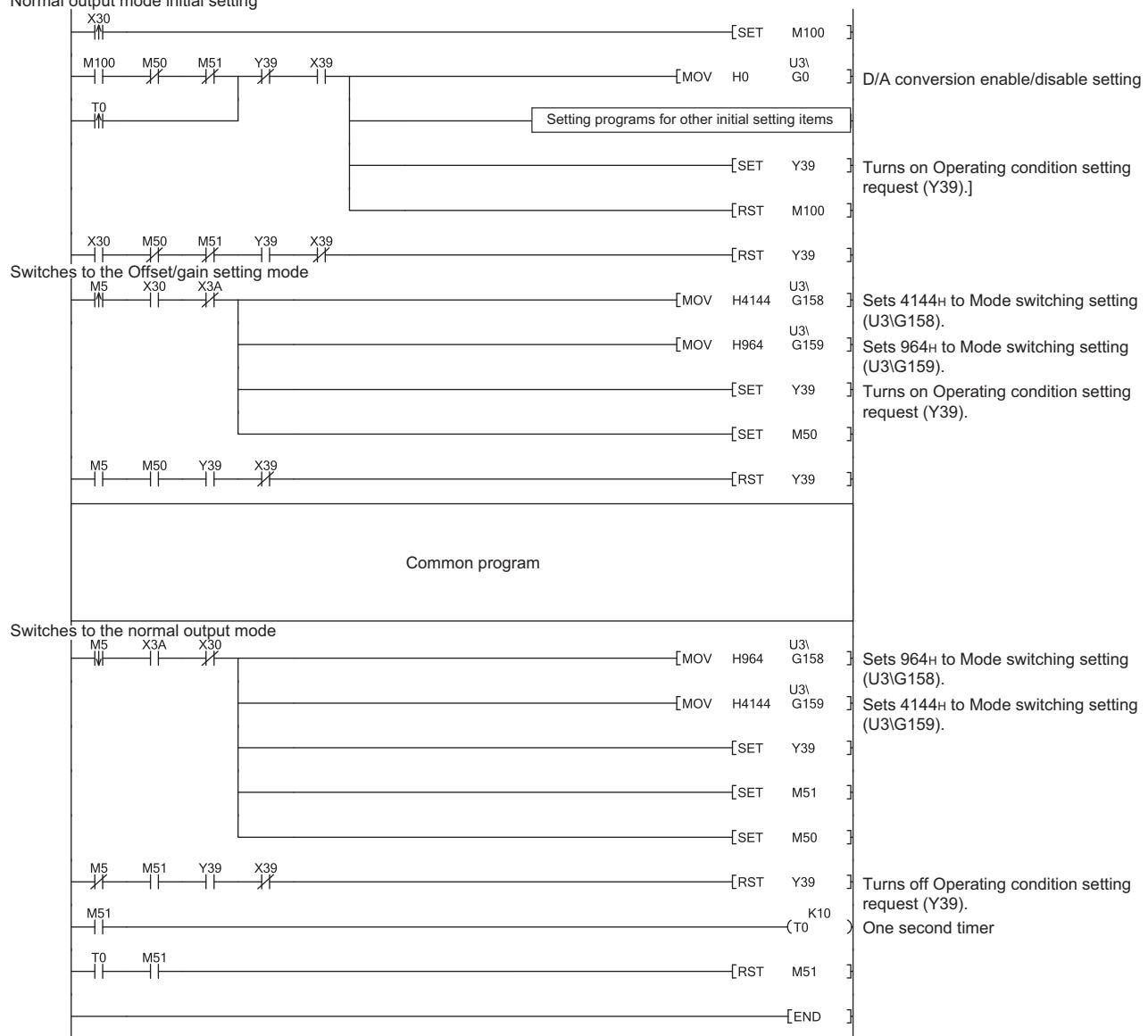
**(d) Switching the mode by using the switch setting**
