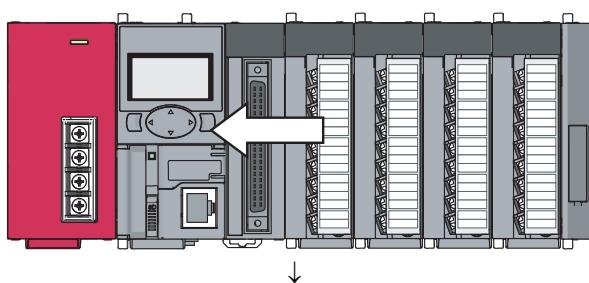
**2. Apply the offset/gain values to modules No.2 to No.4.**
