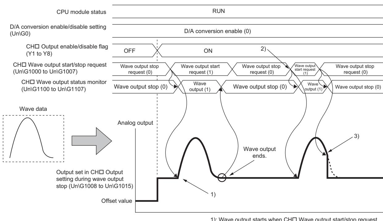
1): Wave output starts when CH□ Wave output start/stop request (Un\G1000 to Un\G1007) is set to Wave output start request (1).
