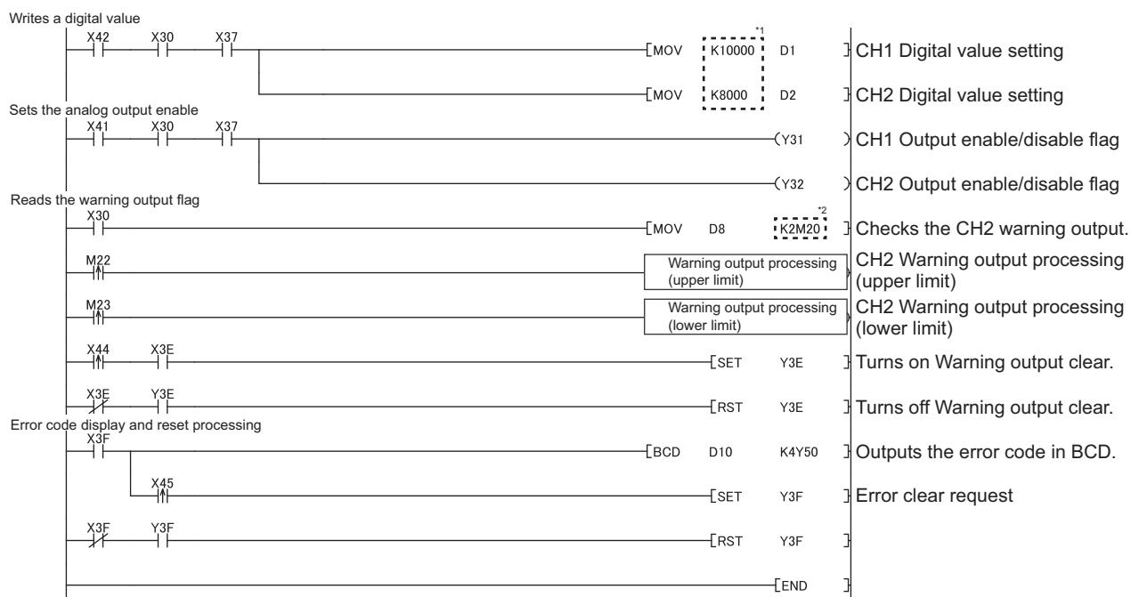
\*1 When using the L60DAVL8 or L60DAIL8, set a value according to the digital value range of the output range used.
