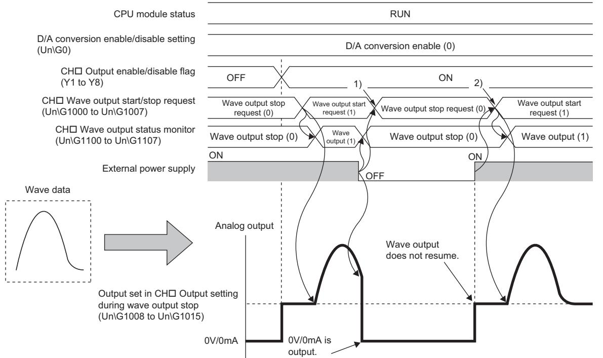
1): Because the external power supply was turned off and wave output stopped, change the value set in CH□ Wave output start/stop request (Un\G1000 to Un\G1007) to Wave output stop request (0).
