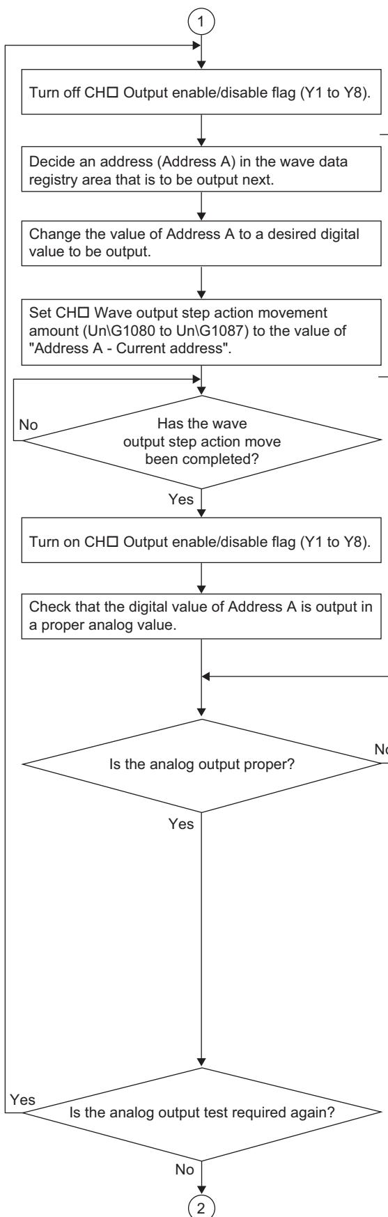
Example of testing analog output in CH1
