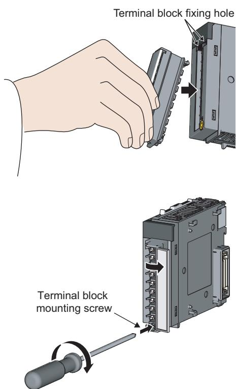
1. Fully insert the projections on the top of the terminal block into the terminal block fixing holes and press the terminal block until it snaps into place.
