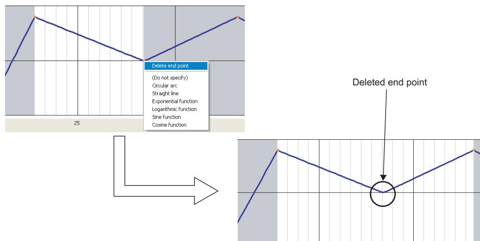
**6. Set the wave between end points from the right-click menu or in "Specify wave" of "Wave details setting".**
