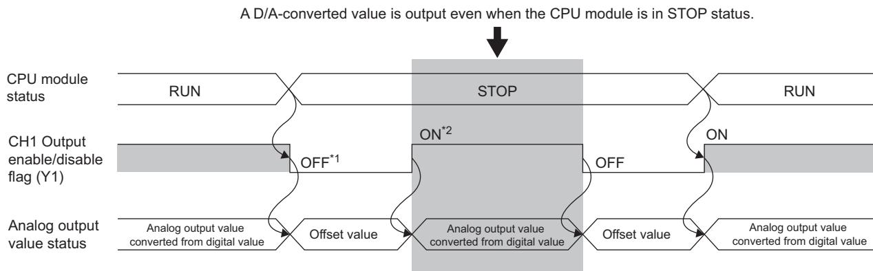
\*1 CH1 Output enable/disable flag (Y1) turns OFF with CPU STOP.
