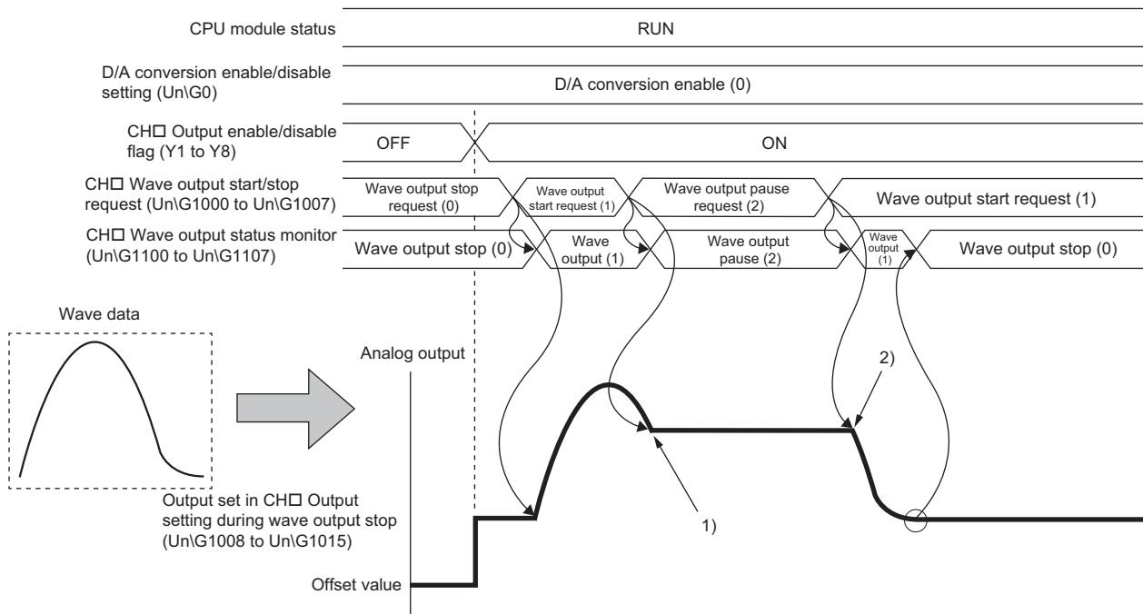
1): Wave output pauses when CH□ Wave output start/stop request (Un\G1000 to Un\G1007) is set to Wave output pause request (2) during the wave output.
