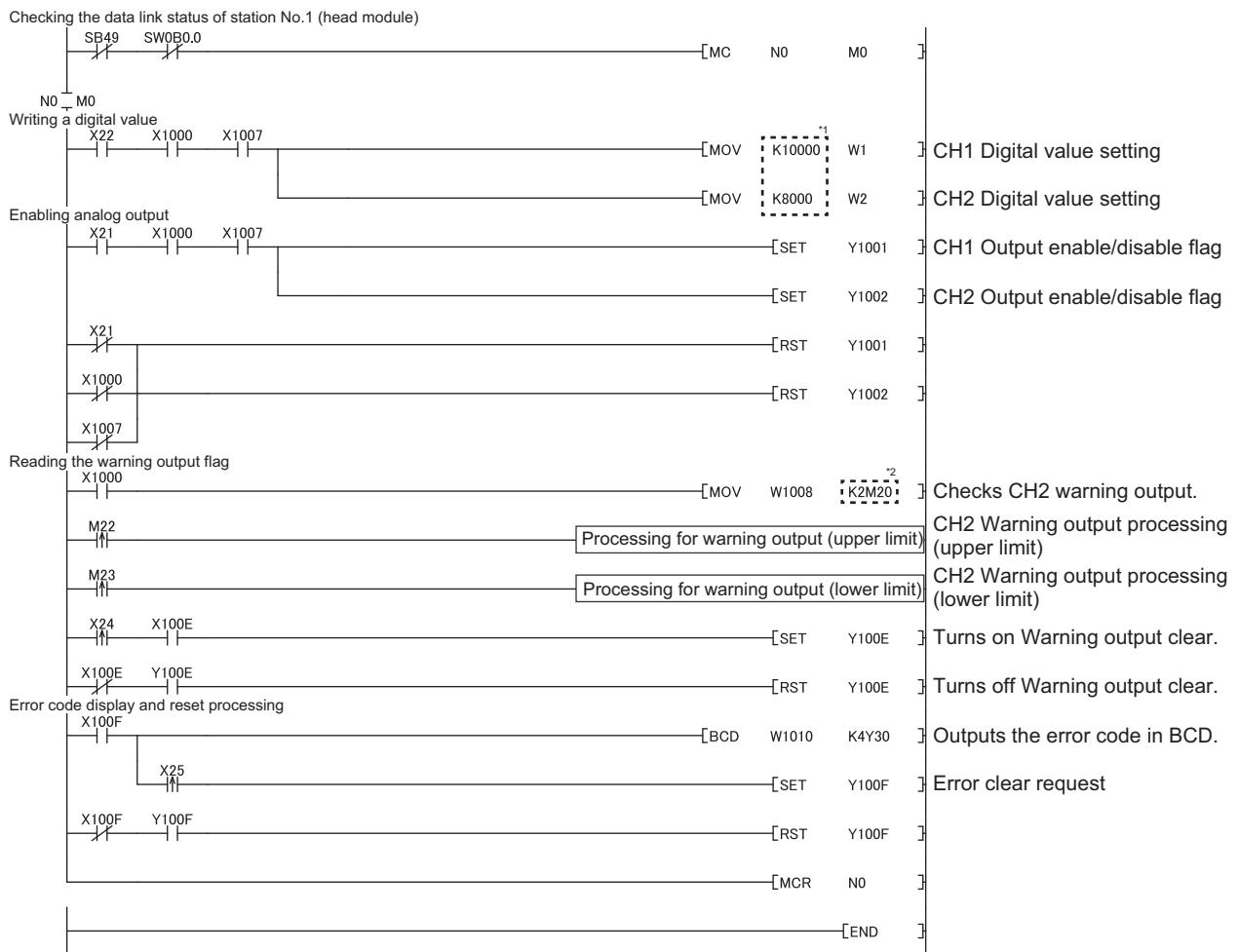
\*1 When using the L60DAVL8 or L60DAIL8, set a value according to the digital value range of the output range used.
