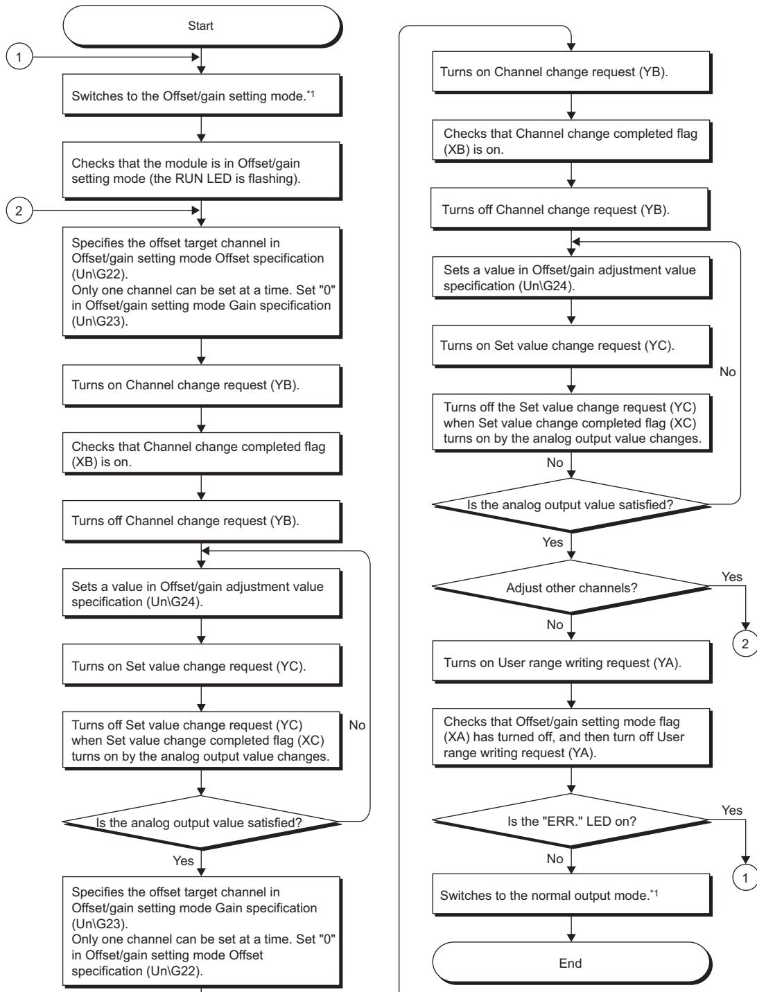
\*1 The following shows the procedure for switching the mode (normal output mode → offset/gain setting mode or offset/gain setting mode → normal output mode).
