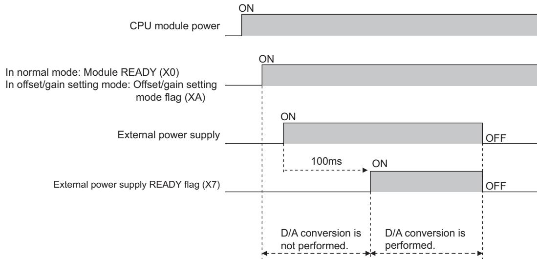
**(c) When the external power supply is turned on and off**
