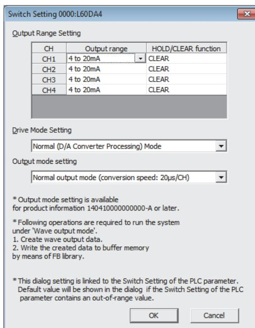
5. Display the initial setting window for the D/A converter module (L60DA4) and configure the setting as follows.
