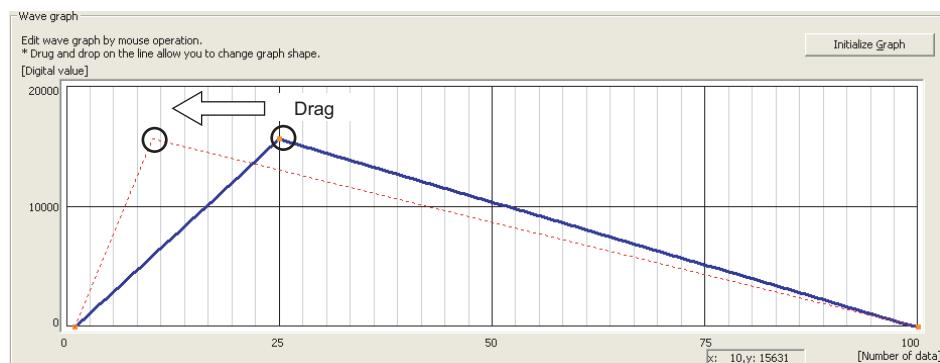
The end point position also can be adjusted by changing the value of "End point" and "Digital value" in "Wave details setting".
