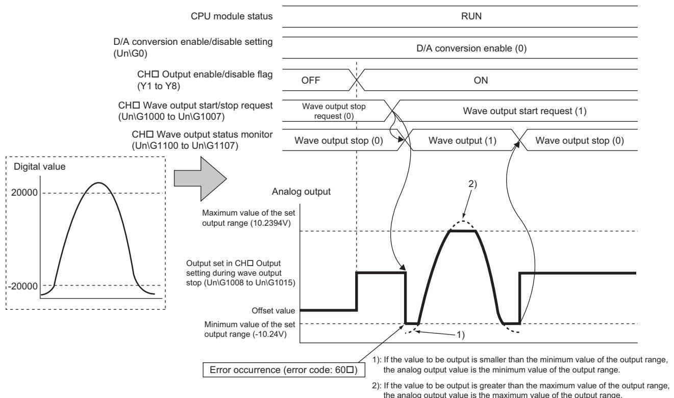
In addition, when the digital value out of the range is set and the error (error code: 60□) has occurred, correct the value to the one within the range and turn on and off Error clear request (YF).
