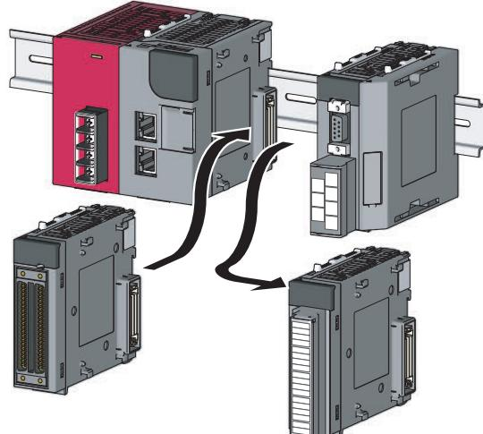
**6. Slide the modules and plug the connectors.**
