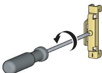
1. Pull down all DIN rail hooks on the back of the modules.
