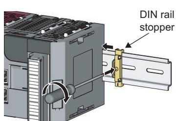
**5. Hitch the bottom hook of the DIN rail stopper to the bottom of the DIN rail.**
