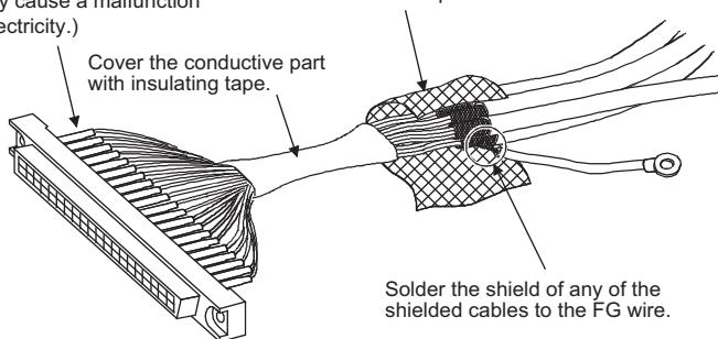
[When a duct is used (problematic example and modification example)]
