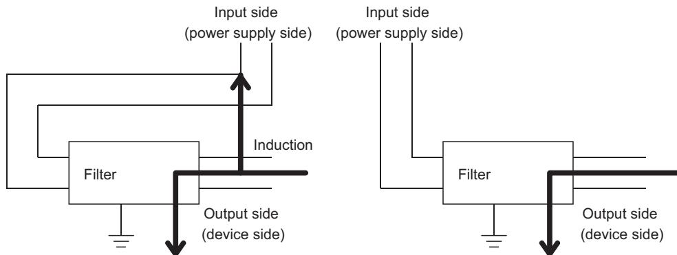
Noise will be induced when the input and output cables are bundled.
