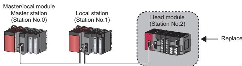
5. If the new head module does not have a station number, connect GX Works2 to the master station, and assign a station number to the head module from the CC-Link IE Field Network diagnostics.
