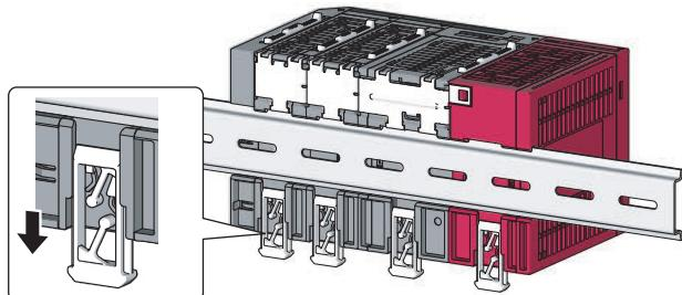
**3. Release the module joint levers on the modules.**
