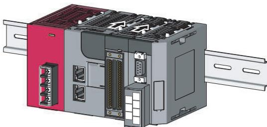
**8. Lock the DIN rail hooks and attach the DIN rail stopper.**
