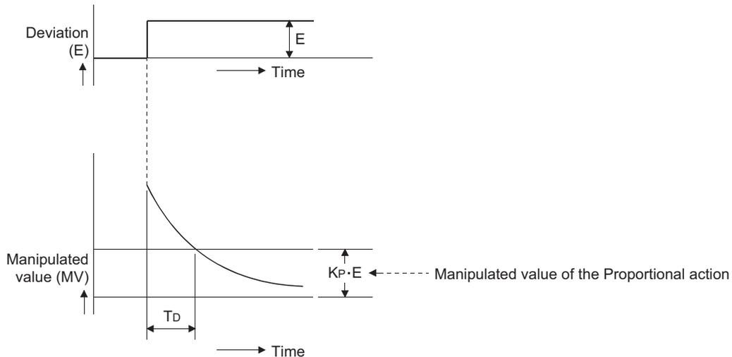
A derivative action is used as a PD action in combination with a proportional action, or PID action in combination with a proportional and integral actions.
