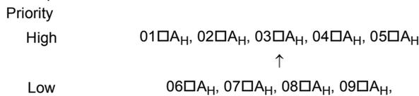
When an alarm occurs, if its priority is the same as or higher than that of alarms already occurred, the new alarm code is written over Write data error code (Un\G0).
