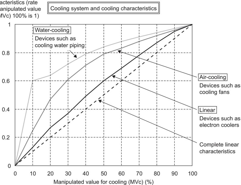
PID constants are calculated and executed based on this setting during auto tuning; therefore, more appropriate PID constants can be found by setting more applicable cooling characteristic of a device.
