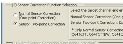
5. Select "Sensor Two-point Correction" under "Sensor Correction Function Selection".
