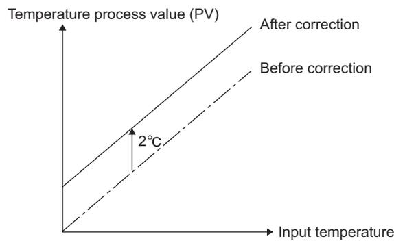
**(a) How to execute normal sensor correction (one-point correction) (when using GX Works2)**
