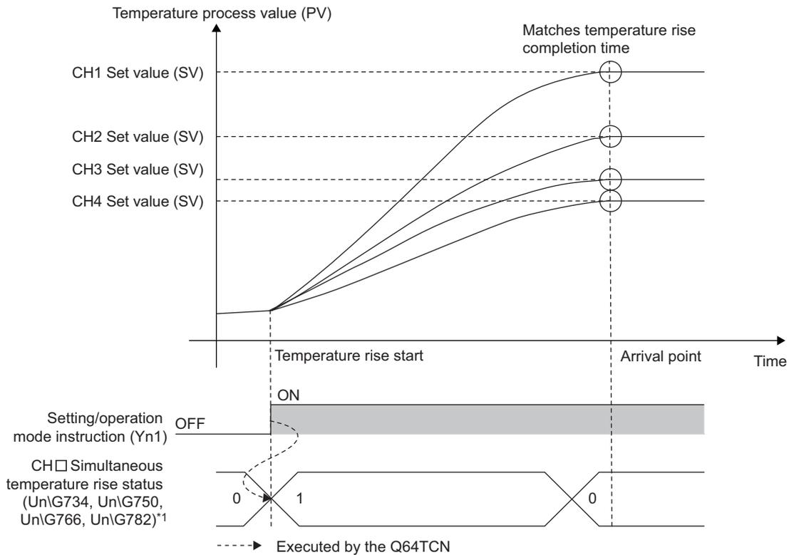
\*1 This becomes Simultaneous temperature rise in process (1) when the temperature rise starts; however, it becomes Simultaneous temperature rise not in process (0) before the temperature rise starts.
