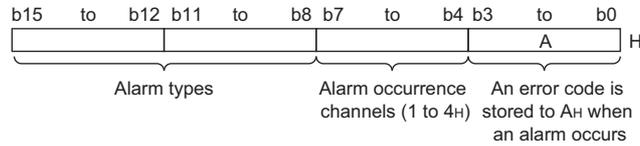
If the lower 4 bits are "0001" (1<sub>H</sub>) to "1001" (9<sub>H</sub>) or "1011" (B<sub>H</sub>) to "1111" (F<sub>H</sub>), an error occurs. When an error occurs, refer to the error code list (Page 373, Section 8.6).
