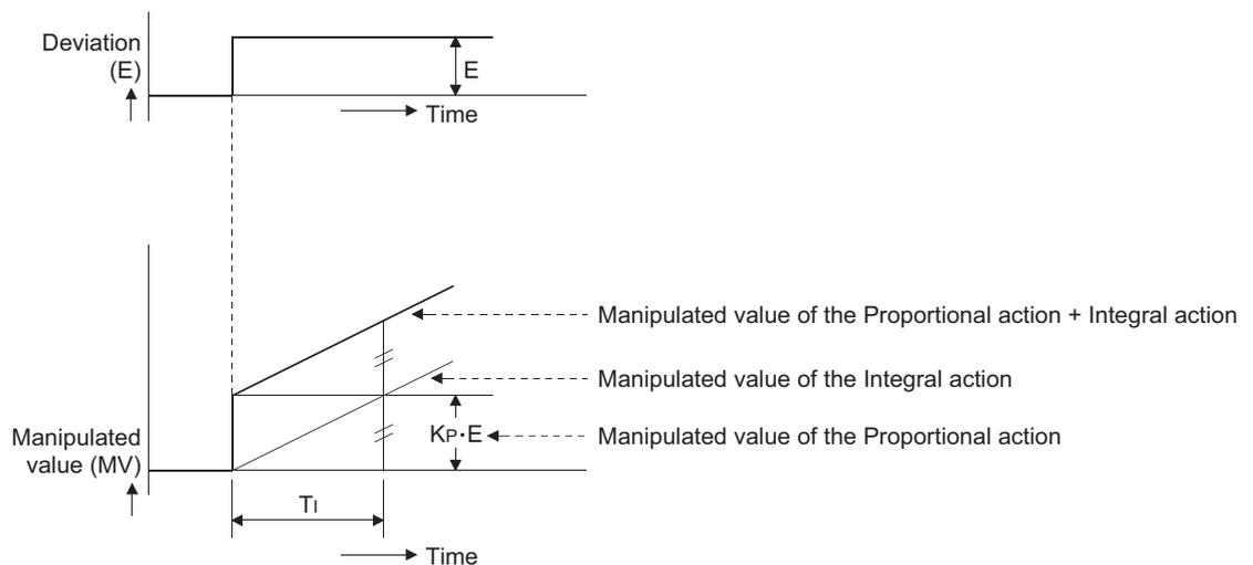
An integral action is used as a PI action in combination with a proportional action, or PID action in combination with a proportional and derivative actions.
