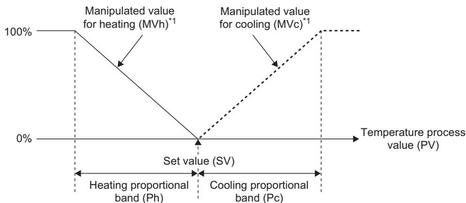
\*1 The actual output value is restricted within the output limiter range set in CH□ Heating upper limit output limiter (Un\G42, Un\G74, Un\G106, Un\G138) and CH□ Cooling upper limit output limiter (Un\G721, Un\G737, Un\G753, Un\G769). (☞ Page 112, Section 3.4.2 (19))
