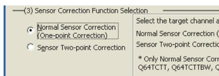
5. Select "Normal Sensor Correction (One-point Correction)" under "Sensor Correction Function Selection".
