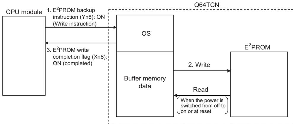
If data write to E<sup>2</sup>PROM does not complete, E<sup>2</sup>PROM write failure flag (XnA) turns on.
