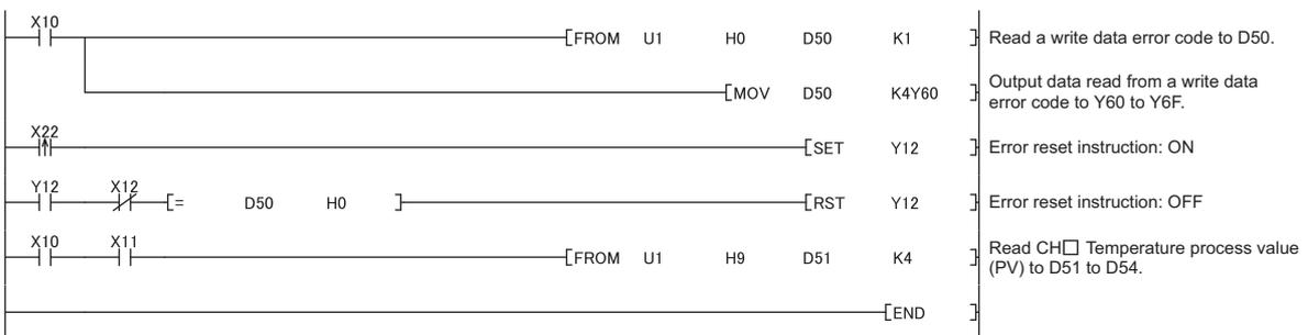
**(c) Program example where the simultaneous temperature rise function is used**
