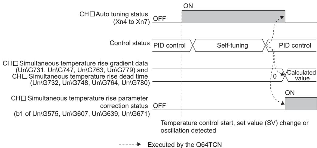
**(b) Condition for the simultaneous temperature rise parameter setting using self-tuning**
