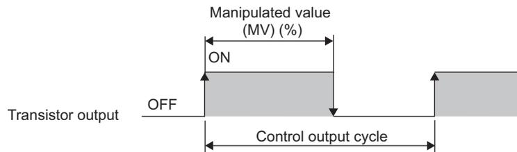
The ON time of the control output cycle is determined by multiplying the control output cycle by the manipulated value (MV)<sup>\*1</sup> (%). If the manipulated value (MV)<sup>\*1</sup> is constant, a pulse of the same cycle is output repeatedly.
