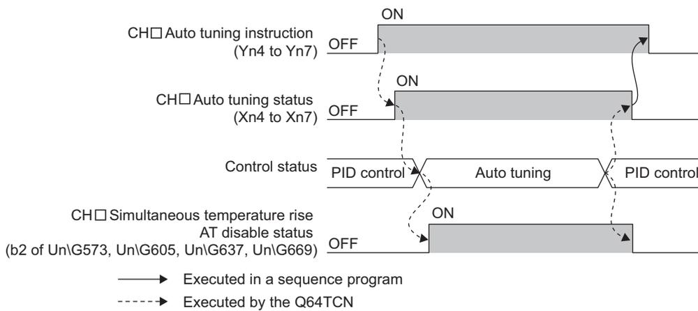
The Q64TCN turns CH□ Simultaneous temperature rise AT disable status (b2 of Un\G573, Un\G605, Un\G637, Un\G669) to 1 (ON). With CH□ Auto tuning status (Xn4 to Xn7) on, the module performs the same processing as normal auto tuning.
