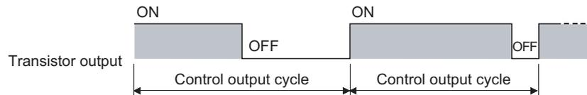
The manipulated value (MV) represents the ON time of the control output cycle in percentage. (☞ Page 91, Section 3.4.2 (5))
