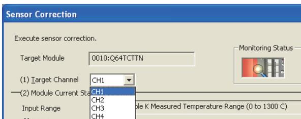
4. Select the channel where sensor correction is executed under "Target Channel".
