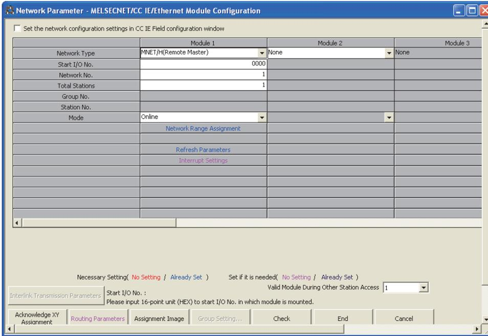
**3. Display the network range assignment setting window and configure the setting as follows.**
