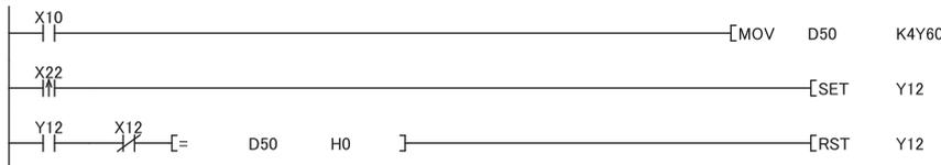
} Output a write data error code to Y60 to Y6F.
