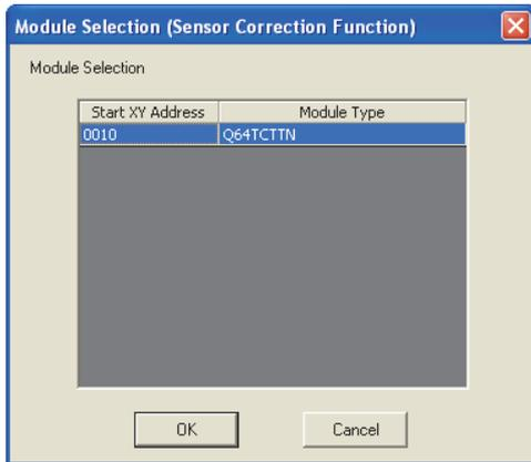
1. Select the module where sensor correction is executed and click
