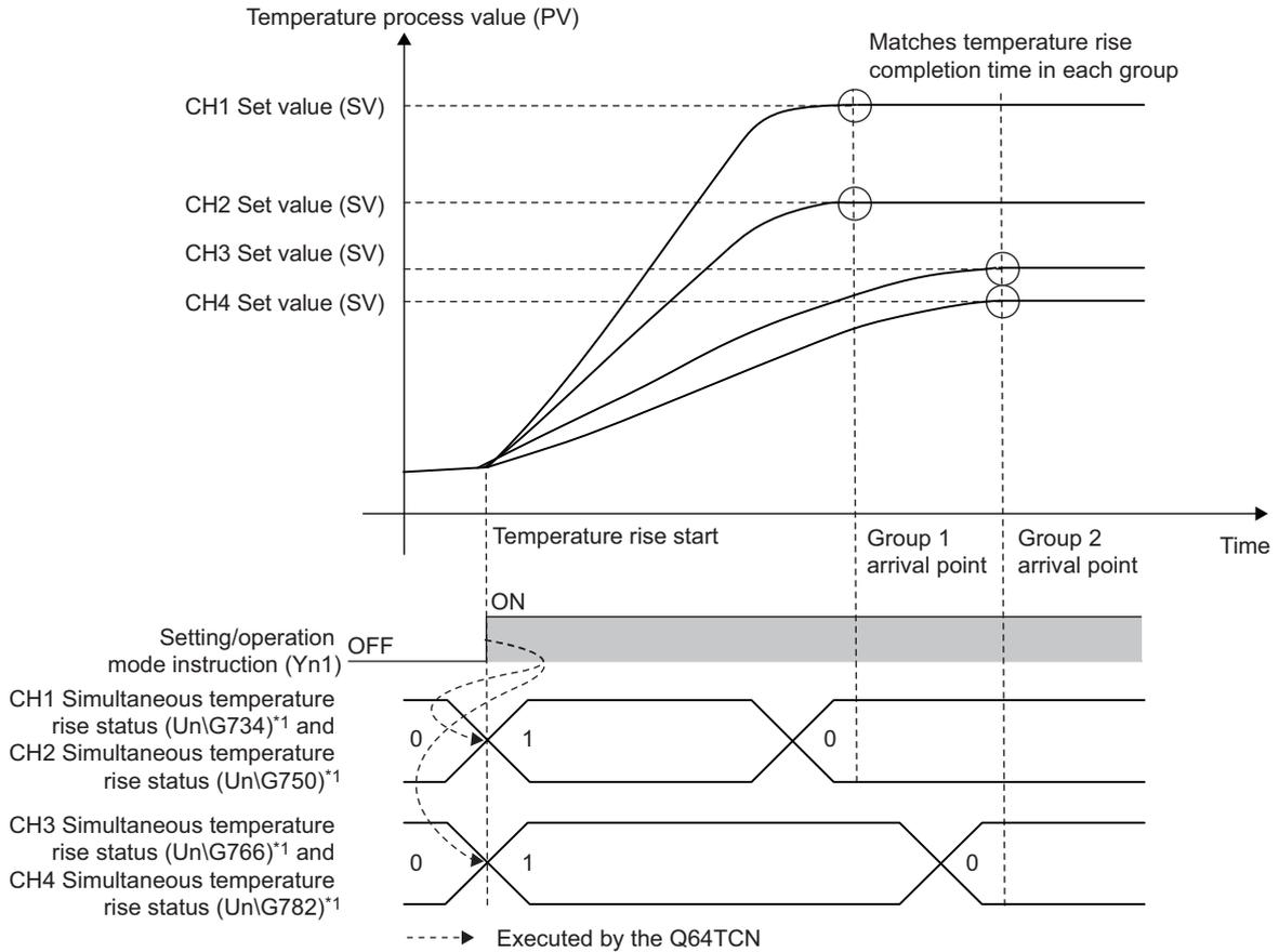
\*1 They become Simultaneous temperature rise in process (1) when the temperature rise starts; however, they become Simultaneous temperature rise not in process (0) before the temperature rise starts.
