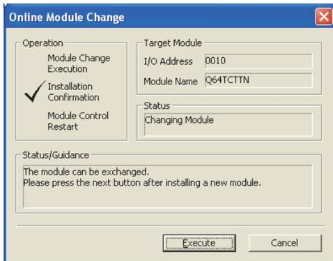
1. Mount a new module in the same slot and connect the external cable.
