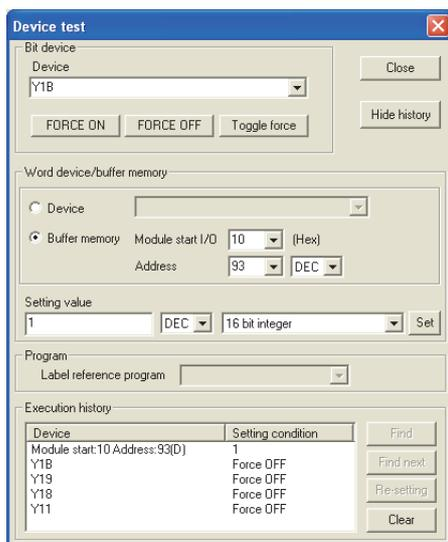
4. Set the data pre-recorded in the device test to the buffer memory.
