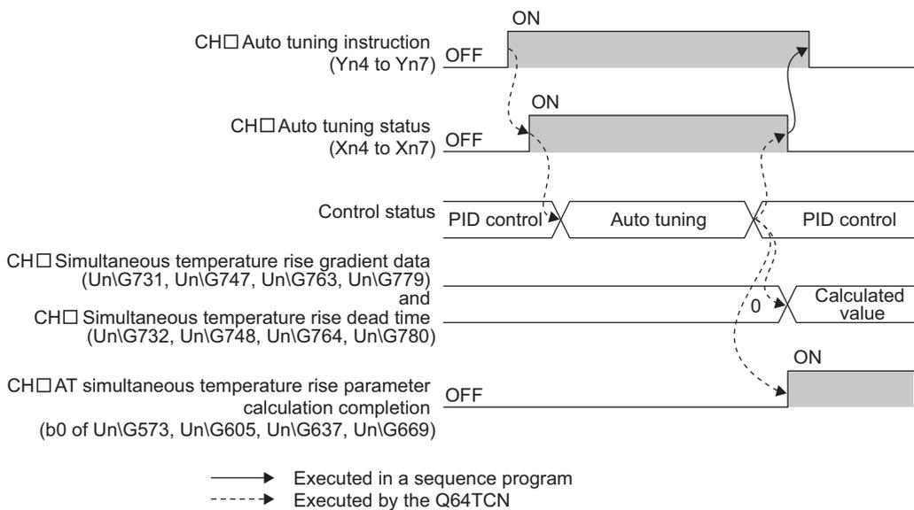
**(c) Condition for the simultaneous temperature rise AT**
