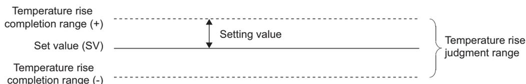
When CH□ Temperature process value (PV) (Un\G9 to Un\G12) enters the temperature rise judgment range, CH□ Temperature rise judgment flag (Un\G17 to Un\G20) is set to Within temperature rise completion range (1). (Set the time from the temperature rise completion to Within temperature rise completion range (1) in Temperature rise completion soak time setting (Un\G168).)
