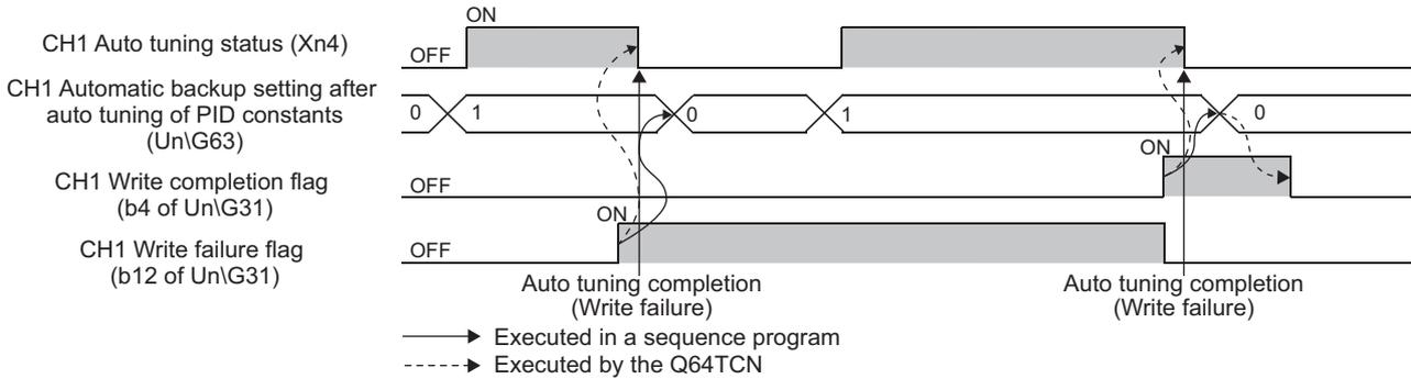
When the data writing to E<sup>2</sup>PROM is completed normally, CH□ Write completion flag (b4 to b7 of Un\G31) turns on.
