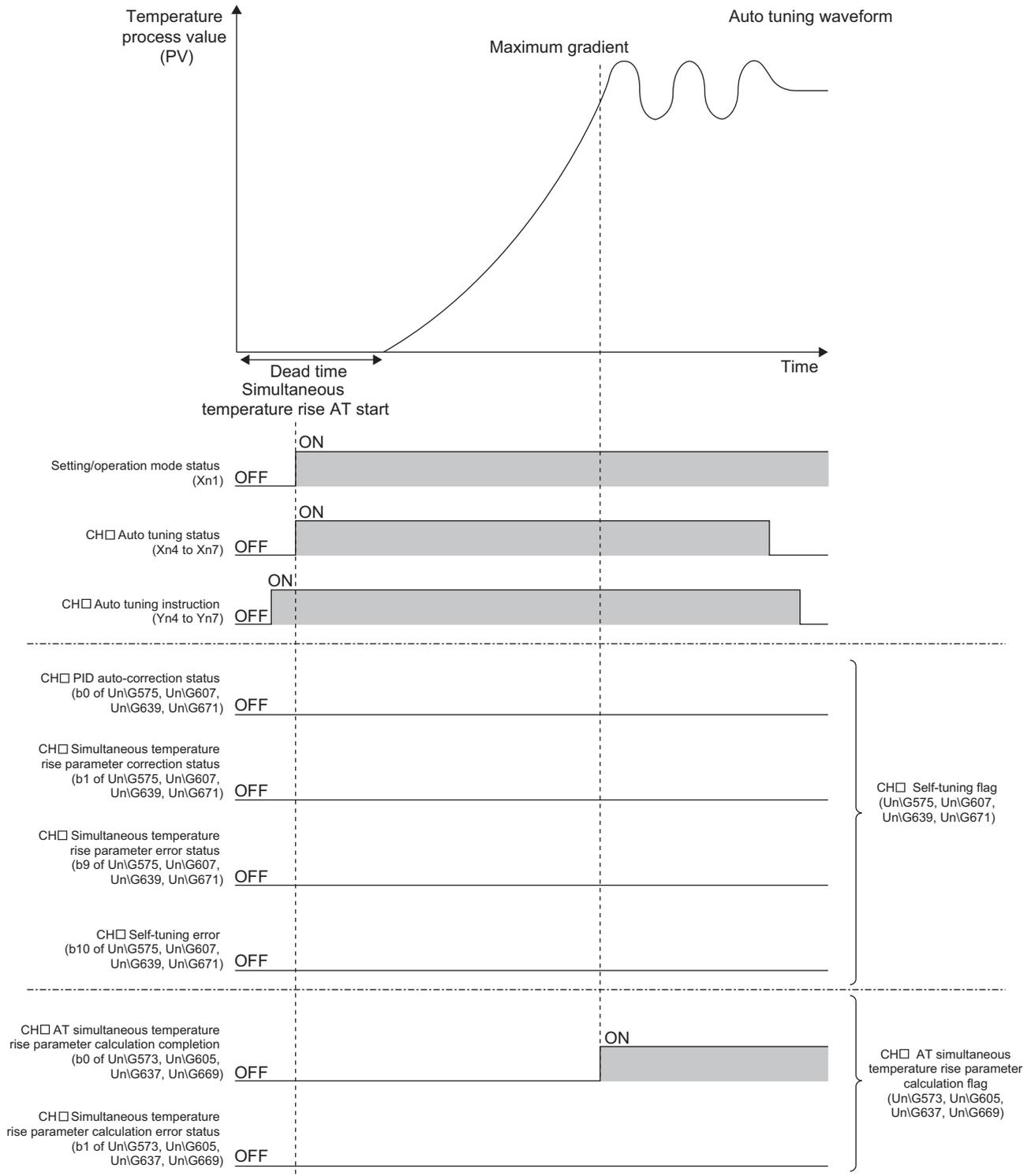
**(d) When auto tuning is started with the temperature process value (PV) within the stable judgment width (1°C (°F)) after the setting mode is changed to the operation mode**
