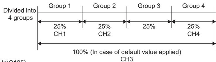
Whether the transistor output is executed or not can be selected by CH3 Unused channel setting (UnG125).
