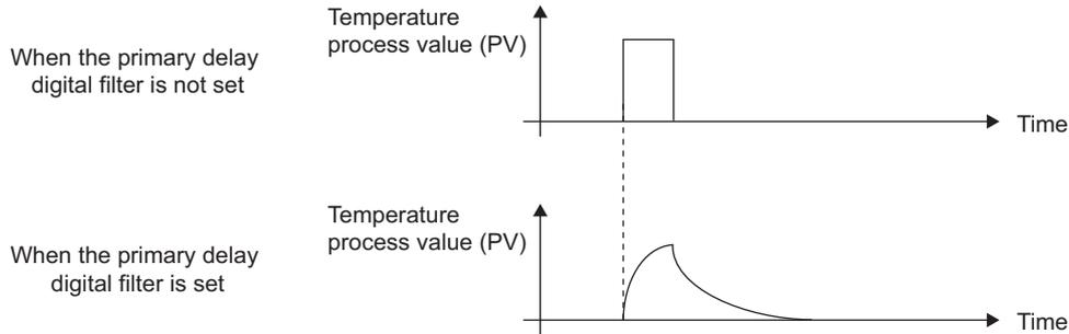
The time for the temperature process value (PV) to change by 63.3% can be set by the primary delay digital filter setting (filter setting time).
