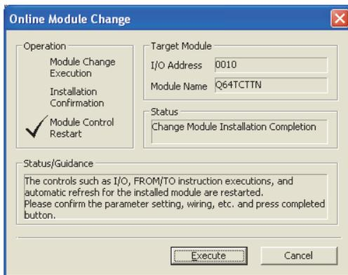
3. When the window appears, click to restart the control. Module READY flag (Xn0) turns on.
