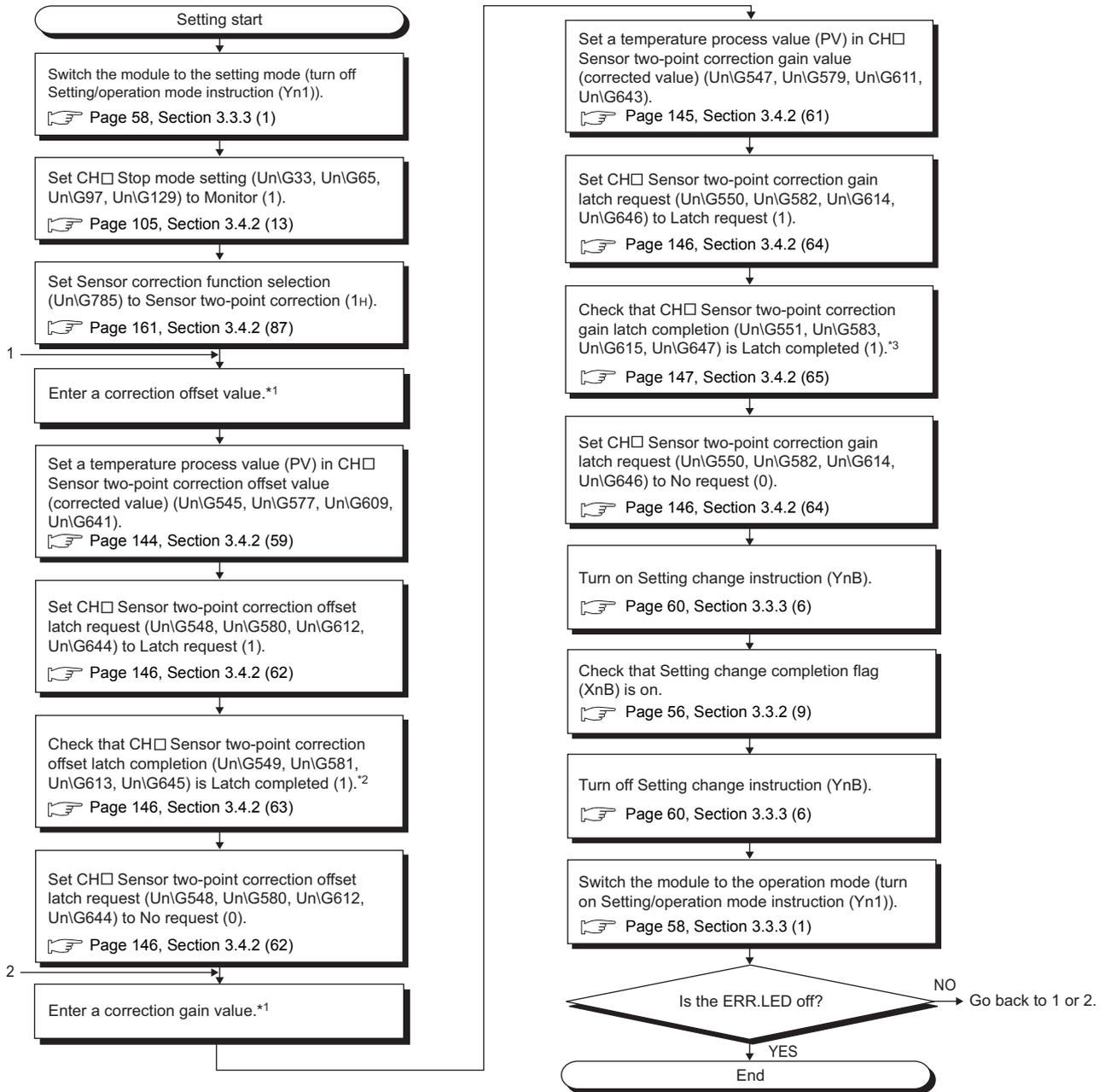
\*1 Enter the value using devices such as a thermocouple, platinum resistance thermometer, and standard DC voltage generator, or based on a general resistance value.
