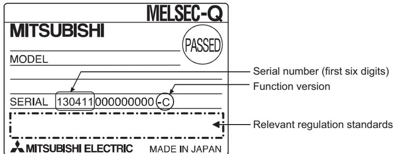
**(2) Checking on the front part (bottom part) of module**
