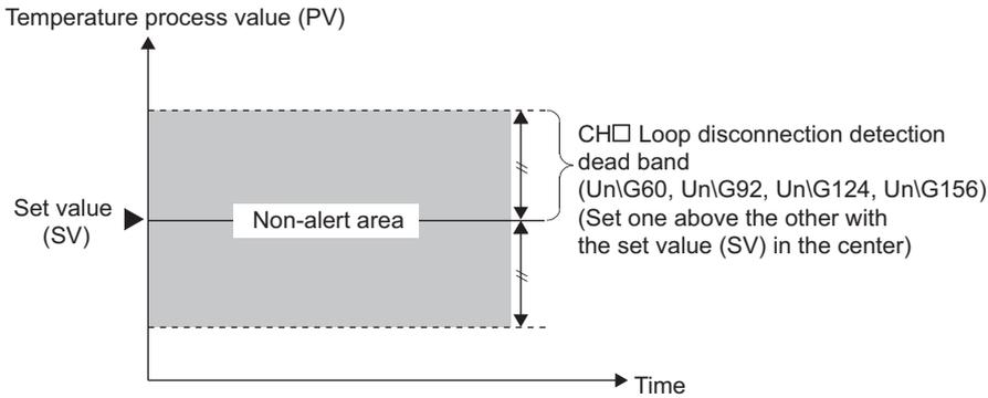
For details on the loop disconnection detection function, refer to the following.
