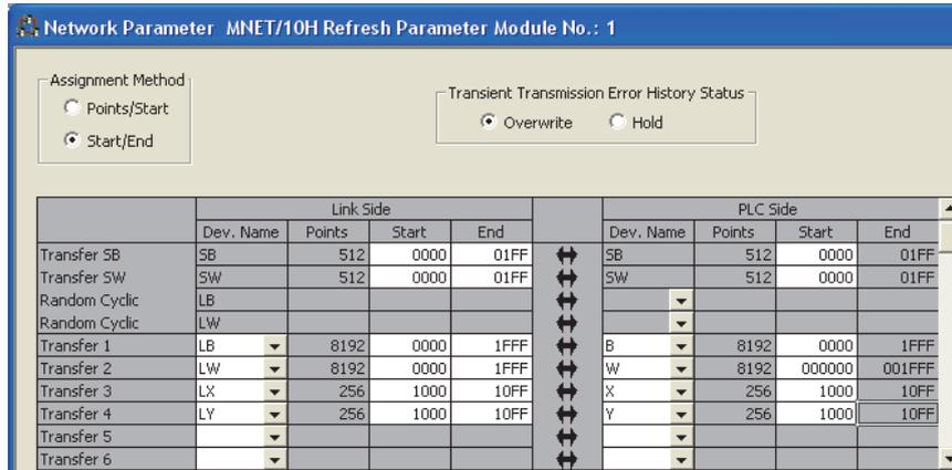
**5. Write the set parameter to the CPU module on the master station. Then reset the CPU module or turn off and on the power supply of the programmable controller.**
