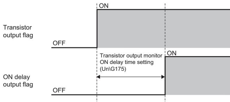
Transistor output monitor ON delay time setting (Un\G175) enables setting considering delay time (response/scan time delay) of actual transistor output. (Page 134, Section 3.4.2 (45))
