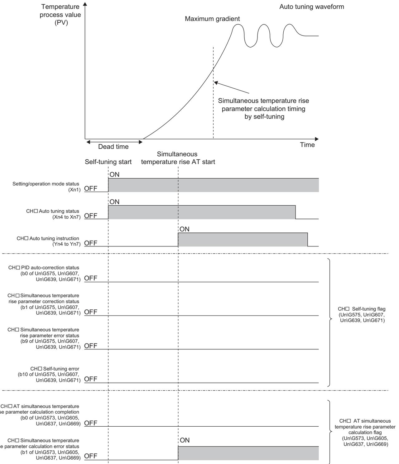
**(b) When the simultaneous temperature rise AT is started after the simultaneous temperature rise parameter is calculated with self-tuning**
