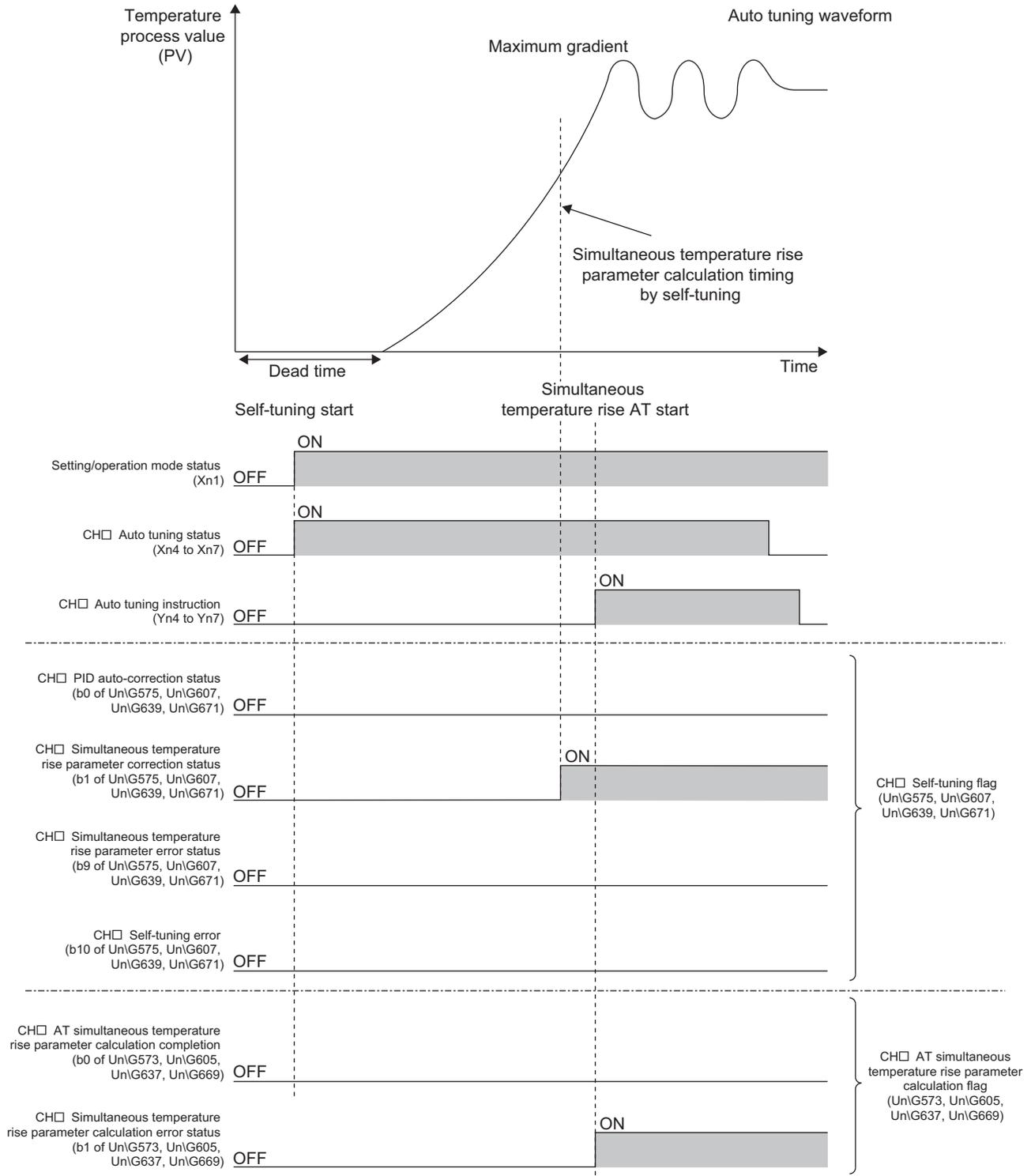
**(c) When CH□ Auto tuning instruction (Yn4 to Yn7) is turned off and on in the setting mode and the module is shifted to the operation mode**
