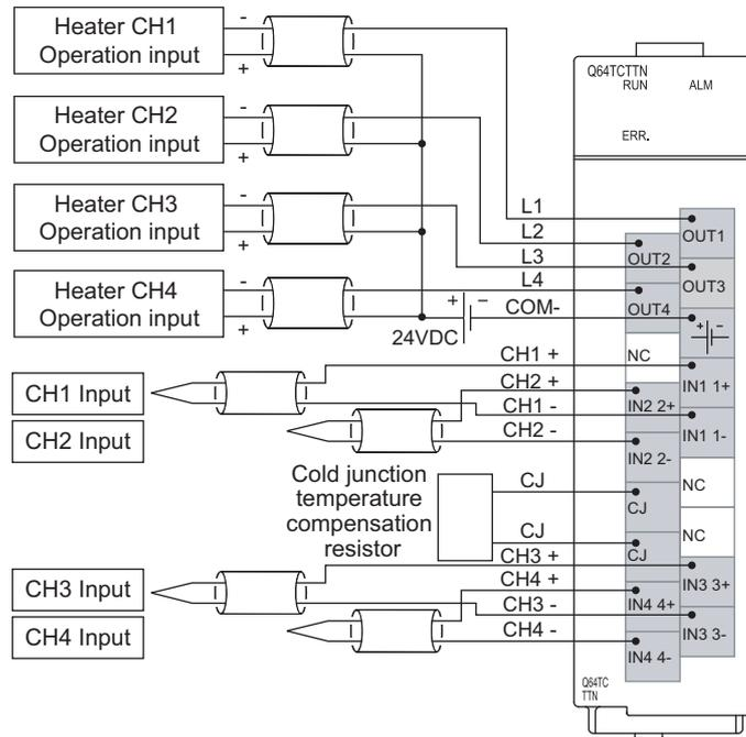
7.2 When Using the Module in a Standard System Configuration
