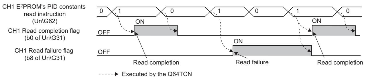
When the data reading from E<sup>2</sup>PROM is completed normally, CH□ Read completion flag (b0 to b3 of Un\G31) of the corresponding channel turns on.
