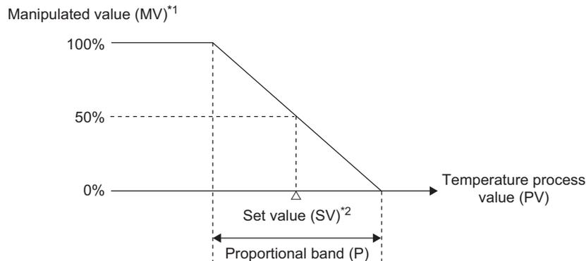
\*1 The actual output value is restricted within the output limiter range set in CH□ Upper limit output limiter (Un\G42, Un\G74, Un\G106, Un\G138) and CH□ Lower limit output limiter (Un\G43, Un\G75, Un\G107, Un\G139). (☞ Page 112, Section 3.4.2 (19))
