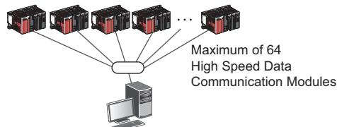
A diagram showing a server personal computer connected to 64 High Speed Data Communication Modules. The server is at the bottom, and 64 modules are arranged in a grid above it, connected by lines. An ellipsis indicates that there are more modules. |
