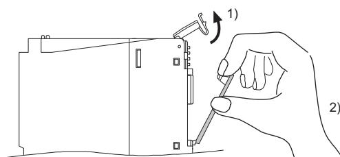
1) Put your finger on the bottom of the LED cover on the front of the module and lift the LED cover up to open.
