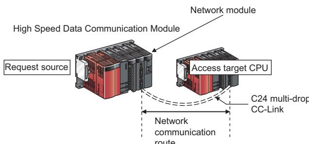
The following shows the CPU modules that can be accessed on the network communication routes.
