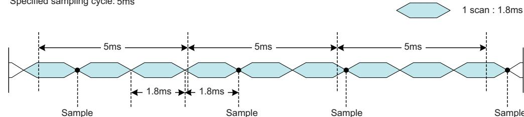
When a sequence scan time is longer than a specified sampling cycle, data are sampled in a sequence scan time.\*1 Device data are sampled even when the access target CPU is in a STOP status.
