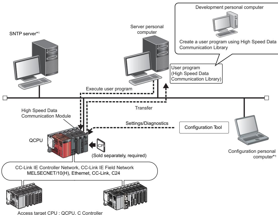
\*1 Required when synchronizing High Speed Data Communication Module and CPU module time to a standard time.
