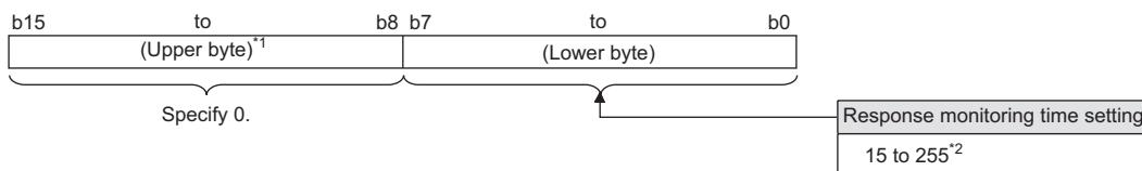
\*1 Basically, the information of upper byte is ignored, however, when upper byte is other than 0, the switch setting error (0180H) occurs at hardware test.
