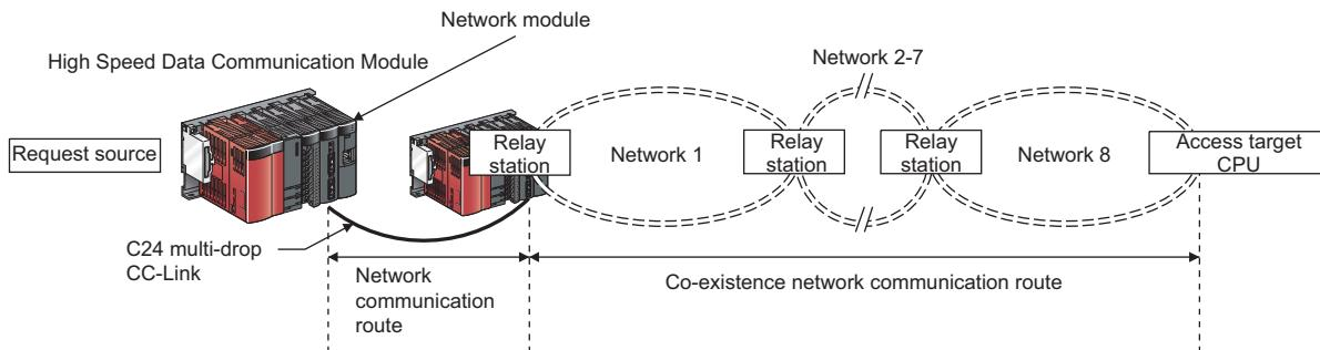
The following shows the CPU modules that can be accessed on the network communication routes and co-existence network communication routes.
