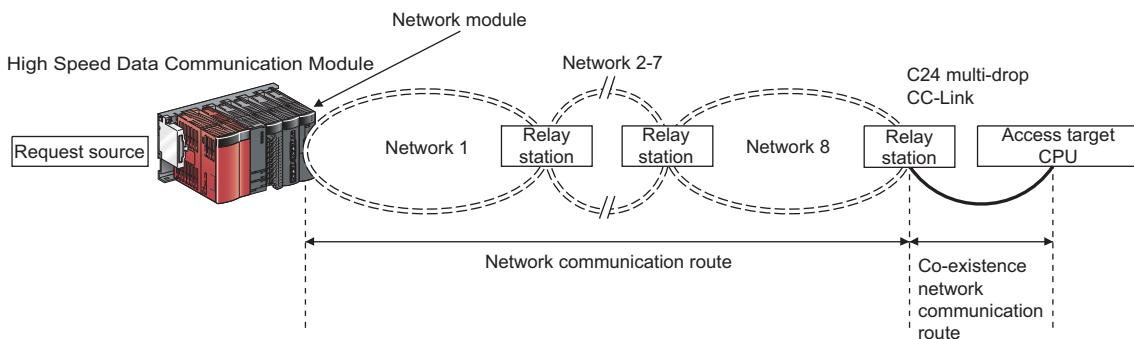
The following shows the CPU modules that can be accessed on the network communication routes and co-existence network communication routes.
