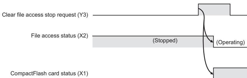
**■When using Configuration Tool (☞ Page 188 Diagnosing the CompactFlash card)****Operating procedure****1. Clearing the file access stop status.**
