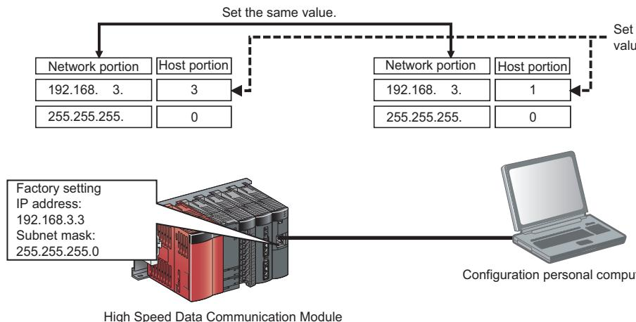
2. Make the network settings for the personal computer on the "Internet Protocol (TCP/IP) Properties" screen.
