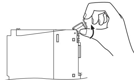
2. Eject the CompactFlash card.
