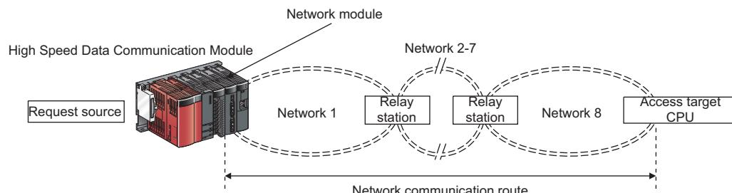
The following shows the CPU modules that can be accessed on the network communication routes.
