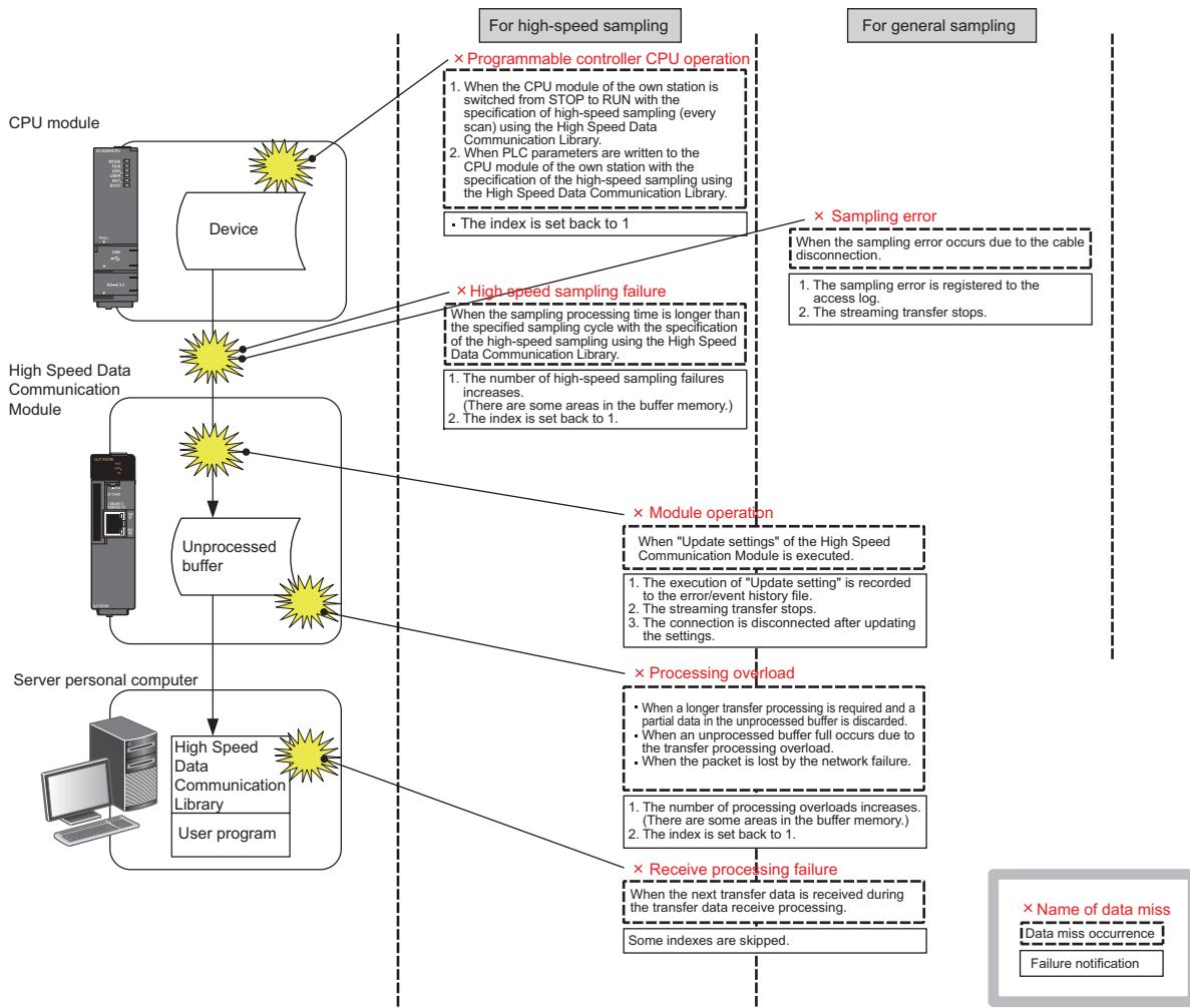
The processing overload counts are not increased when the transfer data is being buffered.
