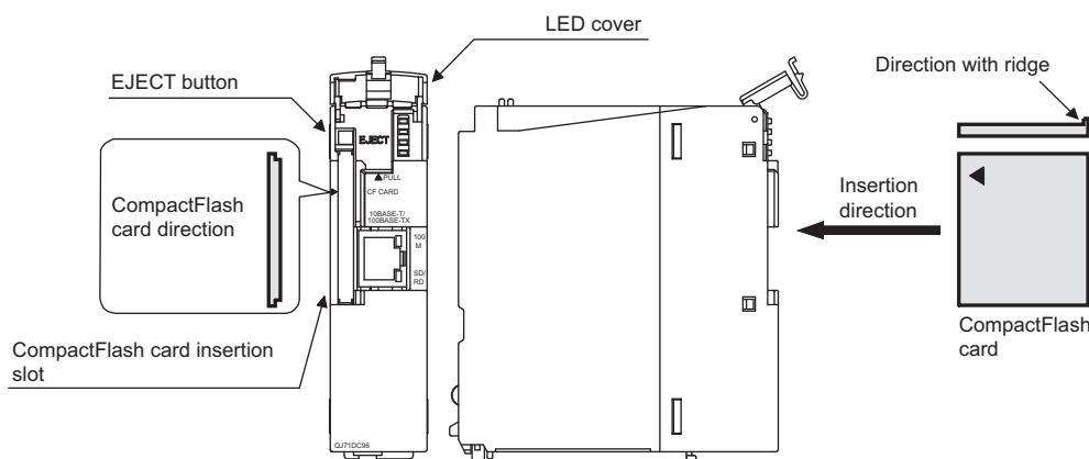
**3. Lower the LED cover on the front of the High Speed Data Communication Module until it clicks.****Restriction**
