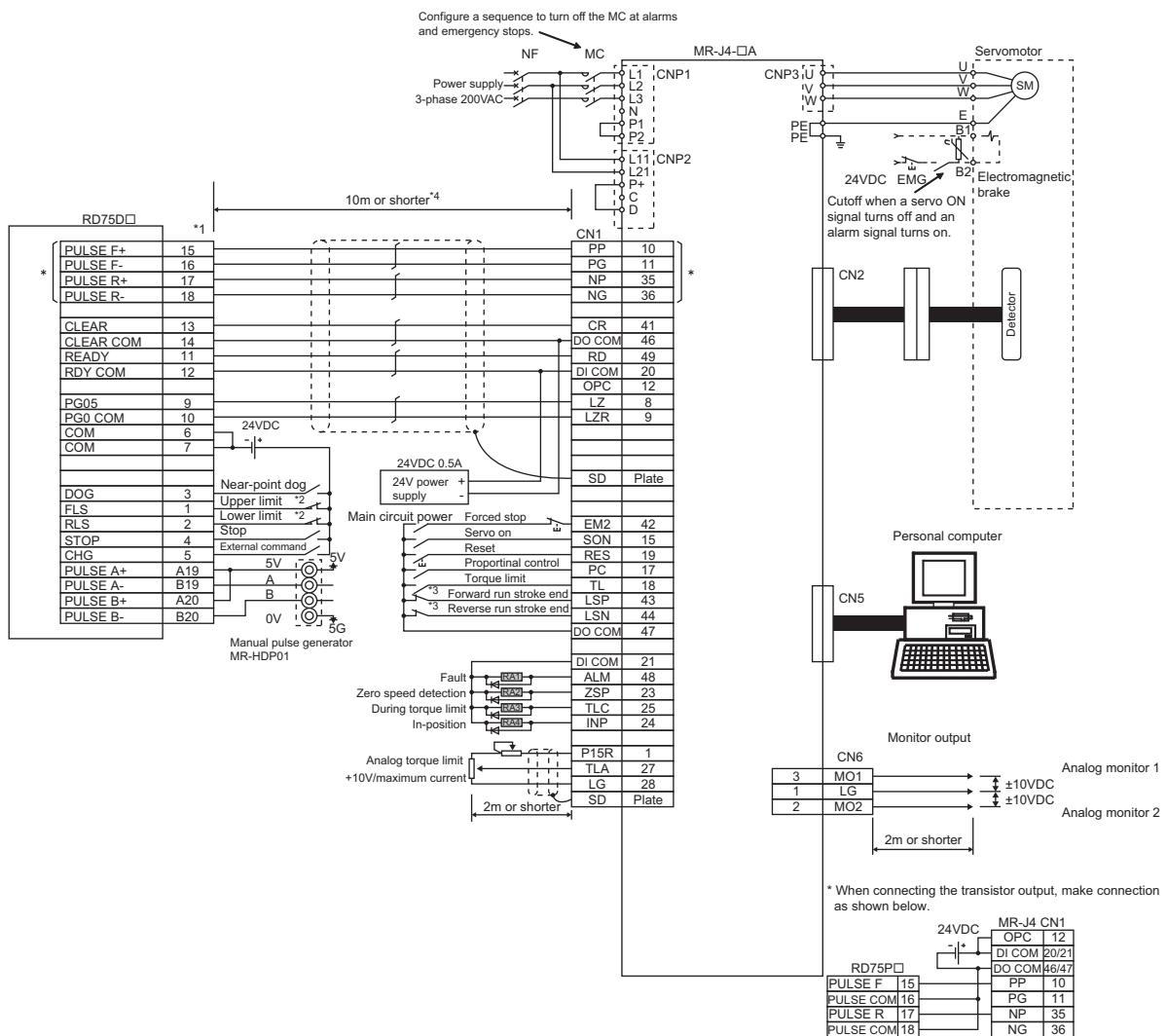
\*1 The logic of each I/O terminal can be changed with [Pr.22] Input signal logic selection and [Pr.23] Output signal logic selection of detailed parameter 1. (The negative logic is set for all terminals in the above example.)
