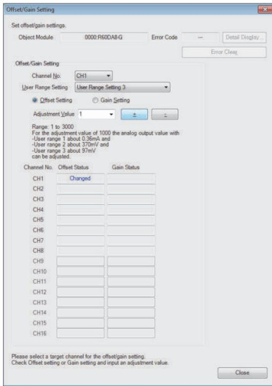
6. The adjustment amount of the offset value or gain value has to be selected from "1", "100", "500", "1000", "2000", and "3000" first; however, further fine adjustments are possible by entering a desired value (1 to 3000).
