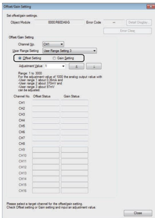
5. Specify whether to configure the offset setting or gain setting with the radio button. (The steps from step 6 assume that the offset setting is specified.)
