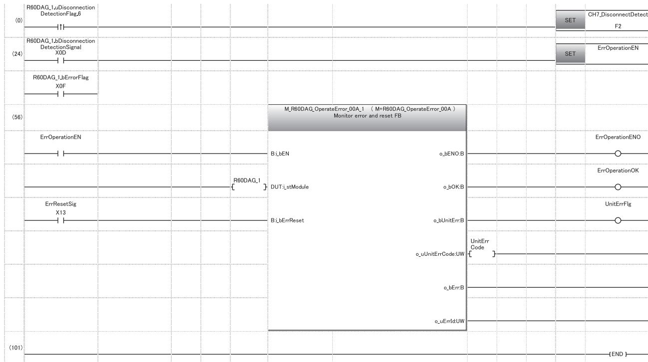
(0) The processing at the time when a disconnection is detected is to be performed.
