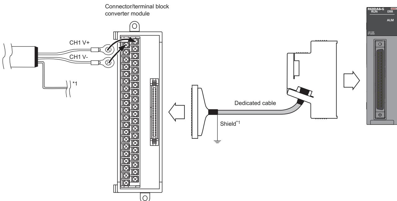
\*1 Be sure to use a shielded cable. The shield must be grounded.
