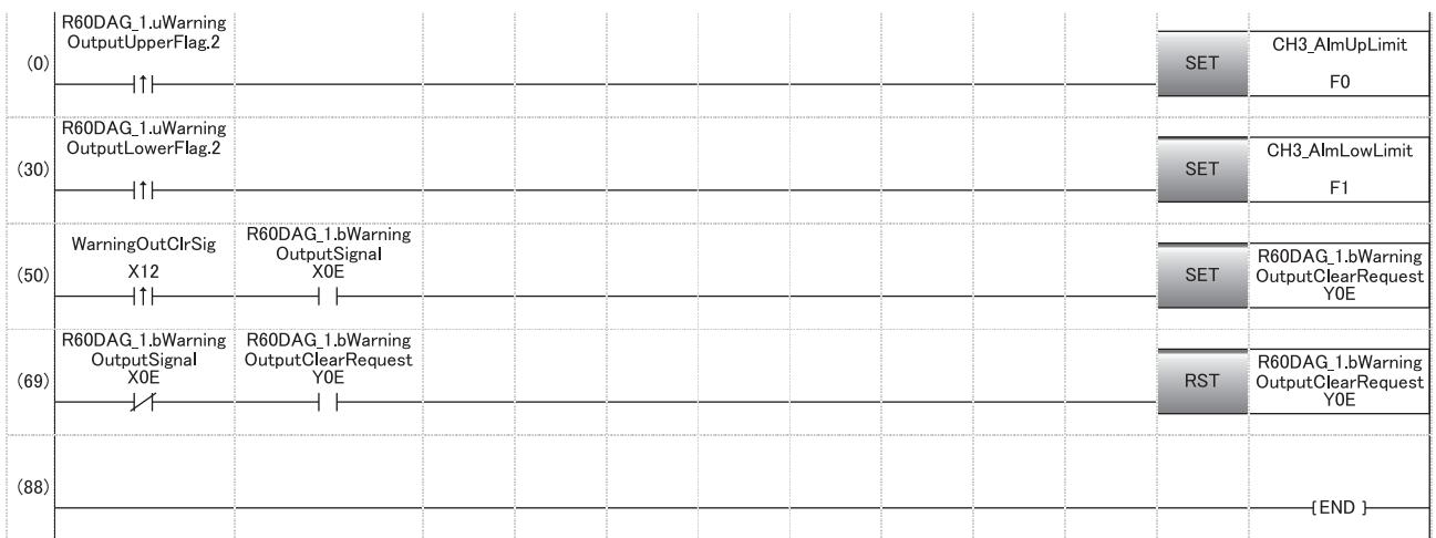
(0) The processing at the time when an upper limit alert is issued in CH3 is to be performed.
