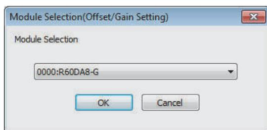
2. Select the target module for the offset/gain setting, and click the [OK] button.
