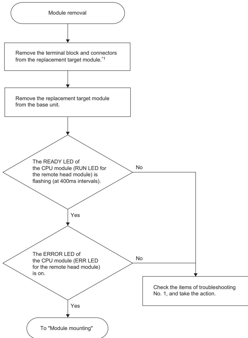
\*1 Remove the SD memory card from the module to be replaced when MES interface module, high speed data logger module, C intelligent function module, and OPC UA server module are used.
