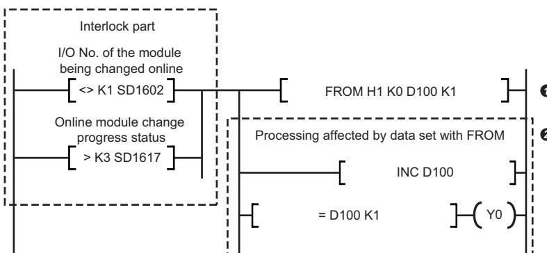
① Establishing the following two conditions results in the stop of the FROM instruction given to the module whose start I/O number is 0010H:
