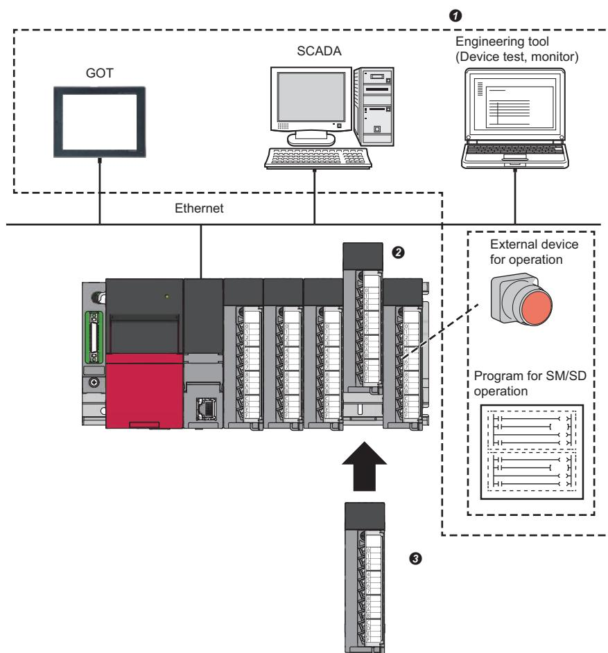
**①** Operate special relays and special registers from an engineering tool, a GOT, or an external device for operation.
