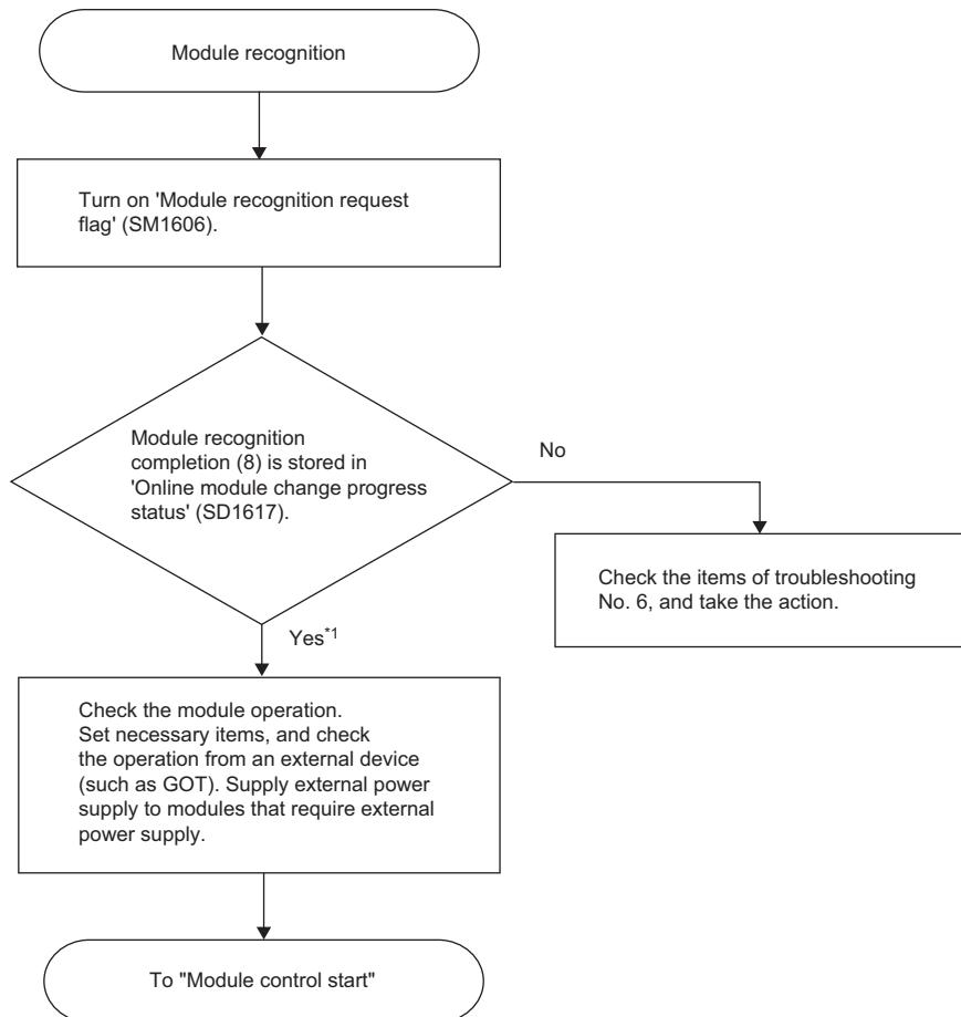
\*1 When the initial setting is configured with the module parameter of an engineering tool, the setting of the module parameter is applied when the RUN LED turns on.
