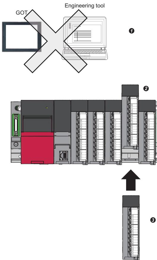
① Do not operate special relays or special registers.
