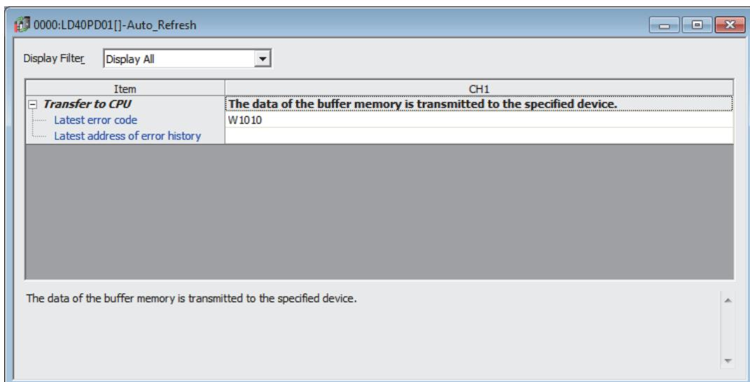
7. Write the set parameters to the head module. Then reset the head module or power off and on the programmable controller.
