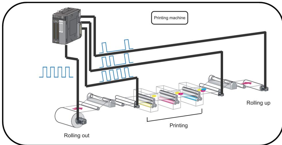
The ratio ( $x/y$ ) used in ratio conversion must be " $y \geq x$ " when a signal multiplied by  $x/y$  is output to an input signal. Conversions with the ratio exceeding one time cannot be performed.
