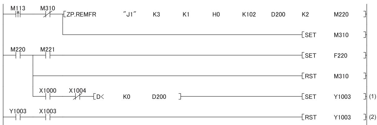
(1) Turn on Operating condition settings batch-reset command (Y1003).
