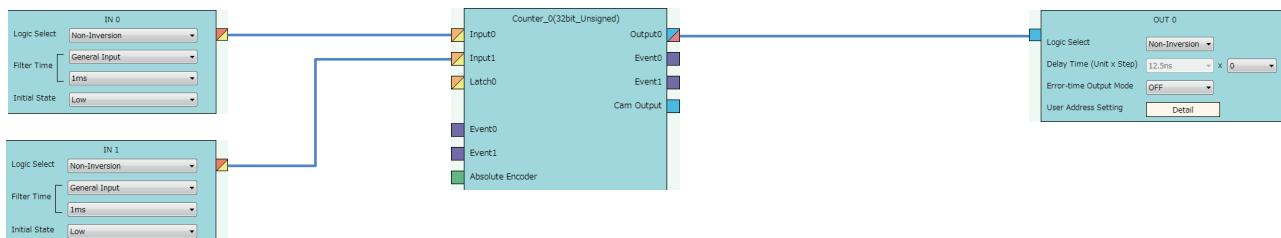
2. Set the external input blocks according to the specifications of external input signals.
