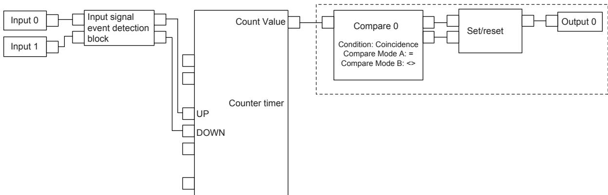
Create the hardware logic by using compare blocks and a set/reset block, as shown in the dotted line frame.
