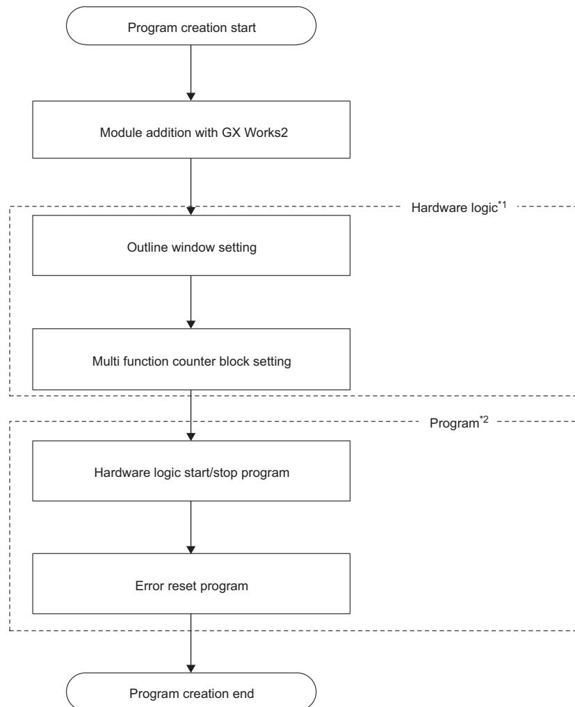
\*1 Set the hardware logic with the configuration tool.
