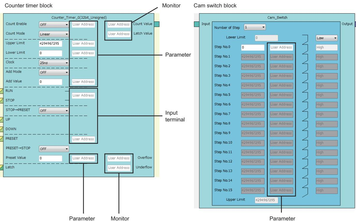
The application varies according to targets to which "User Address" is assigned.
