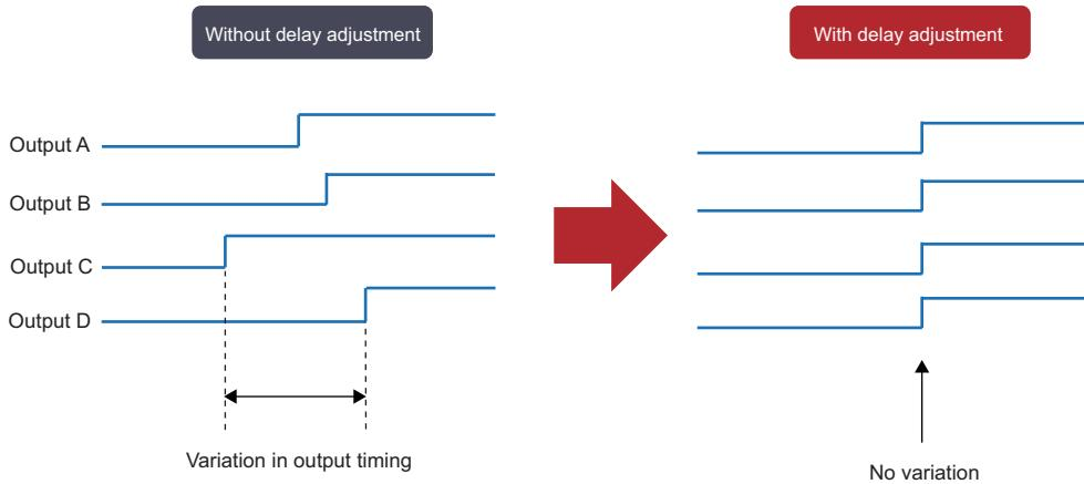
The timing variation due to electronic components can be adjusted.
