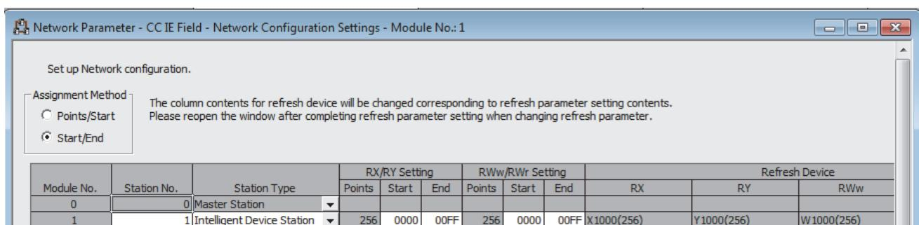
4. Display the setting window for the refresh parameters and set the values as follows.
