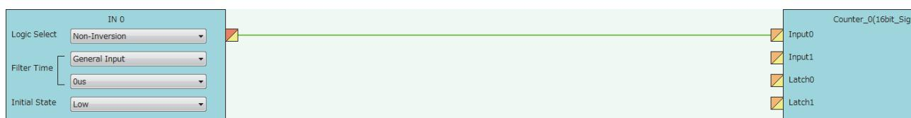
2. Right-click the link and select "Wiring Delete" from the context menu. Or press the **Deleted** key.
