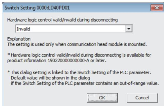
When the own station is disconnected, the operations of the flexible high-speed I/O control module differ depending on the setting of "Hardware logic control valid/invalid during disconnecting" in the switch setting or that of "Error Time Output Mode" in the intelligent function module detailed setting. For details, refer to the following.
