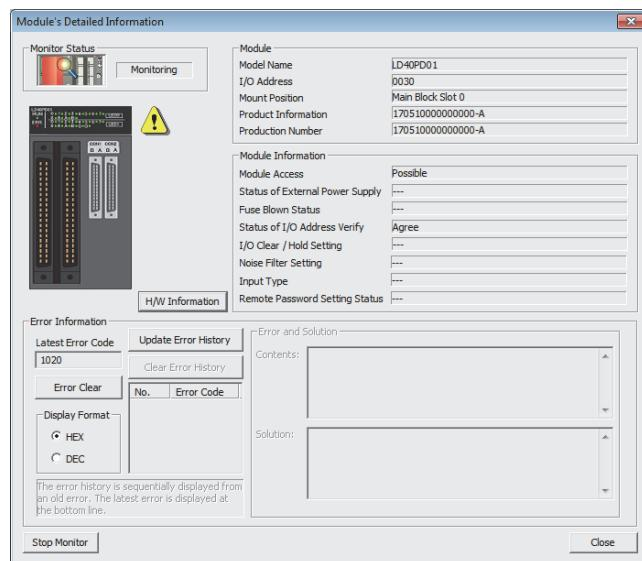
2. The "Module's Detailed Information" window of the flexible high-speed I/O control module is displayed.
