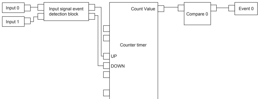
The multi function counter block\_0 counts external input signals. When the count value becomes equal to the compare value, an event signal is output to the multi function counter block\_1.
