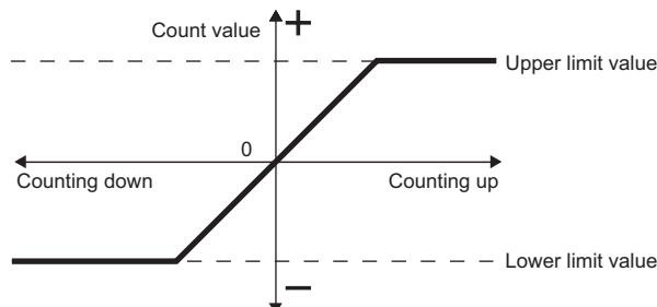
If "Count Value" has reached the upper limit value in up count, "Count Value" does not change in the next up count and the overflow error (error code: 100□H) occurs. "Count Value" does not change until the preset function is performed even if down count is performed.
