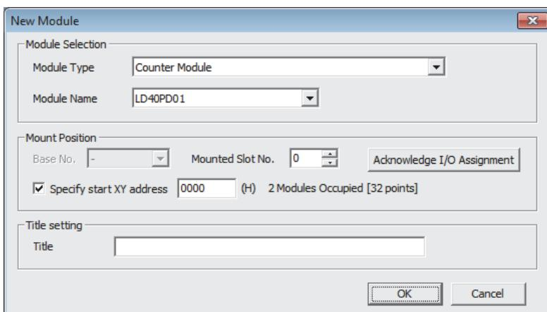
4. Display the setting window for the intelligent function module detailed setting of the flexible high-speed I/O control module (LD40PD01) and set the values as follows.
