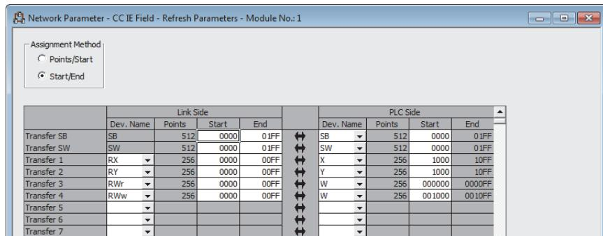
5. Write the set parameters to the CPU module on the master station. Then reset the CPU module or power off and on the programmable controller.
