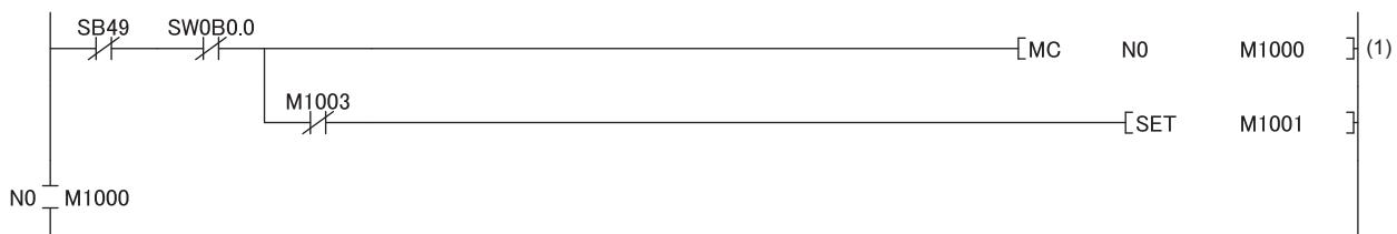
(1) Check the data link status of the head module (station number 1).
