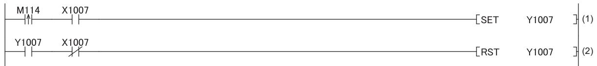
(1) Turn on Hardware logic control stop flag clear request at disconnection (Y1007).
