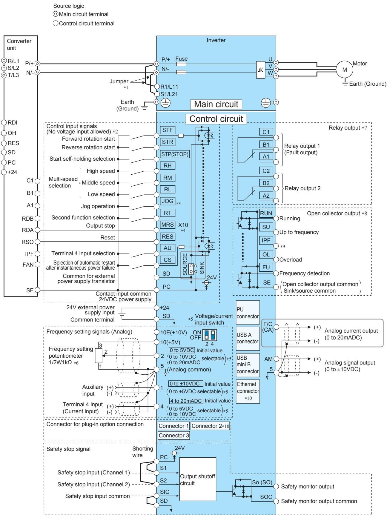
\*1 A jumper is installed across terminal R1/L11 and terminal P/+, and across terminal S1/L21 and terminal N/-. When using a separate power supply for the control circuit, remove the jumpers connected to terminals R1/L11 and S1/L21.
