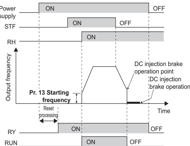
■ **Checking the motor operating status by using the start signal input to the inverter and the Output current detection signal output from the inverter ... (d)**
