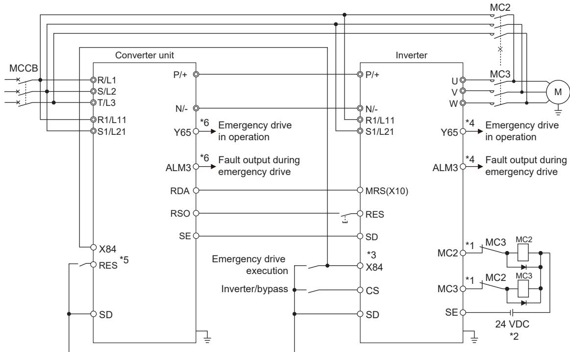
\*1 Be careful of the capacity of the sequence output terminals.
