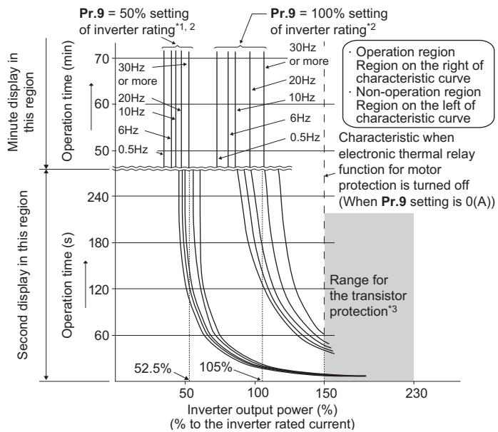
\*1 When setting **Pr.9** to a value (current value) of 50% of the inverter rated output current.
