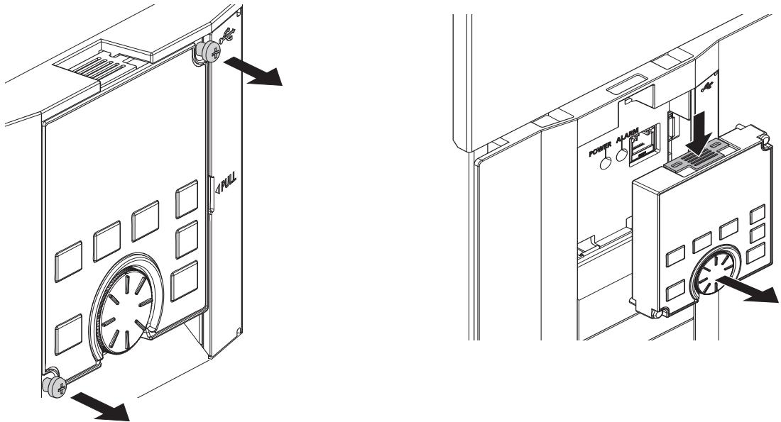
To reinstall the operation panel, align its connector on the back with the PU connector of the inverter, and insert the operation panel. After confirming that the operation panel is fit securely, tighten the screws. (Tightening torque: 0.40 to 0.45 N·m)
