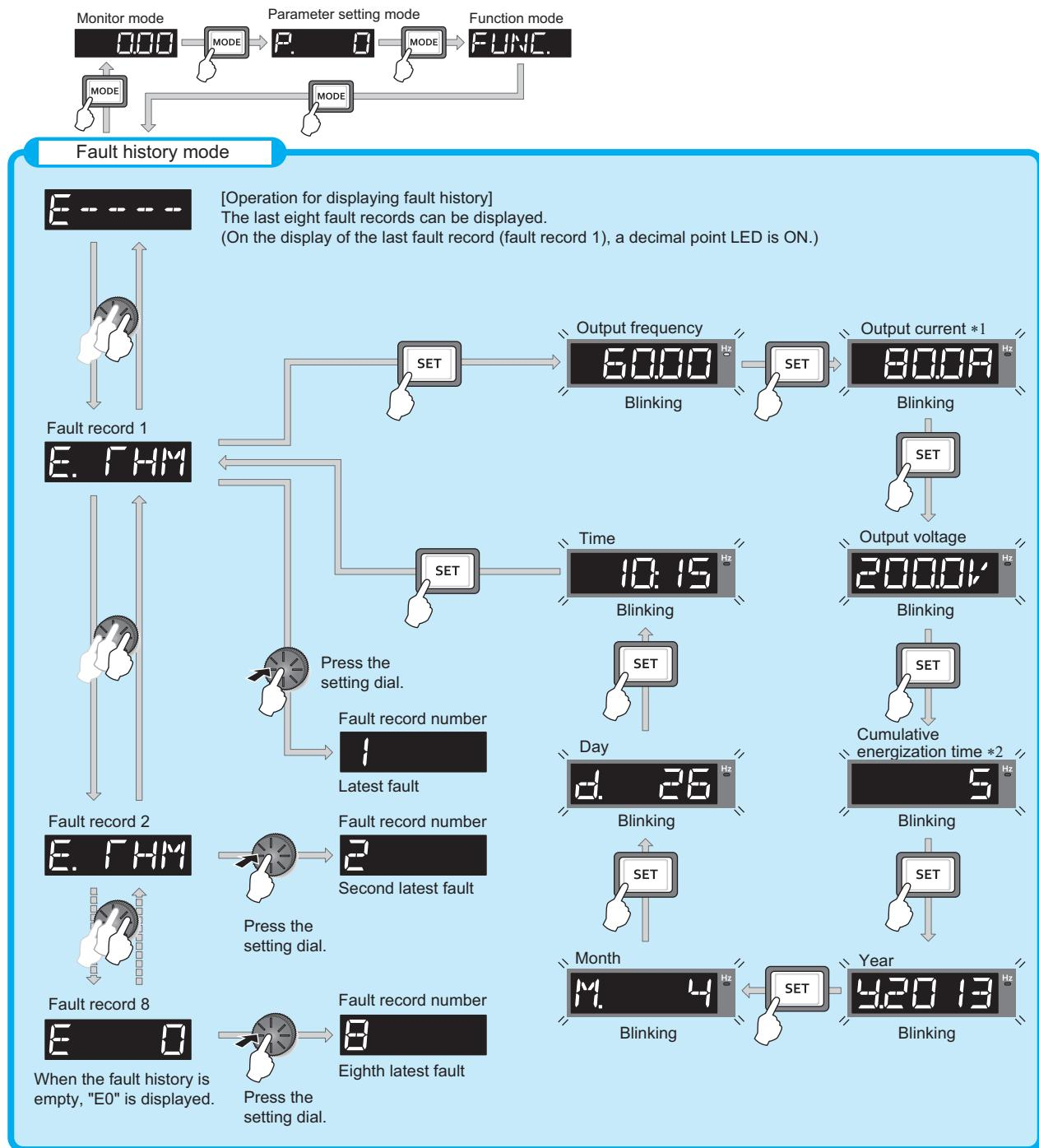
\*1 When an overcurrent trip occurs by an instantaneous overcurrent, the monitored current value saved in the fault history may be lower than the actual current that has flowed.
