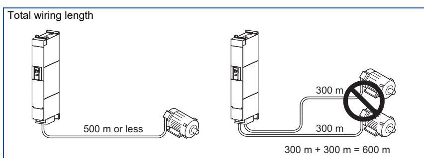
When driving a 690 V class motor by the inverter, surge voltages attributable to the wiring constants may occur at the motor terminals, deteriorating the insulation of the motor. In this case, use a 690 V class inverter-driven insulation-enhanced motor. When the wiring length exceeds 100 m, set "4" (4 kHz) or less in **Pr.72 PWM frequency selection** (carrier frequency).
