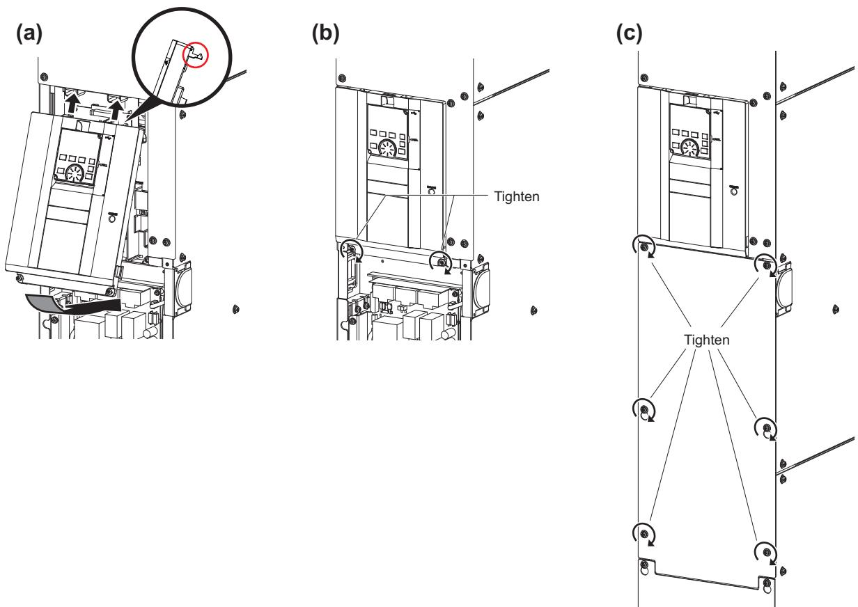
(a) Insert the upper hooks of the upper front cover into the sockets of the inverter.
