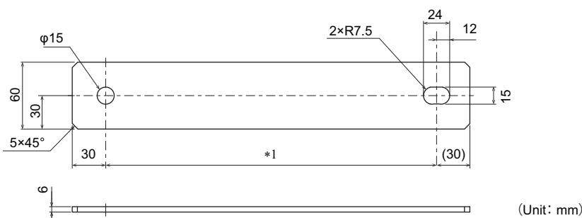
\*1 The bus bar dimensions differ depending on the arrangement of the inverter and the converter unit as shown in the following table.
