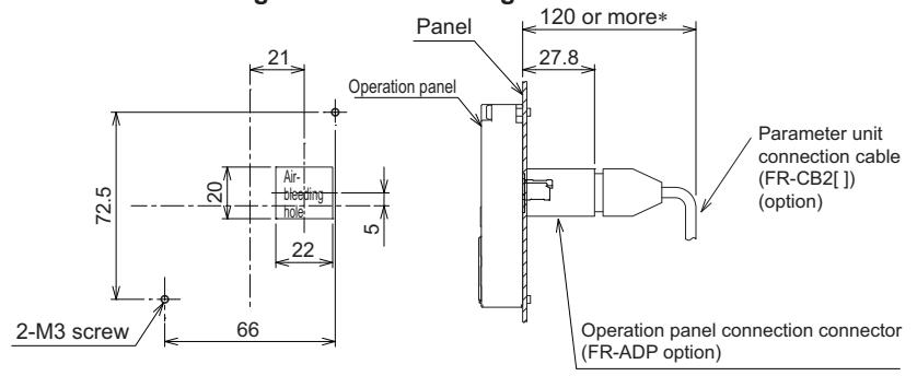
\* Denotes the space required to connect an optional parameter unit connection cable (FR-CB2[ ]). When using another cable, leave the space required for the cable specification.
