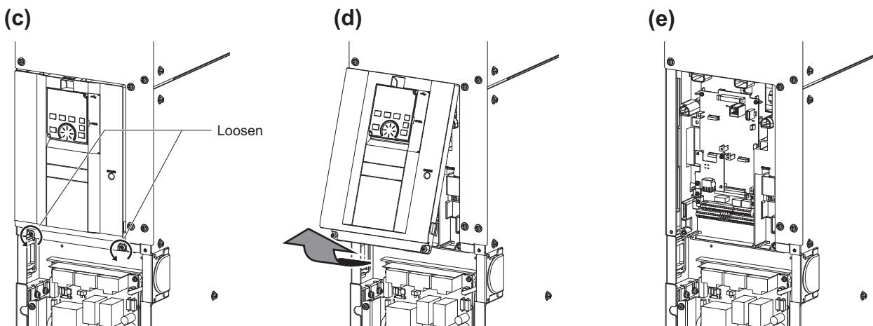
(c) With the lower cover removed, loosen the mounting screws on the upper cover. (These screws cannot be removed.)
