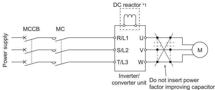
\*1 The converter unit (FR-CC2) has a built-in DC reactor.
