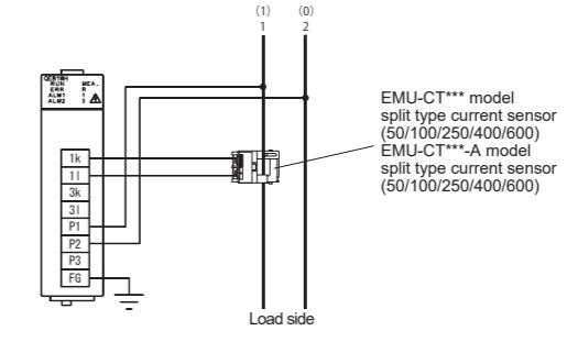
• Input signal wire shall not be bound together with or placed close to the main circuit and power line. Keep 300 mm or longer distance between them.
