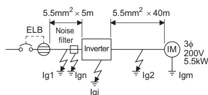
Note: 1. Install the earth leakage current breaker (ELB) on the input side of the inverter.
