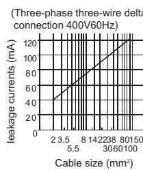
For "Y" connection, the amount of leakage current is approx. 1/3 of the above value.
