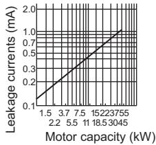
Example of leakage current per 1km during the commercial power supply operation when the CV cable is routed in metal conduit
