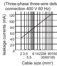
Leakage current example of three-phase induction motor during the commercial power supply operation (Totally-enclosed fan-cooled type motor 400 V 60 Hz)
