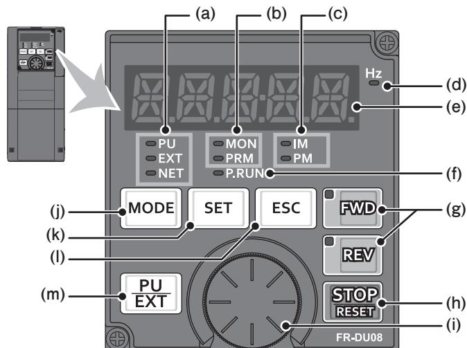
The operation panel of the inverter can be used for the converter unit.
