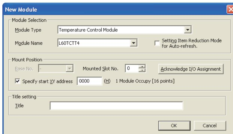
**4. Display the L60TCTT4 Switch Setting window and configure the setting as follows.**
