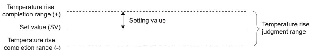
When CH□ Temperature process value (PV) (Un\G9 to Un\G12) enters the temperature rise judgment range, CH□ Temperature rise judgment flag (Un\G17 to Un\G20) is set to Within temperature rise completion range (1). (Set the time from the temperature rise completion to Within temperature rise completion range (1) in Temperature rise completion soak time setting (Un\G168).)
