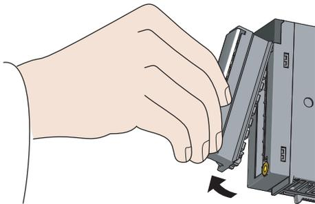
1. Open the terminal cover and loosen the terminal block mounting screw.
