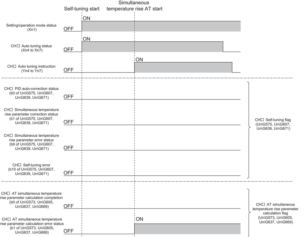
**(b) When the simultaneous temperature rise AT is started after the simultaneous temperature rise parameter is calculated with self-tuning**
