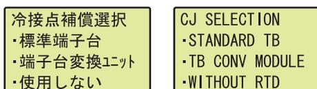
1. Use the ▲ and ▼ buttons to select "STANDARD TB" or "WITHOUT RTD", then make a confirmation with the  button. ("TB CONV MODULE" cannot be used.)
