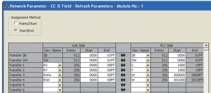
**5. Write the set parameter to the CPU module on the master station. Then reset the CPU module or turn off and on the power supply of the programmable controller.**
