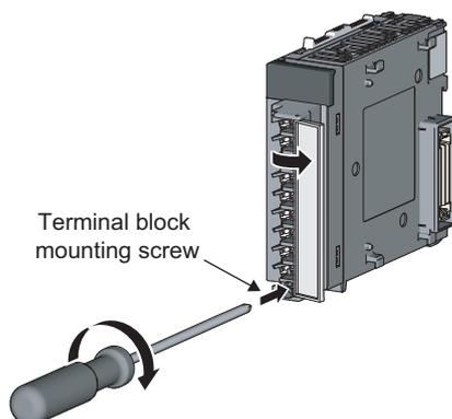
1. Fully insert the projections on the top of the terminal block into the terminal block fixing holes of the module and press the terminal block until it snaps into place.
