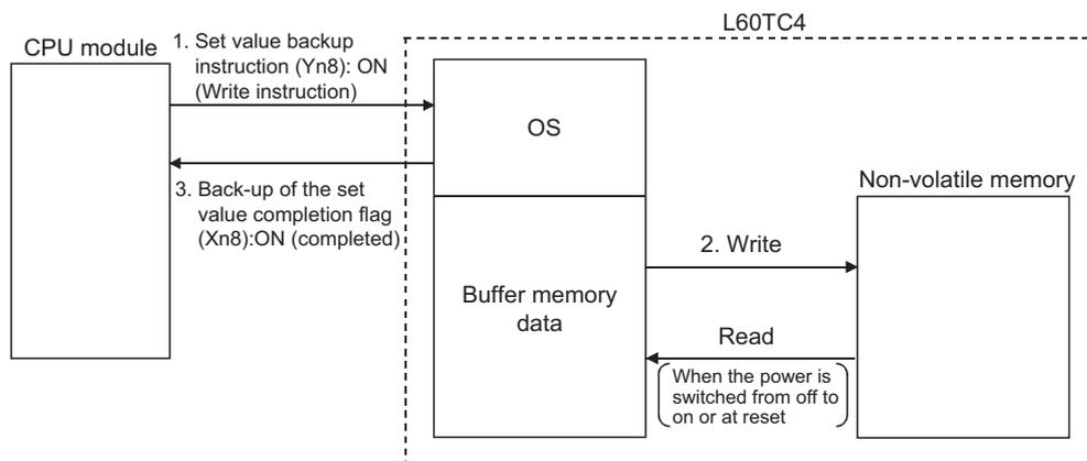
If data write to non-volatile memory does not complete, Back-up of the set value fail flag (XnA) turns on.
