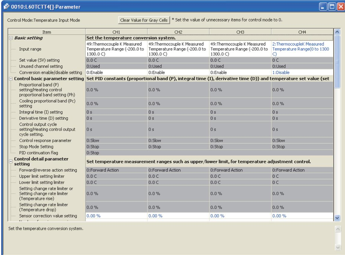
Control Mode:Temperature Input Mode Clear Value for Gray Cells \* Set the value of unnecessary items for control mode to 0.
