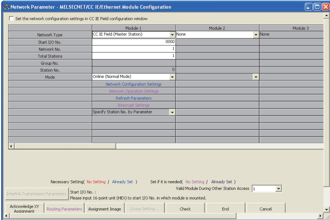
**3. Display the network range assignment setting window and configure the setting as follows.**
