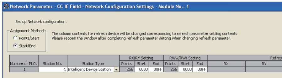
**4. Display the refresh parameter setting window and configure the setting as follows.**
