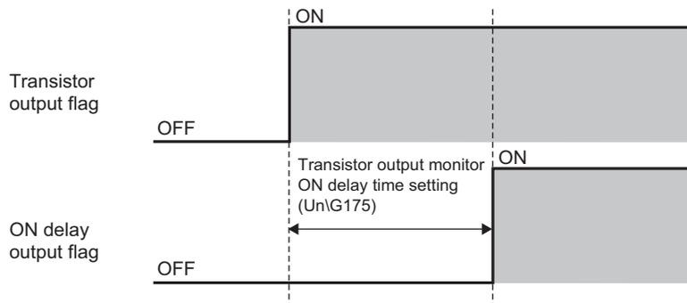
Transistor output monitor ON delay time setting (Un\G175) enables setting considering delay time (response/scan time delay) of actual transistor output. (Page 381, Appendix 2 (45)) By monitoring the ON delay output flag and external output on the program, disconnection of external output can be judged. For details on the ON delay output function, refer to the following.
