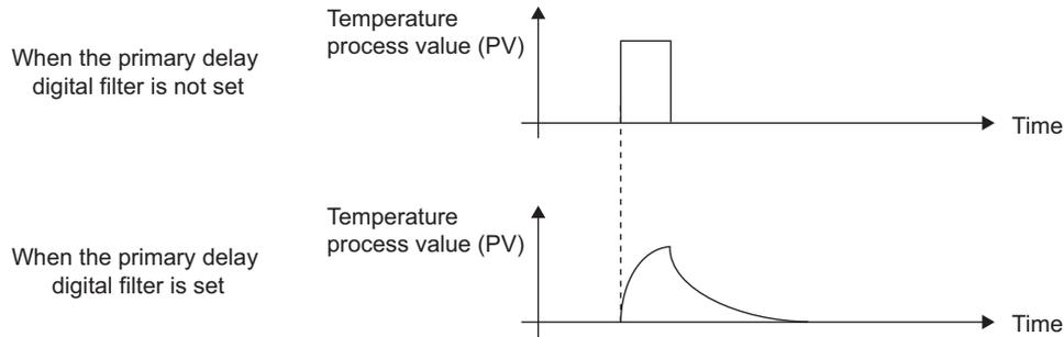
For the primary delay digital filter, set the time until the temperature process value (PV) changes by 63.3% (time constant).
