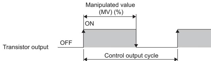
The ON time of the control output cycle is determined by multiplying the control output cycle by the manipulated value (MV)\*1 (%). If the manipulated value (MV)\*1 is constant, a pulse of the same cycle is output repeatedly.
