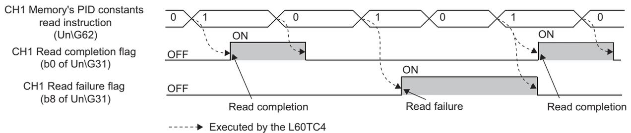
When the data reading from the non-volatile memory is completed normally, CH□ Read completion flag (b0 to b3 of Un\G31) of the corresponding channel turns on.
