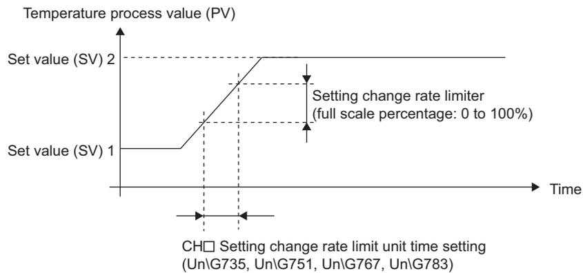
**(a) Batch/individual setting of temperature rise and temperature drop**
