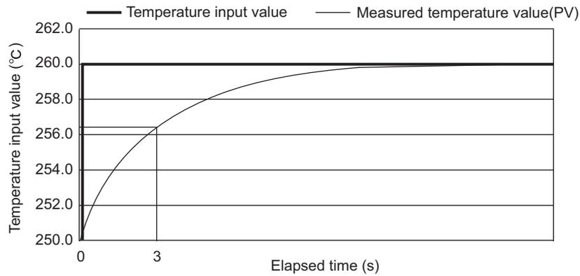
The temperature reaches 256.3°C which is 63.3% of the temperature process value (PV) three seconds after the temperature input value has reached 250.0°C.
