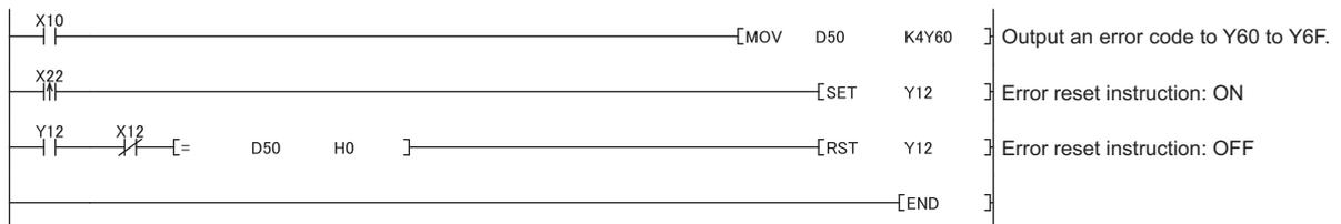
**(7) Program example of when not using the parameter of an intelligent function module**
