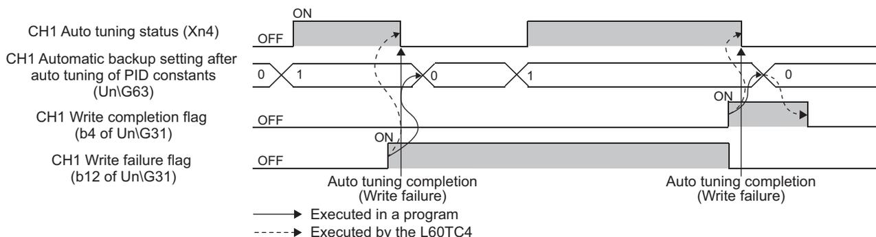
When the data writing to the non-volatile memory is completed normally, CH□ Write completion flag (b4 to b7 of Un\G31) turns on.
