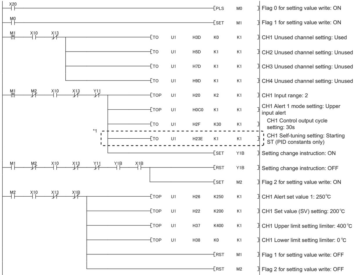
\*1 Configure this setting only when the self-tuning function is used.
