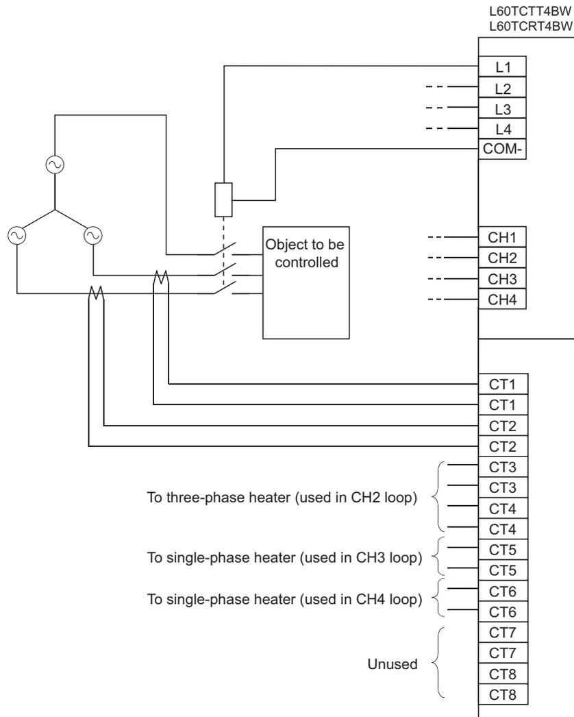
Three-phase heater disconnection detection is executed by measuring the currents of two of the three cables. In the above wiring example, set CT□ CT input channel assignment setting (Un\G264 to Un\G271) as indicated below.
