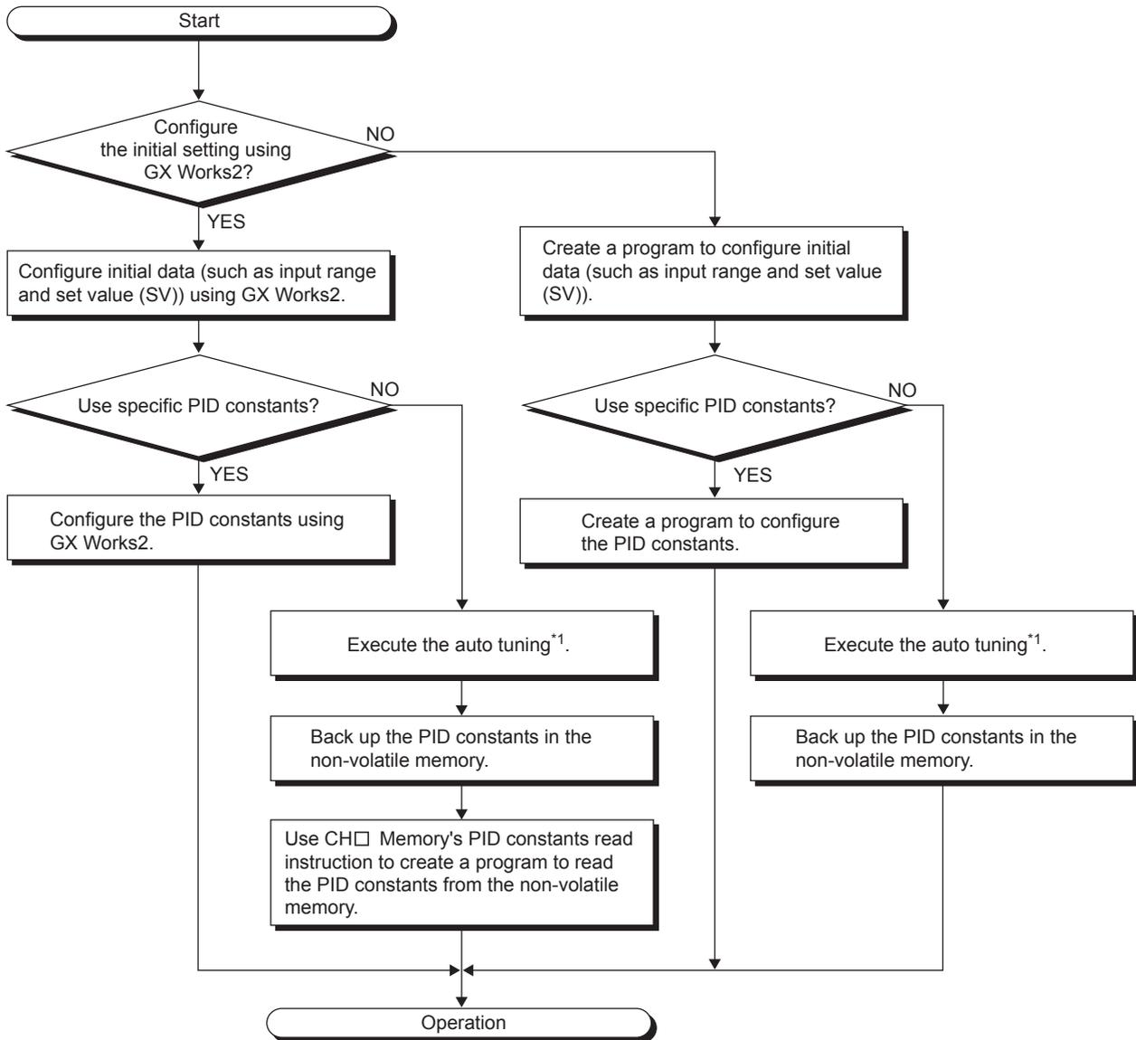
\*1 In the standard control, the self-tuning can be selected if necessary.
