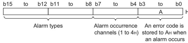
If the lower four bits are "0001" (1H) to "1001" (9H) or "1011" (BH) to "1111" (FH), an error occurs. When an error occurs, refer to the error code list (Page 316, Section 11.6).
