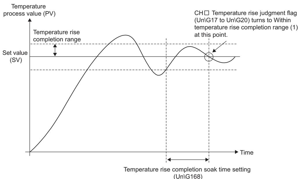
Set the temperature rise completion range and temperature rise completion soak time in the following buffer memory areas.
