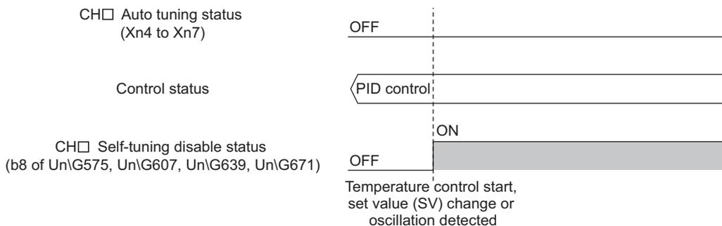
**(c) When the simultaneous temperature rise parameter cannot be calculated**
