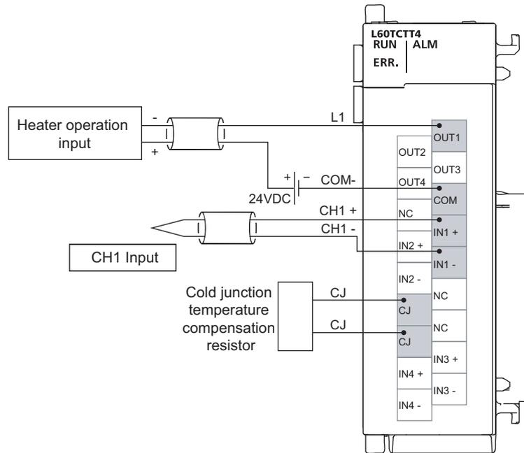
10.2 When Using the Module in a Standard System Configuration
