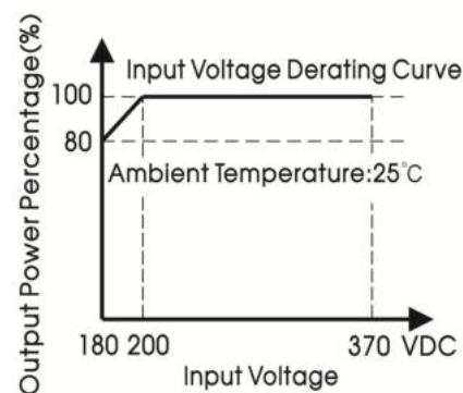
Note: 1. With an AC input voltage between 180-200VDC the output power must be derated as per the temperature derating curves;
